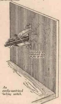
Safety Device for Meter Controls
