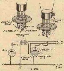
Fig. 4.—This shows the simplest connections for a pentode, as well as the corresponding connections for five-pin and base terminal valves.
