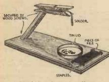
A handy device for use when soldering.
