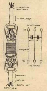
Diagram showing the method of construction employed in the Belling-Lee 3-core suppressor, and the electrical circuit.
