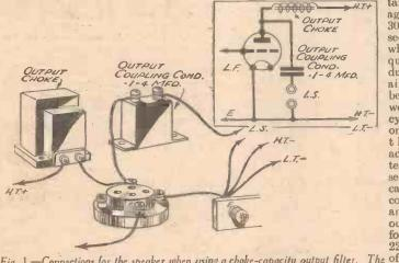
Fig. 1.—Connections for the speaker when using a choke-capacity output filter. The of the factors inductance of the choke must be found by calculation, using the optimum load of the in the above equation are known with valve.
