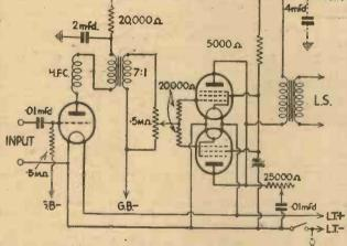
1.- A Push-pull stage will avoid overloading Fig. difficulties, following an efficient L.F. stage.
