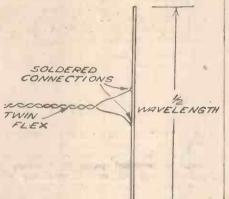
Fig. 2.—Here a single length of rod or wire is used for the aerial, and the feeder ends ore joined at a distance of about 10ins. in the centre.
