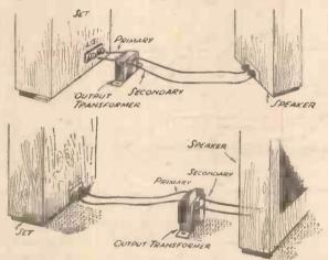
Fig. 1.-When using the arrangement shown in the upper illustration. a loss of signal strength occurs, due to the resistance of the long leads in the transformer secondary circuit. This loss is obviated by using the system shown in the lower illustration.
