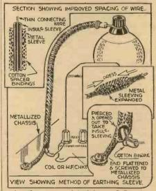
An efficient screened lead for an S.G. value.
