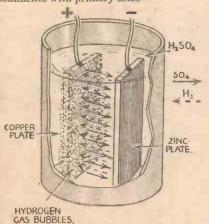
Fig. 1.-The common copper-zinc cell.
