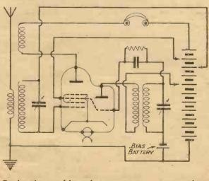
Fig. 1.- A suggested form of super-regenerative receiver employing a triode-hexode valve.
