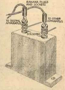
A method of making connections quickly for test purposes.
