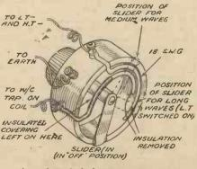
An easily-made dual-purpose rotary switch.
