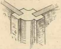
Fig. 2.—An easy to assemble corner which avoids difficult joints.
