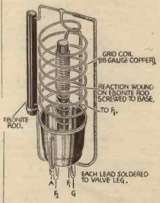
A method of constructing efficient short-wave coils.
