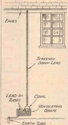
A convenient arrangement, where a screened downlead is passed from the inside aerial beneath the eaves to a lead-in tube in the ventilating grate. An insulated lead is taken from there through the floorboards and to the set.
