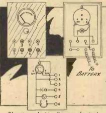
Plan view and wiring diagrams of a simple mulli-purpose testing unit.
