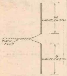
Fig. 4.—In this scheme the aerial is split into two separate quarter-wavelength sections.
