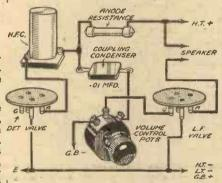
Fig. 3.—L.F. volume control in an R.C.C. or choke-capacity coupled amplifier. The potentiometer volume control replaces the grid leak and should be of similar value.
