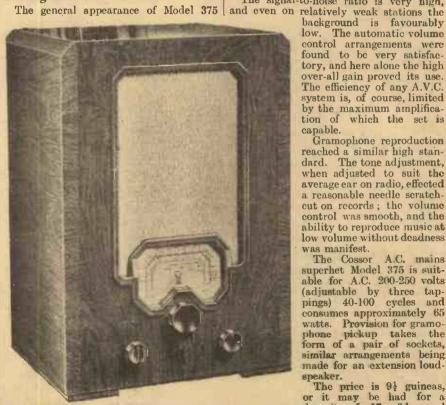
station names and is illuminated, the deep coffee colour preventing the glare that is so In addition to the simple controls on the front, there is a tone control at the rear intended to be treated as a preset adjustment.
