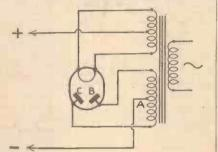
Fig. 1.—Any disconnection or poor contact between A and B or A and C will produce hum as the mains unit will be working as a half wave rectifier. Test voltages between A and B and A and C with an A.C. voltmeter. Readings should be the same.
