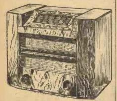
This is the Philips receiver in which the dial is hinged, and may be set at various angles without affecting the indicating mechanism.
