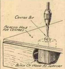
Fig. 2.—After making small centre holes from the inside of the cabinet full size holes should be traced out on the front, using a centre bit.
