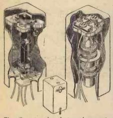
These illustrations show the internal construction of the Raymart variable selectivity I.F. kit components.
