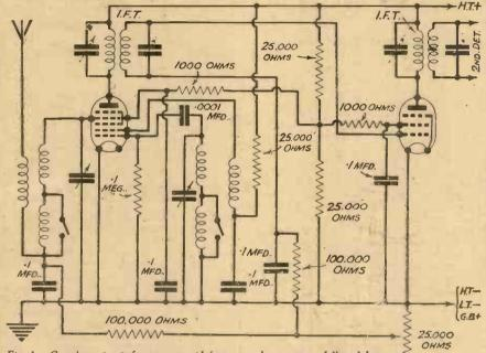
Fig. 1.—Complete circuit for a pentagrid frequency-changer stage followed by an H.F. pentode I.F. amplifier. Values of components are shown, but these may have to be modified for certain makes of valves.
