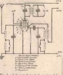
Fig. 5.—A theoretical circuit of a pentagrid frequency changer, showing the arrangement of the value electrodes. knob tuning can be obtained in conjunction, with a gang condenser.
