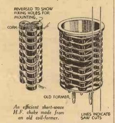
their junk box. It will be seen from the sketch that three portions are cut from the old coil former by means of a hacksaw, and then placed together. A small cork placed in the middle will assist in holding the parts together while the choke is wound. The together while the choke is wound. winding of the choke consists of 120 turns wound in eight sections of fifteen turns each. The wire can be anchored at each end in the usual way.—Lewis Jones (Holyhead).
