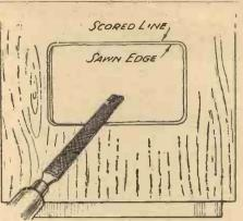
Fig. 4.—How the opening in the cabinet is finished off. The file is inclined.
