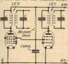
Fig. 5.- A simplified method of feeding the screening grids of the frequency-changer and I.F. valves. This is not as good, theoretically, as the method shown in Fig. 1, but can often be used successfully.
