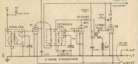
Fig. 1.- A simple but efficient circuit using the BP. 114 coil combination.
