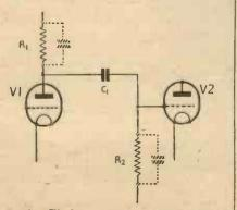
Fig. 1.-The basic resistance-capacity circuit.
