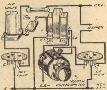
Fig. 2.—Connections for an L.F. volume control when using transformer or resistance-fedtransformer coupling.
