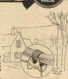
A method of suspending an aerial to allow for automatic adjustment.
