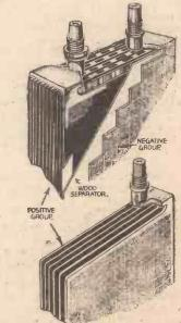
Fig. 7.-Showing the construction of the Faure cell.
