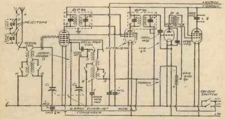
Fig. 3.-In this battery circuit the BP. 112 coil combination is employed.
