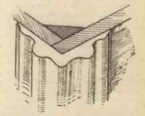
Fig. 4.— This type of corner moulding will cover up faulty workmanship.
