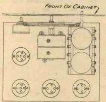
Fig. 3.—The set can be used as its own template by first making a hole for the longest spindle, and then marking the positions of the others, and drilling the holes in turn.
