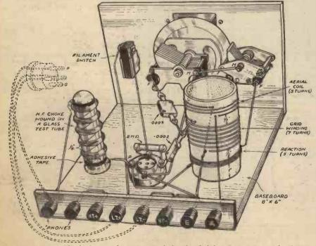
Here is an example of a home-made receiver in which coil and choke are also constructed at hom
