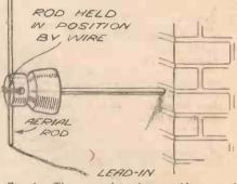
Fig. 6.—This type of insulator enables a rigid acrial to be erected on the side of the house.
