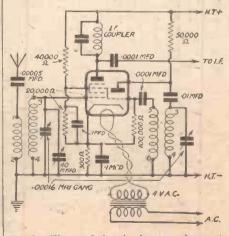
Fig. 3.—The triode-hexode frequency-changer is a more efficient arrangement, but requires some experiment to find the most suitable working voltages.
