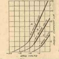
Fig. 1.—Anode<sup>2</sup>-current-grid-volts characteristic curves for a typical small power valve. Straight portions of the "curve" are shown heavier to simplify reference.
