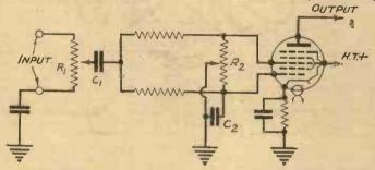
known as a programme expander. The ar-rangement is shown diagrammatically in Fig. 4 overleaf
