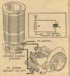
Fig. 2.—This is the method of building up an ácrial tuner as described in this article.
