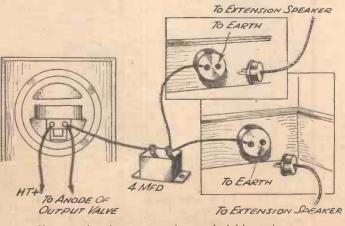
How a number of extension speakers can be fed by single wires.
