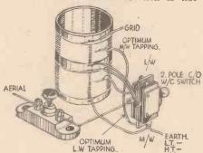
Fig. 5.—Connections for a wave-change switch.
