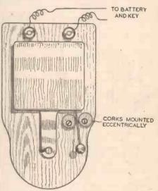
A high-note buzzer made from an old bell.
