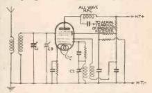
Fig. 3.—A mains-operated S.W. superhet converter using heptode frequency changer. Cl and C2 are ganged, and C3 is a variable trimmer.
