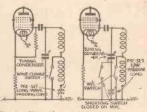
Fig. 2.—These circuits show alternative connections for the long-wave padding condenser.
