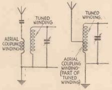
Figs. 1 and 2 (left and right).—These circuits show the similarity between a loose-coupled and tapped aerial coil.
