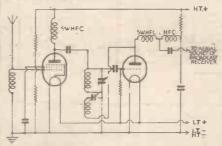
Fig. 2.—A superhet S.W. converter using simple autodyne circuit with an untuned H.F. amplifier to reduce re-radiation.
