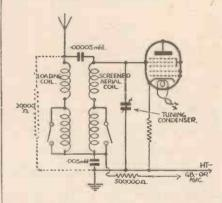
Fig. 6.—Showing the connections for an "image filter" suitable for use in conjunction with a single-circuit aerial tuner of a 465 kcls superhet.
