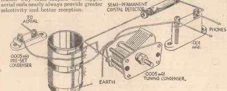
Fig. 4.—This shows the method of using the coil in a modern crystal-set circuit.
