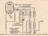
Fig. 1.—This skeleton circuit shows the complicated system of condensers required in the oscillator circuit when using certain types of coil in a 465 kc/s circuit.
