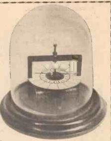
The finished galvanometer.
