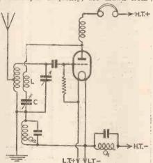
Fig. 5.—The basic circuit of a superregenerative receiver.
