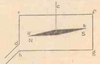
Fig. 4.—A magnetic needle suspended in a single coil of wire.
