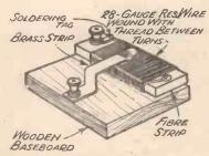
Fig. 4.—This illustration shows the construc-tional details of the 10 ohm variable resistance described.
