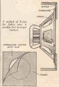
then cut a hole in the centre the same size as the diameter of the speaker cone. On the cardboard glue the fabric with the pattern arranged as desired. Place the cardboard with the fabric side against the back of the baffle, and then screw the speaker in place. This idea enables the fabric to be fixed behind the fret without wrinkles or creases-G. A. WREN (Deptford).
