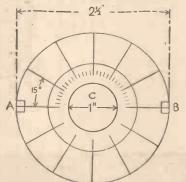
Fig. 9 .- How to mark out the scale.
