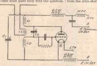
Fig. 1.—The circuit for a suitable ultra-short-wave converter.
