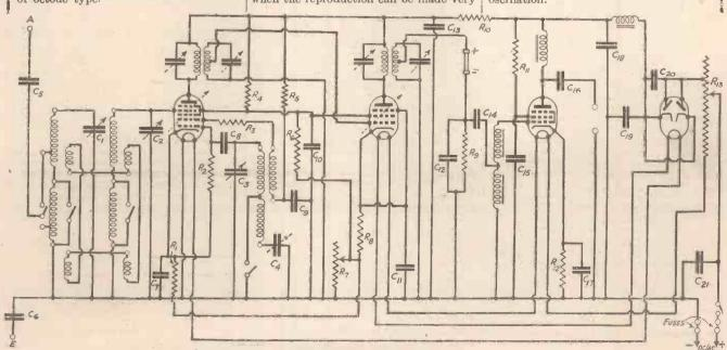
Fig. 4.—Theoretical circuit of the Universal Three-valve Superhet.
