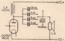
Fig. 3 .- Varying the tone by means of a condenser circuit.
