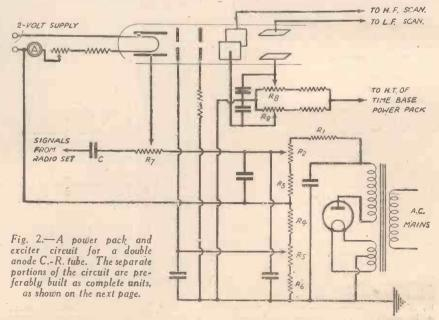
fixed condenser C, which of course serves to isolate the cathode-ray tube proper from the radio set.
