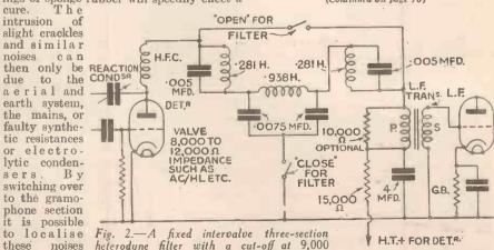
Fig. 2.—A fixed intervalve three-section heterodyne filter with a cut-off at 9,000 H.T.+ FORDET. cycles. The two switches can be linked together to operate as denoted, so that for transmissions free of sideband interference the full frequency response of the set may be utilised.
