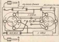
Fig. 4.—Wiring plan using the flat construction. This may, of course, be modified to suit the particular construction which is adopted.
