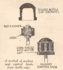
passed through the centre of the cork, which is clamped between nuts and washers as shown. The cork is pushed into the cap to the necessary depth, and, by tightening the outside nut, the cork can be made a tight fit in the cap.—B. KING (Cardiff).
