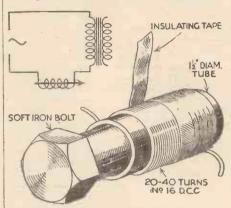
An easily-made voltage regulator for A.C. mains.
