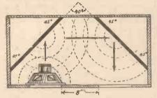
An idea for a single-unit stereophonic loudspeaker
