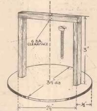
Fig. 8.—The galvanometer bridge and base.
