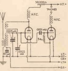
2.- A detector circuit in which an additional valve (the first) is used for reaction control.
