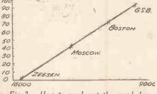
Fig. 3.—How to mark out the graph for calibrating the meter.
