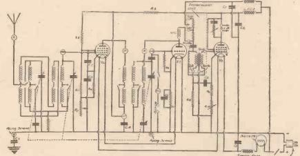
Fig. 1.—The circuit of a typical receiver where the band-pass filter precedes the first valve.
