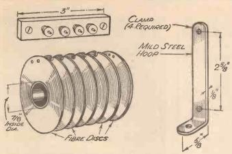
Fig. 3.—Details of the winding spool.
