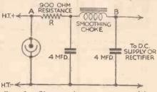
Fig. 5.—Showing how a neon stabiliser should be connected. Note the extra resistance used to bring the total value between the rectifier and H.T.+ lead up to 1,800 ohms.
