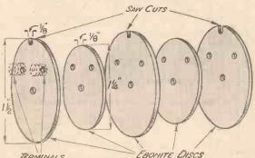
Fig. 2.—Constructional details of the high-frequency choke.
