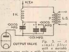
with a variable response over quite a wide frequency range. The tuning condenser can be of the bakelite dielectric type, the other condensers being of fixed capacities. For commercial receivers the components can be mounted in a small box and then connected across the primary of the transformer fitted to the loudspeaker, as shown. It is also possible to join the filter as shown. It is also possible to join the filter across the primary of an L.F. transformer.
