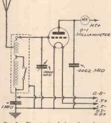
Fig. 3.—The circuit of the valve voltmeter described.
