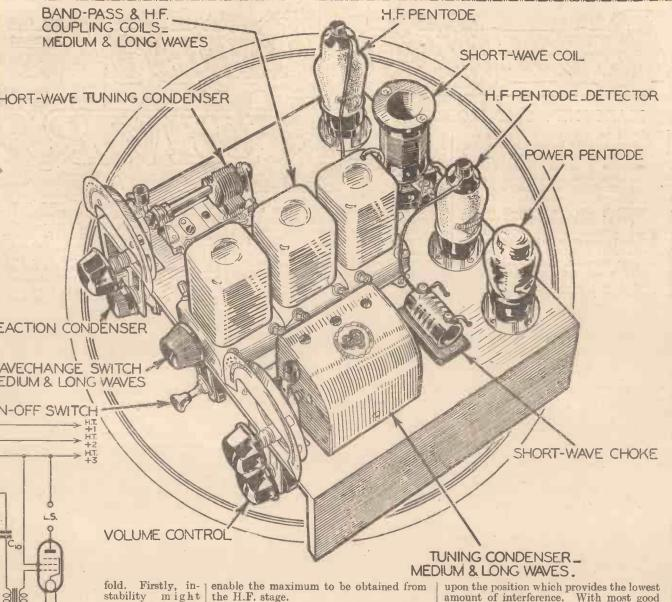
fold. Firstly, instability might arise due to the necessity for decoupling the anode circuits, and secondly, hum might be experienced when the receiver is tuned to the short waves. The first-mentioned trouble is overcome in the usual way by O→C.B+ the use of decoup->LT+ ling resistances and condensers, and in general it should
