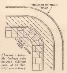
bility of the return current leaking, via earth, to another part of the circuit and causing the voltage drop which he measured. There is also a possibility of leakage from some large electrical apparatus nearby.-ROBERT BARLOW (Prestwick).
