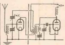
Fig. 4.—A modification of Fig. 3—using a tapped H.F. transformer.
