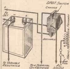
Fig. 6.—The switching system required when using an A.C. trickle charger.
