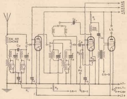
Three valves, all-wave, separate short-wave components and all-pentode circuit, are the main features of this interesting receiver.
