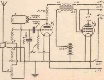
Fig. 4.-Circuit diagram of the Guinea Two-Valver
