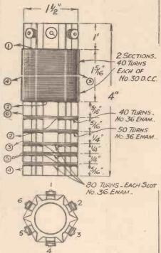
Fig. 1.—Details of the tuning coil.
