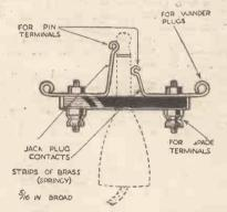
A neat jack plug switching arrangement for alternative speakers.
