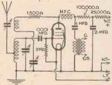
Fig. 2.—An H.F. pentode as detector.
