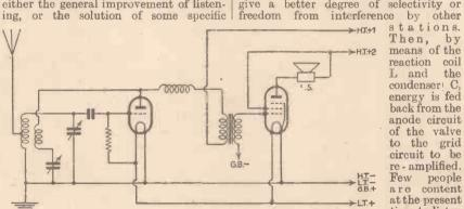
Fig. 2.—Adding a stage of L.F. amplification to the circuit shown in Fig. 1 to increase signal output.
