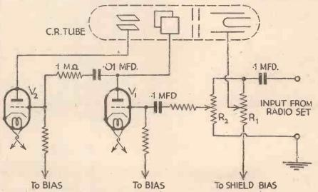
that, provided the set employed is a good | Fig. 1.—One arrangement for linking the signals from the radio receiver to the C.-R. tube.
