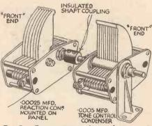
Fig. 7.—Ganging two condensers for use in the circuit given in the first column.
