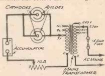
Fig. 3.—The circuit for the A.C. charger described, and which uses two chemical rectifiers wired in parallel.
