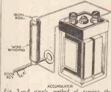
Fig. 3.—A simple method of proving the creation of electro-magnetism.
