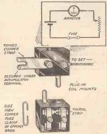
A plug-in fuse using a strip of tinfoil.
