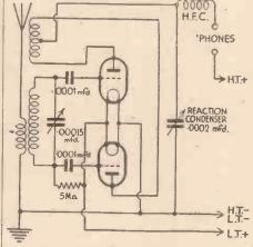
Fig. 1 .- The push-pull detector circuit described.
