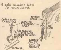
fail, and costs next to nothing. The dodge is a boon to anyone wanting a simple remote control for a receiver, and not wanting to interfere with the wiring of their sets, and not wishing to run live wires about the house.—A. E. Ball (Morden).
