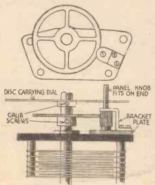
A slow-motion drive made with old gramophone motor gear wheels.
