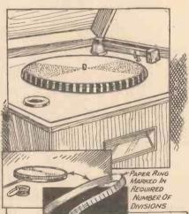
THE EDGE OF A GRAMOPHONE TURNTABLE IF DIVIDED IN ALTERNATE BLACK & WHITE SECTIONS, AS SHOWN ABOVE, FORMS A PERMANENT STROBOSCOPE FOR 40 CYCLES\_120 DIVISIONS: FOR 60 CYCLES. 184 DIV.: FOR 25,508 100 CYCLES. 152 DIV.
