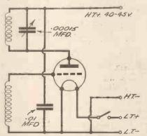
Fig. 2.—An alternative tuned-anode circuit.
