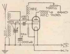
Fig. 3.—A modified arrangement of the circuit shown in Fig. 2, but using an S.G. valve for detection and reaction control.
