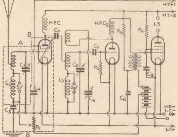
Fig. 1.—The complete three-valve circuit considered in this series of articles, the components described this week being enclosed in the box marked B.
