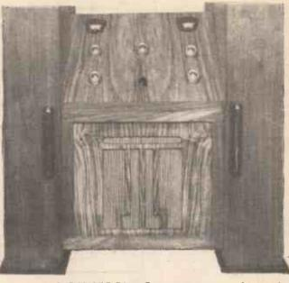
Here is F. J. CAMM'S Silver Souvenir in its new and original cabinet. The panel is inclined for ease of operation. Chromium-plated knobs are used. The two lockers provide accommodation for phones, testing equipment, batteries, books, etc.
