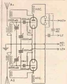
Fig. 4.—A double detector circuit which is suggested for experimental purposes. Both detectors are individually tuned and have their own aerials.
