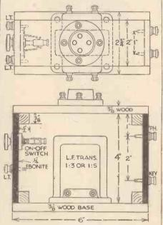
Figs. 1 and 2.—Plan and elevation of a morse code practice unit for giving noiseless signals.
