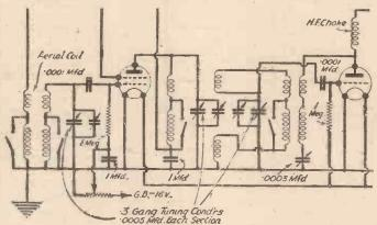
Fig. 2.—In this diagram the band-pass tuning circuit is shown between the first two valves. The advantages of this arrangement are explained on this page.
