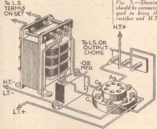
Fig. 3.—A practical wiring plan of the amplifier. The arrangement is the same as that shown in the theoretical in Fig. 1.
