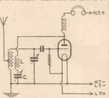
Fig. 1.—A simple one-valve detector circuit with reaction to illustrate the principles.
