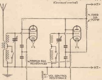
network before the Fig. 3.—A system of variable-mu volume control frequently used in 2 H.F. first valve, as shown or superhet. mains receivers. It often proves inferior to the circuit arrange-in Fig. 1, especially, ment shown in Fig. 4. Component values are not shown, since they depend entirely upon the particular valves employed.
