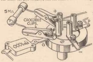
Fig. 1.—A simple scheme for adjusting the detector circuit.
