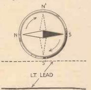
Fig. 1.—Showing how an electric current has a directive effect on a magnetic needle.
