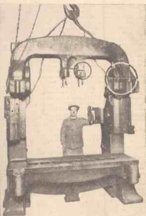
This illustration shows the cracks in a powerful press which were repaired by the low-temperature welding process described in this article.
