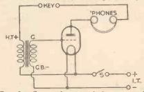
Fig. 3.—Circuit diagram of the morse code practice unit.
