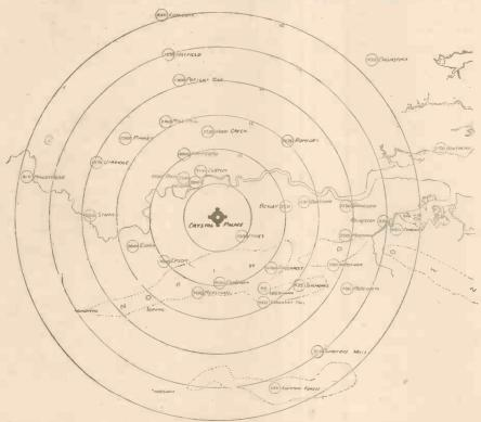
Fig. 2.—Chart indicating field strength data in microvolts from the Baird transmitter at the Crystal Palace.
