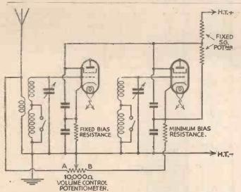
Fig. 4.—Another system of volume control which has many important advantages.
