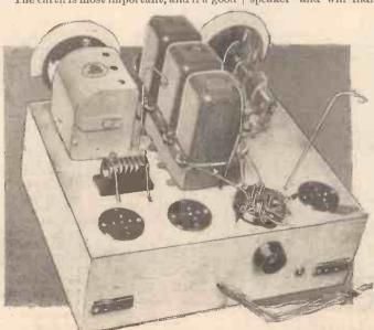
This rear view shows the short-wave change-over switch, An underneath view of the Silver Souvenir.
