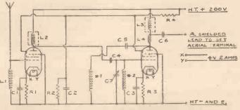
The new Mervyn 3-range short-wave coil unit, and a theoretical circuit of a short-wave converter incorporating the unit.
