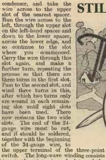
of twenty-three turns in each slot, and the finish of the winding is joined to the lower terminal of the left-hand tuning condenser.
