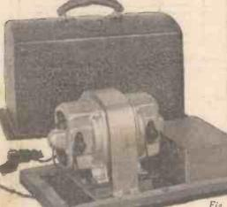
Fig. 5.-Recourse must be made to machinery rotating in order to "step-up" the vollage of a D.C. supply.
