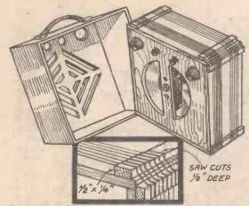
Fig. 4.—Details of the frame and case of the portable receiver described in the text.
