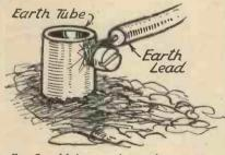
Fig. 7.- Make sure the earth connection is sound.
