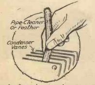
Fig. 8.- Dust in between condenser vanes gives rise to grating noises when taning.
