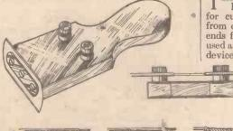
A handy tool for removing the insulation from connecting wire.
