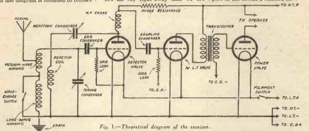
you what the set looks like in its assembled form and to show the disposition of the various parts, otherwise it does not help much towards understanding how it works. Figs. 1 and 2 are provided for that purpose, as they show clearly all the
