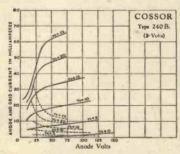
Anode and Grid Current/ Anode volts curves of Cossor Class "B" Valve Type 240 B.
