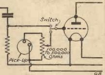
Fig. 13-Control of input from pick-up by a potentiometer.
