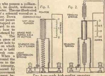
Two home-made high-reading ammeters.
