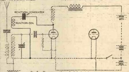
Fig. 7.—Here we see the path of the high-frequency currents which provide reaction.
