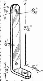
Fig. 4.—Dimensions of transformer core clamps -four are required.
