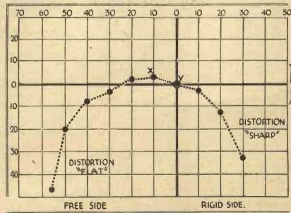
Fig. 3.—Chart showing results of tests with the semi-rigid type of diaphragm.
