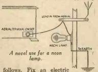
follows. Fix an electric lamp holder beside the aerial lead-in tube and connect up as illustrated. One terminal of the holder is joined to the aerial and the other is earthed. Insert a standard 240–260-volt neon lamp into the holder; most electrical dealers can supply these for about 3s. each. When a thunderstorm
