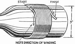
Fig. 4.—Winding the coil round a bottle.
