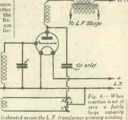
former would be to reduce the high note response, while if the capacity were decreased the high note response would be correspondingly increased. A varying capacity shunt is provided by the use of a differential reaction condenser of somewhat special design, and connected in a manner which differs slightly from the normal.
