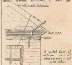
the accompanying sketch. The mast was a short piece of old conduit, as used by electricians for wiring purposes. It is very rigid when erected, if a short length is used. One end was flattened and driven into the bricks by long nails.
