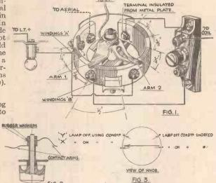
A multi-control switch made from an old rheostat.
