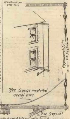
Fig. 2 .- A vertical aerial held well away from the wall approximately 20 ft. high, will give very good results.
