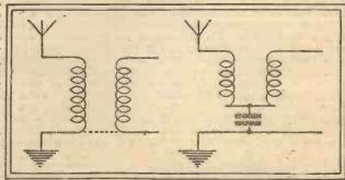
Fig. 6 .- Diagrams showing inductive coupling (left) and capacifative coupling (right).
