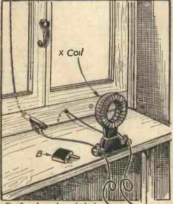
Fig. 2.—A simple method of terminating the aerial and earth leads.
