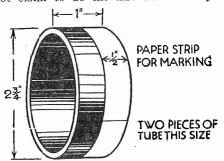
Fig. 3.-Marking the end pieces for the coil.
