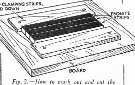
Fig. 2.—How to mark out and cut the coil supports.
