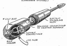
Fitting an indicator to an electric soldering iron.
