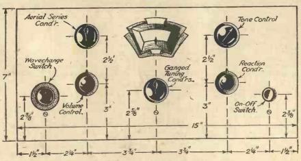
Fig. 2.—Panel-drilling dimensions.
