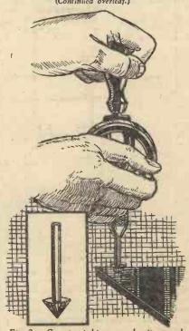
Fig: 2.—Countersinking an ebonite panel.
