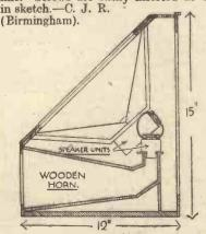
Fig. 2.—Sectional view of speaker.
