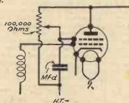
Fig. 5-Variation of screen voltage mains connections.
