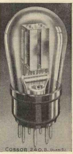
Filament volts 2.0; amps. 0.4; Anode volts 150 max.; Max. Anode Current Swing 50 mA.; Max. Peak Applied Signal (Grid to Grid) 40 volts; Static Anode Current at Va=100, Vg=0 (each half) 1.5 mA.
