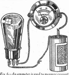
Fig. 6—An ammeter is used to measure current. The illustration shows a valve under test.
