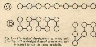
axes at right angles one to the other, and don't have them closer together than is necessary. This will generally obviate serious interaction. Fig. 5 shows a suitable arrangement.
