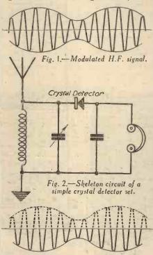
Fig. 3.—The result of half-wave rectification—the "negative" half-cycles have been suppressed.
