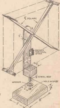
Fig. 1.—Constructional details for a square frame aerial.
