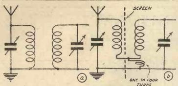
Fig. 4.—Two methods of inductively coupling two circuits.
