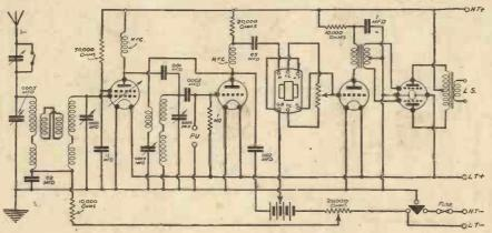
Fig. 1.—Circuit diagram of the Beta Universal Four.
