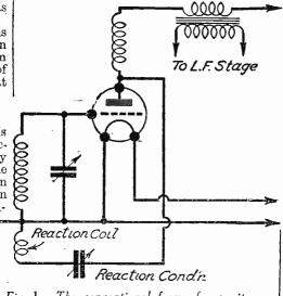
Fig. 1.—The conventional form of capacity reaction control.
