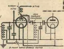
Fig. 2.—Circuit showing how to add an S.G. valve.
