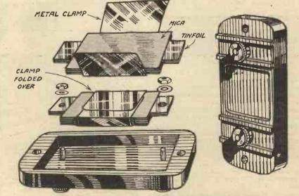
Fig. 2.—Three stages in the construction of a mica condenser.
