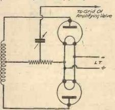
Fig. 5 .- Push-pull diode detection. Instead of two diodes two triodes may be used, their grids being employed as the diode anodes and their anodes lest disconnected.
