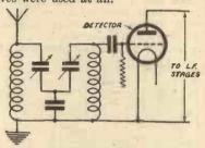
Fig. 2.—One way to employ two tuned circuits is to place them both before the detector.
