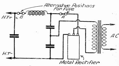
Fig. 9.—Fitting a fuse in a mains unit.
