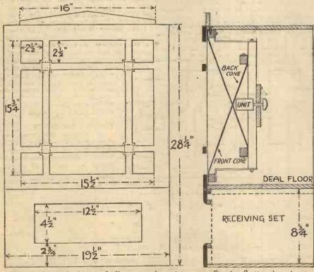
Fig. 2.- Front of cabinet with all necessary dimensions for making up.
