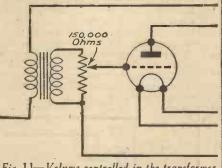
Fig. 11-Volume controlled in the transformer coupled stage by a potentiometer.
