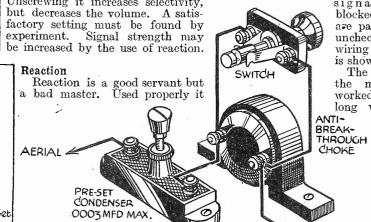
Fig. 2.—An arrangement for preventing the medium wave station breaking through on long waves.
