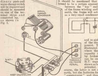
Fig. 6.—The method of connecting a centre-tapped frame aerial to eliminate electrical interference.
