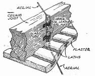
Method of taking a down lead through a
