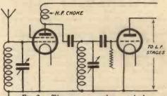
Fig. 3.—The more popular method is to employ a stage of H.F. amplification and to use the second circuit as the coupling between the S.G. valve and the detector.
