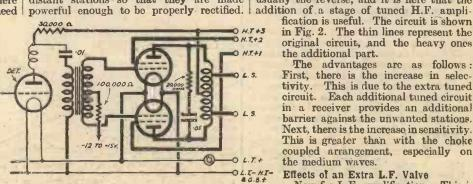
Fig. 5.—Circuit for pentodes in push-pull.
