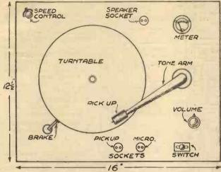
Fig. 1.—The lay-out of the motor-board.
