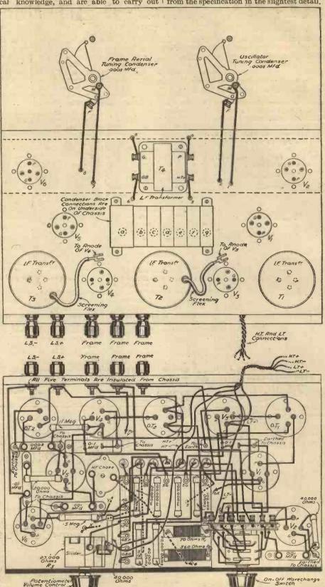
Above- and sub-baseboard wiring diagrams of the Supersonic Six.
