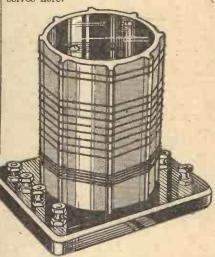
Fig. 4.—Shows three windings on the same former. The coupling here is fairly tight.
