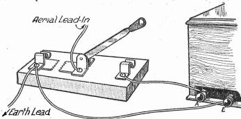
Fig. 4.—A single-pole aerial-earth switch fitted with a spark gap.
