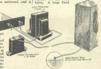
Fig. 2.—The best method of connecting a loud-speaker when it is to be used at a distance from the set.
