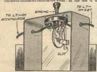
Fig. 1.—A simple coin-operated radio switch showing how a penny completes the circuit.
