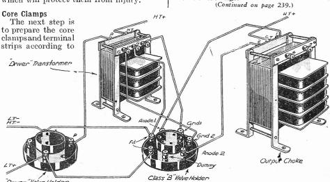
Fig. 8.—This sketch shows how the home-made components are connected up.
