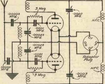
Fig. 2.—The theoretical circuit of the two-detector receiver.
