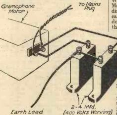
Fig. 1.—A simple method of curing interference caused by an electric motor or similar device.
