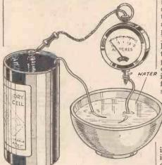
Fig. 2.—This experiment demonstrates that water is a poor conductor.
