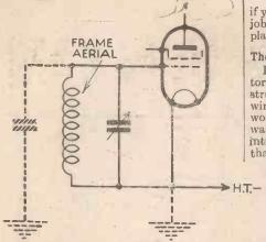
Fig. 4.—This diagram illustrates the effect of stray capacities when using a "plain" frame (the aerial is shown as a coil to simplify the illustration).
