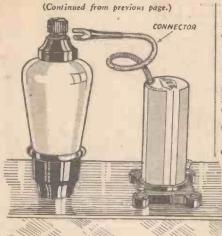
Fig. 4.—An H.F. choke fitted with a connector for joining it to a screen-grid valve.
