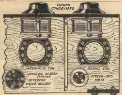
Fig. 7.—How to arrange the lay-out when adding an S.G. valve to a EARTH REEL TECCIVET.
