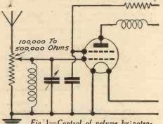
Fig. 1-Control of volume by potentiometer in aerial-earth circuit.
