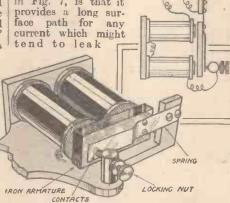
Fig. 6.—A typical contact breaker as fitted to a buzzer.
