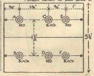
Fig. 2 .- Drilling dimensions for the ebonite top.
