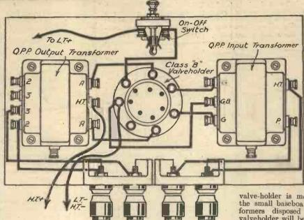
Output Wiring diagram of the Class B Unit
