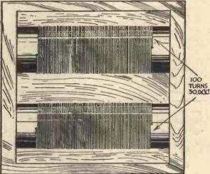
Fig. 3.—How the chokes are made up and mounted.
