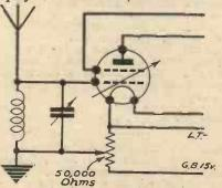
Fig. 6-Control of volume by battery variable mu valve.
