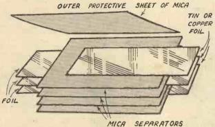
Fig. 1.—How a fixed condenser is built up.
