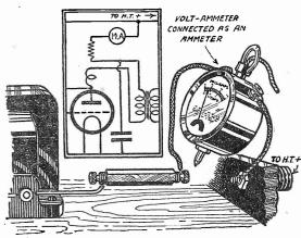
Fig. 4.—Testing the current passing through a resistance in the anode circuit of a valve.
