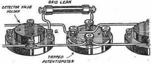
Fig. 5.—Using a tapped potentiometer in the filament leads.
