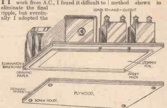
An efficient method of curing mains hum.
