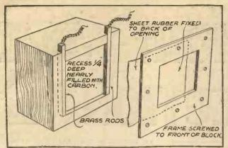
Fig. 10.-A simple carbon microphone.
