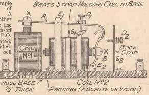
ARMATURES A"&B. DI& D2 ADJUSTING SCREWS. X IRON CYCLE NUTS & BOLTS.
