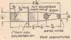
BOLT NUT & BOLT. TO ARMATURE (FREE) +
