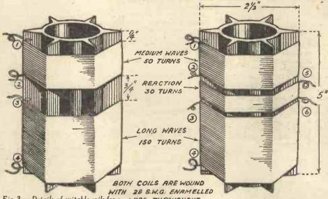
shall be and so on. Fig. 3.—Details of suitable coils for a WIRE THROUGHOUT home-made band-pass tuner.
