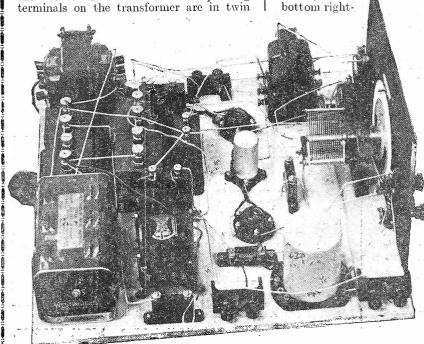
Fig.~4. — This view shows the simple component lay-out. It can be seen that the mains equipment is mounted all together at the back of the baseboard.
