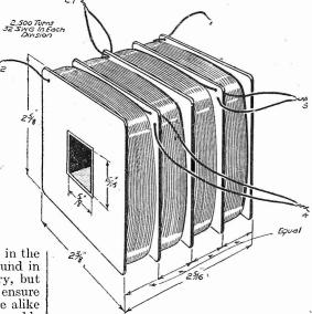
Fig. 7.—Details of spool and windings for output choke.
