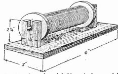
Fig. 3. A simple reel holder which is useful when winding the spools.
