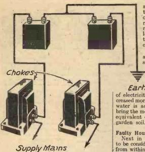
Fig. 5.—To prevent interference from machinery, etc., special chokes may be used as shown here.
