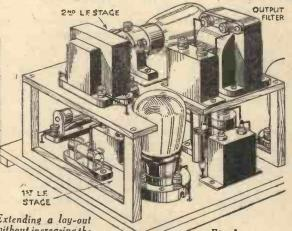
room on the baseboard, but this can easily be overcome by placing the additional components on a raised platform in the manner shown in the accompanying sketch. Valves can be mounted horizontally so that they will not project above the panel. First get two pieces of plywood, about Sin. by 3½in., and cut them to the shape shown in Fig. 2. The platform, which measures 8in. by 6in., can also be cut from
