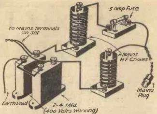
ent kinds of interference require Fig. 3.—A rather elaborate filter circuit which is useful in cases of different methods of prevention, serious electrical interference of the kind introduced by the mains leads.
