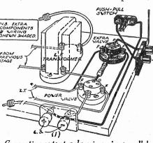
Connecting output valves in series-parallel,
