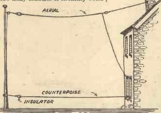
Fig. 1.—How to fix up a simple counterpoise earth.
