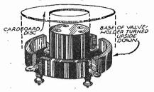
Adapting an ordinary valve-holder for chassis mounting.
