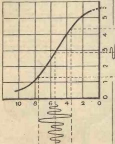
Fig. 1—The curve of a valve biased to give even amplification. The lower line gives grid volts, and the right-hand line gives anode current.
