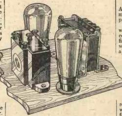
Fig. 6.—One way of adding a valve is to connect it in push-pull with the existing output valve. The lay-out for such an arrangement is shown here.
