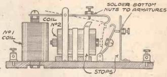
Fig. 10.—Showing top armature in action at the moment of energising No. 1 coil. The armature is clear of its stop for a moment, and this frees the bottom armature which is shown dropped clear by its own weight. The dotted lines show the previous position of the armatures. Top armature drops back on to its stop after being momentarily energised.
