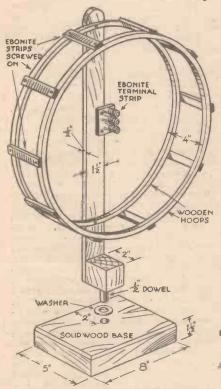
Fig. 2.—This shows how a circular frame aerial can be made quite easily.
