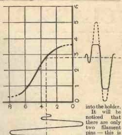
Fig. 2—The effect of grid current shown in diagrammatic form.
