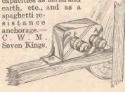
Using a fixed condenser case for a terminal block.
