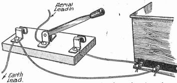
Fig. 2.—The connections to a single-pole aerial-earth switch.
