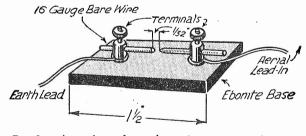
Fig. 3.—A simply made spark gap for connecting between the aerial and earth.
