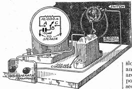
Simple device for controlling frequency response.
