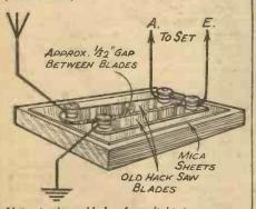
Using hacksaw blades for a lightning arrester.
