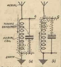
Fig. 3 (a) and (b).-Diagram illustrating the flow of electric currents in the aerial circuit of a receiver.
