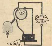
Fig. 6 .- Controlling the tone and eliminating needle scratch.
