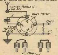
A handy plug and socket switching device.
