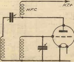
Fig. 2.— A typical reaction circuit.
