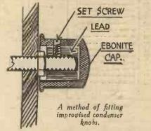
slot with a hack-saw to take a screw-driver. You will find that the head, owing to the moulded threads in the cap, will show no tendency to work loose; besides, the set-screw, if you leave it just long enough, will prevent this. The space between the lead and the end of the cap, allows it to fit over the "one-hole fixing" nut of the com-
