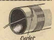
Fig. 2.—Another method of anchoring the end of a coil.
