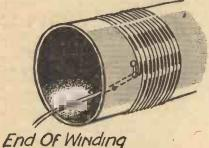
Fig. 1.—Anchoring the end of a coil by means of a loop through two holes.
