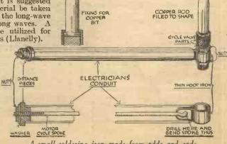
A small soldering iron-made-from odds and ends.
