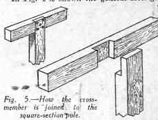
ment for a horizontal dipole, the insulators being mounted on the cross-member at the centre, which is also shown in Fig. 5 half-lapped into the square section pole.
