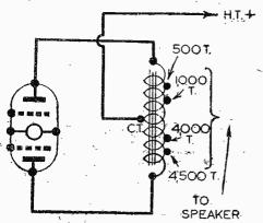
Fig. 2.—Diagram of connections and tappings to the Class Boutput choke.
