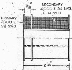
Fig. 1. Method of dividing primary and secondary windings with a spacing cheek.
