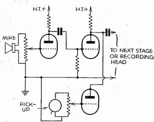
Fig. 3.—To obtain a balanced output, additional amplification for an insensitive mike may be obtained as shown here.
