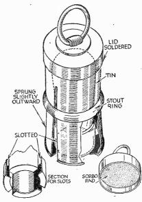
A useful device for removing tight-fitting valves.
