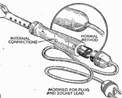
An improved method of connecting an electric soldering iron.
