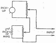
Fig. 2.—The simplest form of mixing circuit for mikes and/or pich-ups.
