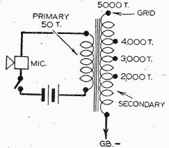
Fig. 3.—Arrangement of windings and connections in the microphone transformer described.
