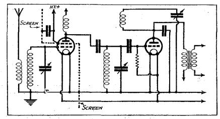
Fig. 3. The valve through the screen shows clearly which components must be to the left of the screen and vice versa.
