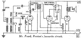
indeed, it is so much so that there is a decided "cut-off" of high notes. The cut-off is purposely arranged for in the tuning circuit, but all the higher notes can be restored to any desired extent by adjustment of the variable resistance operating | in push-pull. A moving coil loud-speaker |
