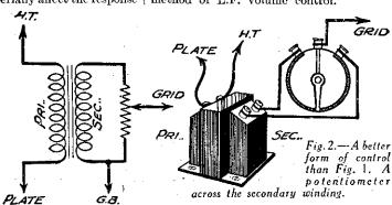
secondary winding-In this case the value of the resistance across the transformer the whole
