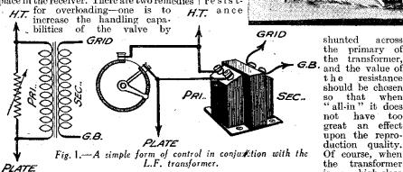
applying more H.T., and the other is to cut down the signal strength.
