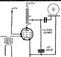
Fig. 7.—Tapped output choke and tone corrector.
