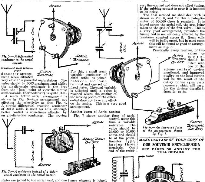
plates are joined to the aerial lead, and one set of fixed plates is joined to earth and the other end to the aerial terminal of the This gives a very smooth control of volume and does not materially alter the tuning of the set. A more elaborate version, for use in band pass circuits and other critical tuned circuits, is shown in Fig. 6.
