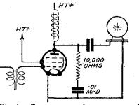
Fig. 6.—Tone corrector for using a standard speaker with pentode.
