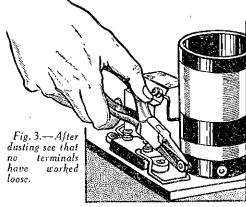
the terminals are serewed down tightly (a twist with a pair of pliers will do) and examine the contacts of the switches (see Figs. 3 and 4). The filament switch is
