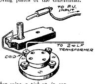
When using a pick-up in con-junction with two L.F. stages, the usual panel switch or jack arrangement for bringing the pick-up into circuit generally in-volves a long grid lead and return. This can be obviated by using two old plug-in coil-holders as shown.
