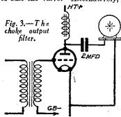
manufacturers wind the coil to a high resistance to any specification. The majority, however make a serious mistake as, when asked to supply a loud-speaker to match a particular valve, they wind the coil so that it has the same resistance as the valve impedance.
