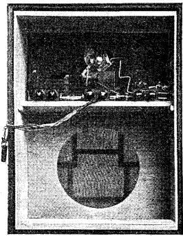
–A rear view of the set showing the fillet supports for the baseboard and the roomy compartment for the speaker and batteries.
