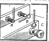
Fig. 3.—Instead of soldering the straight end of a wire to a terminal stem, it is much better to bend the end of the wire into a loop and then solder it.
