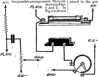
Fig. 3.—A potentiometer used instead of the grid leak in an R.C. amplifier,
