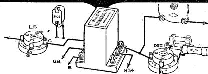
Brilliant reproduction is assured by incorporating this new unit in place of existing L.F. Transformer. This diagram illustrates the simple connections, and, once diagram indistrates the simple connections, and, once incorporated you will be astounded at the evenuess of amplification and enormous improvement in bass and treble response. Universal type for use in all receivers. Fitted in a few minutes by even inexperienced amateur constructors. One of the greatest successes at Radiolympia.
