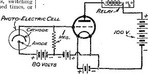
this particular cell, and it The standard method of connecting the photo-electric cell,
