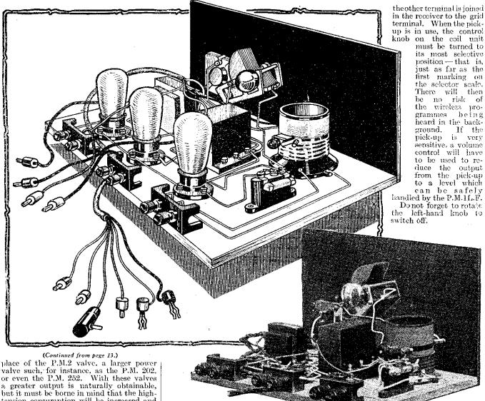
but it must be borne in mind that the hightension consumption will be increased and this will destroy one of the features of this receiver—economical running.
