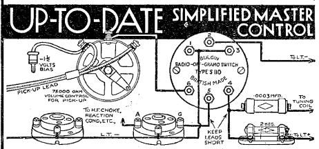
Bulgin S.110 Switch is a D.P.D.T. type with central "OFF" position. It gives complete control over the Radio/gramo and On/Off switching of a battery set. The diagram clearly shows the connections. The normal connections for a Volume Control the connections. The normal connection use with a pick-up are also shown.
