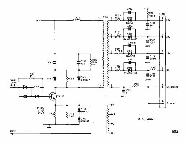
Fig. 2: Main power supply differences in stereo models. In addition:
