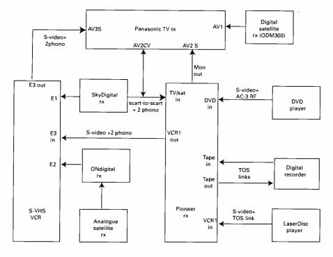
Fig. 2: Wiring diagram for the author's AV system. All unspecified cables are scart-to-scart. that out. As the DVD player, a Pioneer DV505, stores the last fifty disc set-ups in memory, I would probably have to change the setting for each disc in turn.
