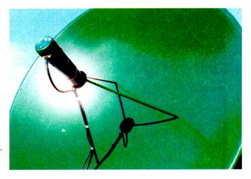
aligned on-axis – the shadow at the centre of the surface of the dish should be an end-on one, see photo above.
