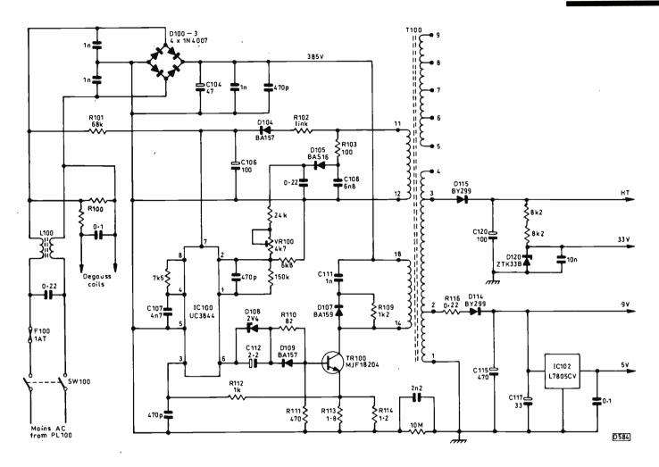
Fig. 1: The chopper power supply circuit used in mono-sound versions of the Grundig G1000 chassis.
