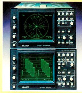
Two precision video monitors in the Leader 5000 range are now available from TTi. The 5212 vectorscope and 5222 waveform monitor offer multi-channel inputs for both composite and component signals, with automatic PAL/NTSC selection. Line selection with the 5222 enables BITS, VIR and teletext lines to be observed. For further information apply to Thurlby Thandar Instruments Ltd., 2 Glebe Road, Huntingdon, Cambs PE18 7DX. Tel 01480 412 451, fax 01480 450 409.
