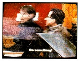
Photo 12: A satellite D-MAC signal makes a nice mess of UHF ch. 47 reception. In this case the outlet plate crosstalk was –30dB. Matters were made worse by a UHF signal at –10dB/mV.
