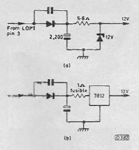
Fig. 1: Top (a) the zener diode 12V regulator circuit that's used in many Alba/Bush and other sets (Onwa chassis). Bottom (b) Mel's mod, using a 7812 regulator instead. It would be preferable to add 0.1µF decoupling capacitors at the regulator's input and output.
