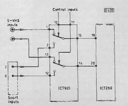
Fig. 1: The audio switching arrangement used in versions of the Philips G110 chassis with S-VHS provision.
