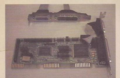
Typical I/O card for an ISA slot. result that you would have to enter the drive parameters (cylinders, tracks, sectors) into the BIOS set-up screen manually. If you have fitted one to the second IDE channel you are unlikely to have even this option.
