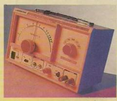
AG2601 is a portable mainspowered instrument covering 10Hz to 1MHz in five overlapping decades. Sinewave distortion between 500Hz and 50kHz is just 0.05%.
