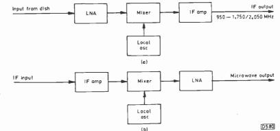
Fig. 1: Block diagrams showing at (a) the basic LNB arrangement and at (b) the LNB rearranged as an up-converter. Fig. 2: I.F. amplifier modifications: the initial arrangement – to clarify the situation most of the components are not shown.
