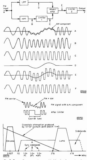
Fig. 7: Crosstalk attenuation provided by the slant azimuth technique over the range of frequencies within the standard VHS signal spectrum.
