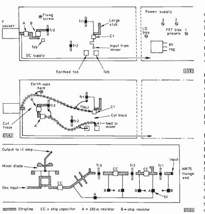
Fig. 2. The GaAs FETs require a small negative gate bias which is generated by the i.c. The three co-located presets power each LNA stage, the end one. by the 8V regulator, providing bias for the oscillator FET.
