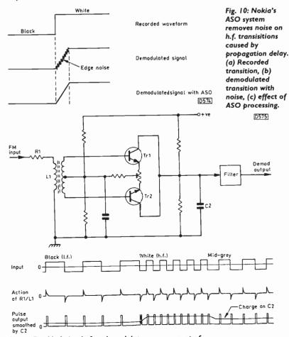
Above, Fig. 11: A simple f.m. demodulator arrangement of the frequency doubling and pulse-counting type.
