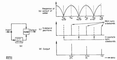
Fig. 9: A comb filter arrnagement used to cancel crosstalk between line sync sidebands. Fsc is the carrier frequency, f the line frequency (15·625kHz). At points Fsc + 0·5f, Fsc + 1·5f etc. the crosstalk will cancel.
