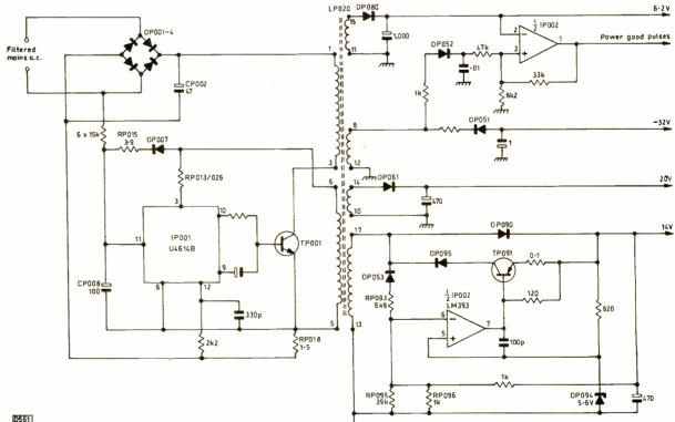
Fig. 1: Simplified circuit of the power supply used in mono sound models.
