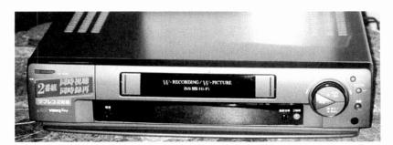
Sharp's VCBF80 dualrecording capability VCR. would cost! So far the technique is available only for NTSC operation: one wonders whether the same principle could be adopted for PAL, given the narrower video tracks.
