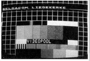
Belgacom Liedekerke, a Belgian SNG identification, inserted in the field blanking period. The identification can be seen by adjusting the field hold control so that the field slips down.
