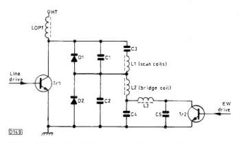
Fig. 8: Basic form of diode modulator. Transistor Tr2 controls its operation.
