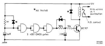
Fig. 4: Circuit to select channel one on powering the Amstrad SRX100. A small RS DIL relay with a normally-open contact was used: wire the contact across the channel 1 pushbutton.
