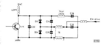
Fig. 11: Diode-modulator circuit with a coupling transformer, used to drive a Philips 110° tube.
