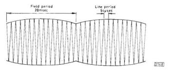
Fig. 7: Use of a parabolic field-frequency waveform to amplitude modulate the line-scan current – not to scale.
