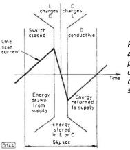
Fig. 3: The switching and energy-interchange phases during one complete cycle of operation of the circuit shown in Fig. 1.
