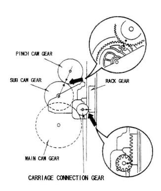
Fig. 7: Gear phase alignment, bottom view.
