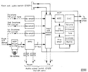
Fig. 2: Block diagram of the audio processing system (full options).
