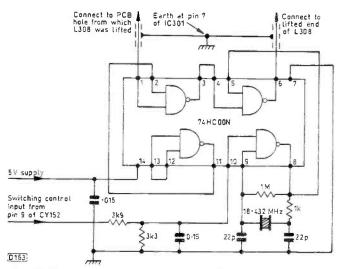
Fig. 5: Circuit to enable extra sound channels to be received with the Amstrad Models SRX100 and SRX200.
