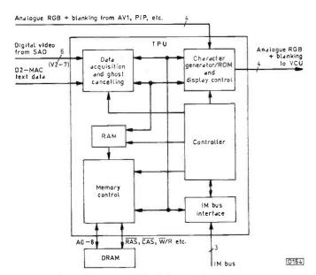
Fig. 1: Block diagram of the teletext circuit.
