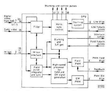
Fig. 3: Simplified block diagram of the DPU chip.
