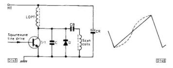
Fig. 4 (left): Basic elements of a practical line output stage. The scan coils are capacitively coupled and the output transformer acts as a loading choke.
