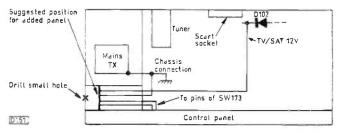
Fig. 3: Connection points and suggested position for the circuit shown in Fig. 2. A small hole in the case will enable the step speed to be adjusted easily. If a scart lead is used the control wire at pin 8 must be removed.
