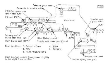
Fig. 8: Post and main-lever position in each mode.
