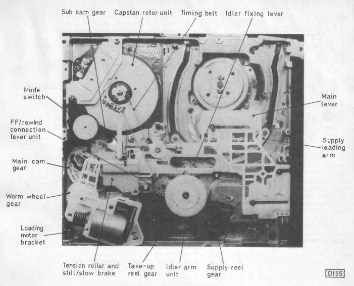
Fig. 2: Bottom view of the K mechanism.
