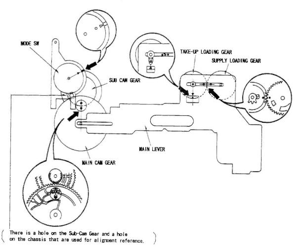
Fig. 6: Gear phase alignment, top view.
