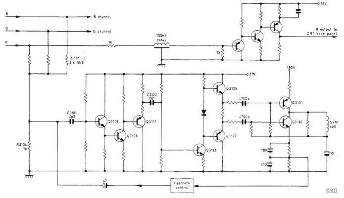
Fig. 4: The SVM board circuitry, simplified and with only the red channel is shown.
