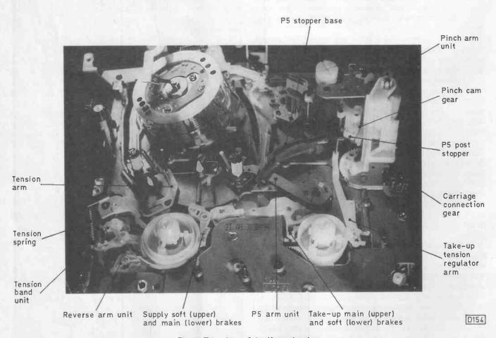
Fig. 1: Top view of the K mechanism.
