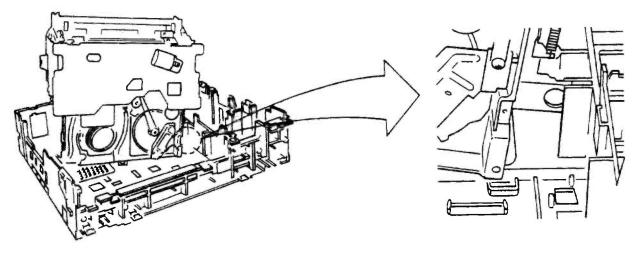
Fig. 4: Service position for the K deck. The mechanism can be easily fixed by standing it up in the main frame as shown.
