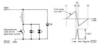
Fig. 1 (left): Theoretical representation of the bare essentials of a TV line output stage.
