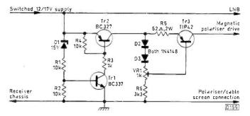
Fig. 1: Circuit for providing magnetic polariser switching with the Grundig GRD2000 satellite receiver.
