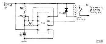
Fig. 2: Circuit for providing simple channel stepping with the Amstrad SRX200 receiver.
