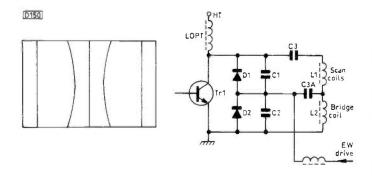
Fig. 9 (left): The inner pincushion distortion (exaggerated) inherent with some tube/yoke designs when simple pincushion-distortion correction is applied.
