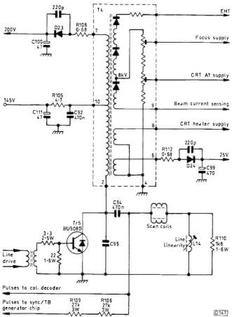
Fig. 6: Practical line output stage circuit used to drive 90° 20 and 22in. tubes. All the components in the brokenline box are encapsulated within the line output transformer T4. The value of the flyback tuning capacitor C95 varies with tube size: it's 10nF with a 22in. tube and 9.1nF with a 20in. tube.
