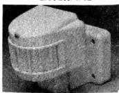
Simply connect to existing external lighting. Swivel mounted passive infra red sensor for the detection of body heat. The mounting asrrangement allows horizontal and vertical swivel of 180°, allowing difficult to reach areas to be covered by the beams. A built-in adjustable photo detector prevents daylight operation. Adjustable timed on period. Provided with a walk test LED.
