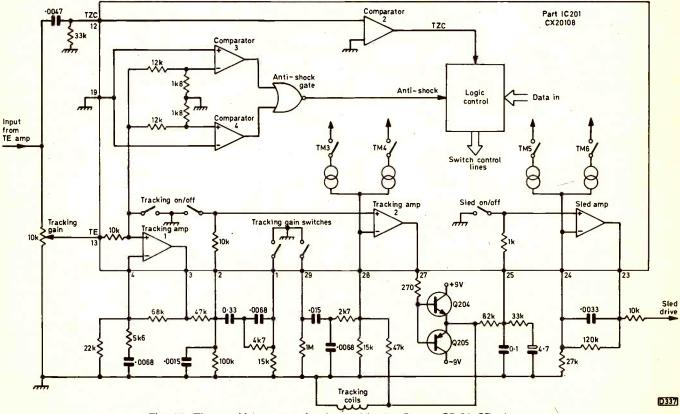
Fig. 11: The tracking servo circuit used in the Sanyo CP-08 CD player.
