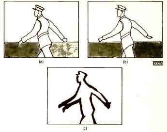
Fig. 3: Sketches – (a) and (b) – of two consecutive pictures from a camera shot. The black areas in (c) show roughly the difference between (a) and (b). Note that the background remains the same from (a) to (b).
