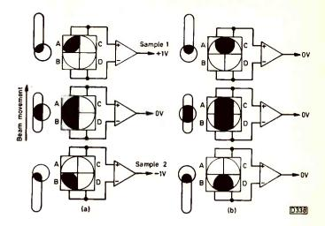
Fig. 12: Sony method of obtaining a tracking error signal with a single-beam laser assembly.
