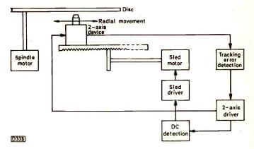
Fig. 7: The joint action of the two-axis device and the sled maintains correct tracking. The tracking arrangements must be able to operate in the forward and reverse directions so that tracking is also maintained in the reverse search mode.
