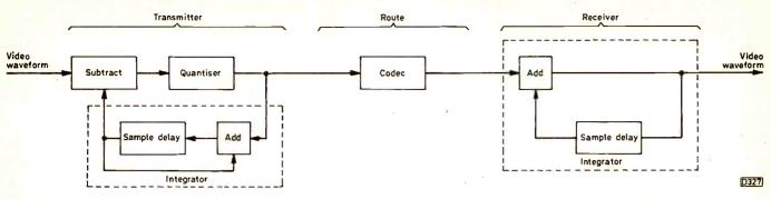
Fig. 5: An early digital compression system for videophone use, based on differential pulse code modulation.
