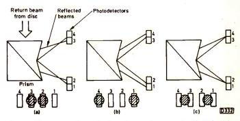
Fig. 6: Philips method of obtaining a focus error signal with a single-beam laser assembly. (a) Lens too far from the disc, (b) lens too close, (c) correct focus.
