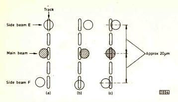
Fig. 8: Obtaining a tracking feedback signal with a threebeam assembly. (a) Mistracking to left: E - F is less than zero. (b) Mistracking to right: E - F is greater than zero. (c) Correct tracking. E - F = 0V.
