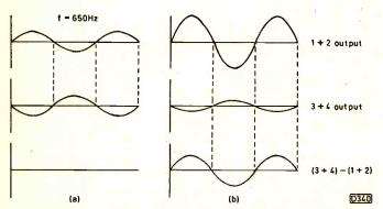
Fig. 14: Principle of the additional fine tracking system in the Philips single-beam arrangement: (a) shows correct tracking, (b) incorrect tracking.
