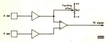
Fig. 9: Amplification and addition of the E and F signals.
