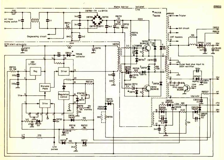
Fig. 1: The Ipsalo circuit used in the Salora J chassis. RB507 is 3·9kΩ in 22/26in. sets, 2·2kΩ in 20in. sets; RB726 is 56Ω in 22/26in. sets, 82Ω in 20in. sets; RB739, 560kΩ, is fitted in 20in. sets only; RB706 is 2·7kΩ in 22/26in. sets, 15kΩ in 20in. sets (4W in both cases); CB707 is 1nF in 22/26in. sets, 270pF in 20in. sets (1kV in both cases).
