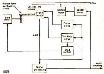
Fig. 1: Block diagram of a CD player's servos.
