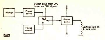
Fig. 3: Basic focus servo system.
