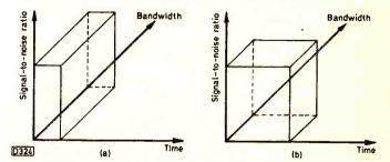
Fig. 2: Three-dimensional diagram illustrating the relationship between bandwidth, time and signal-to-noise ratio. In (b) the time taken to transmit the vision information is longer than in (a) so the bandwidth can be less.
