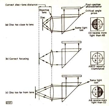
Fig. 5: Sony method of obtaining a focus error signal with a single-beam laser assembly.
