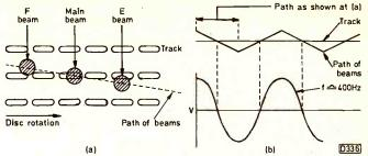
Fig. 10: Because the track spirals outwards, there is a continuous tendency towards incorrect tracking. This is shown at (a). As a result, the tracking error signal is cyclical with a frequency of about 400Hz, as shown at (b).
