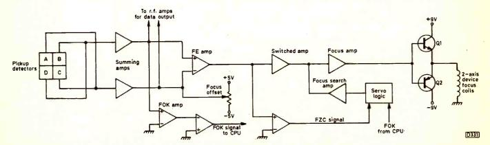
Fig. 4: Typical focus servo system. In most players the FOK signal is available at the pin of an i.c. and is a useful check to show that the beam is correctly focused.
