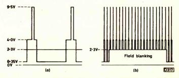
Fig. 2: The sandcastle pulse waveform at pin 7 of ICB200. (a) At line rate, (b) at field rate.
