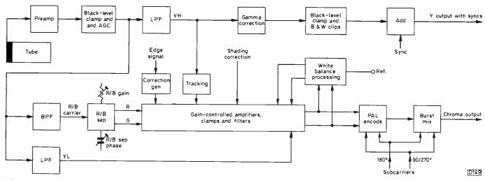
Fig. 5: Block diagram of a typical colour video camera using a pick-up tube.
