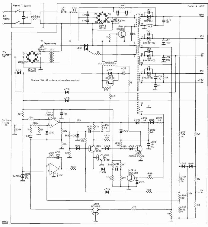
Fig. 4: The chopper power supply circuit. In earlier versions 4R32 was  $3.9k\Omega$  with 4R99 and 4R100 omitted. There have been other minor modifications to the circuit.
