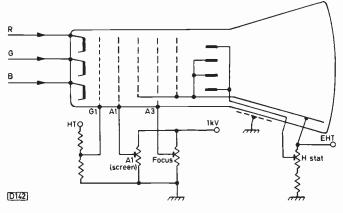
Fig. 2: Inputs to the various electrodes.
