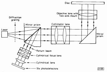
Fig. 4: Arrangement of the flat optical pickup (FOP).
