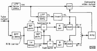
Fig. 4: Block diagram of the R/B signal separation system.
