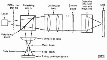
Fig. 1: Arrangement of the various items that comprise the T-type three-beam laser optical unit.
