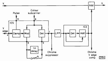
Fig. 11: Block diagram of the edge compensation system.
