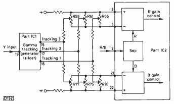
Fig. 9: Basic triple-level tracking circuit.
