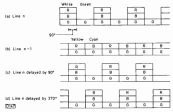
Fig. 3: Separating the R and B components of the R/B carrier signal obtained from the tube.
