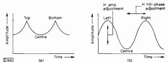
Fig. 5: Waveforms present at the dynamic convergence coils, (a) for vertical axis correction (field rate parabola), (b) for horizontal axis correction (line rate sinewave).
