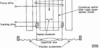
Fig. 8: Basic arrangement of the two-axis mounting for the objective lens, giving focus and fine tracking adjustment.
