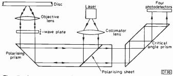
Fig. 5: Arrangement of the single-beam laser assembly used in some Sony CD players.
