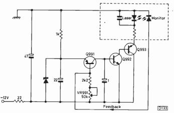
*Fig. 2: Laser current stabilising circuit used in an early Mitsubishi CD player.*
