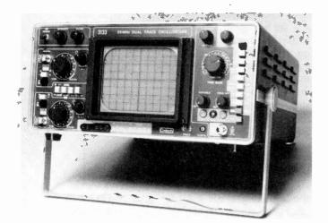
The Crotech 3133 25MHz dual-trace oscilloscope. TELEVISION APRIL 1989
