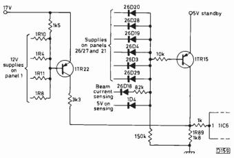
Fig. 3: The power failure detection circuit.
