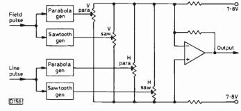
Fig. 13: Method of producing the dynamic focusing and the shading correction waveforms.
