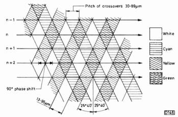
Fig. 2: The colour stripe filter arrangement.
