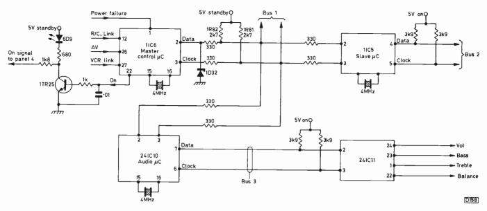
Fig. 2: Outline of the microcomputer control system.
