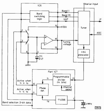
Fig. 5: The frequency synthesis tuning system.
