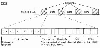
Fig. 3: The address code system.
