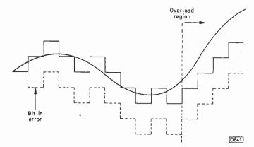
Fig. 12: Differential pulse-code modulation (PCM) signal, showing bit error and overloading.
