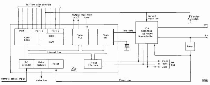
Fig. 7: Block diagram of the 2070 central control unit chip and its associated EEPROM.
