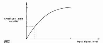
Fig. 3: Non-linear quantization characteristic.
