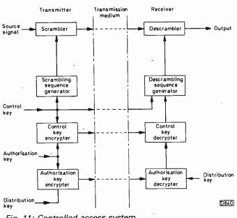
Fig. 11: Controlled access system.
