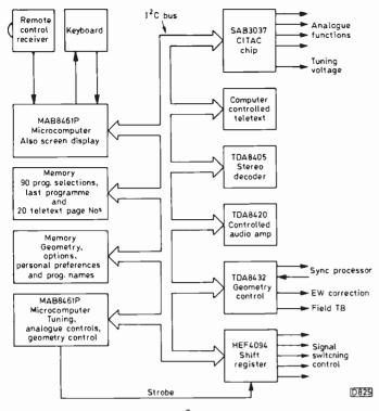
Fig. 1: Connections via the  $l^2C$  bus between the two microcomputer chips and the chips they control.
