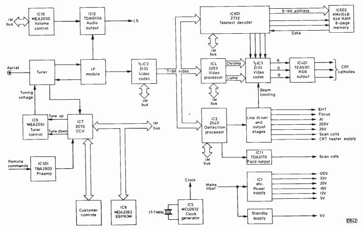
Fig. 1: Block diagram of the Fidelity ZX5000 chassis.
