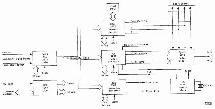
Fig. 2: Block diagram of the digital signal processing sections of the receiver.
