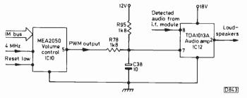
Fig. 4: Block diagram of the a.f. section.
