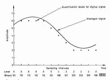
Fig. 1: Sampling and quantization.
