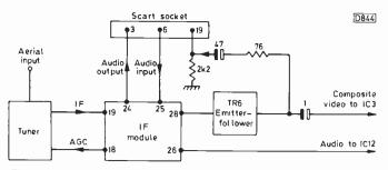
Fig. 3: Block diagram of the tuner and i.f. sections of the receiver.
