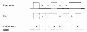
Fig. 8: A simple encryption system.
