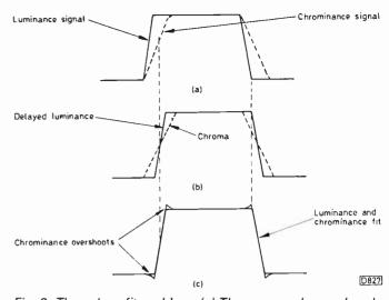
Fig. 3: The colour fit problem. (a) The narrow chroma bandwidth has the effect of displacing the colour to the right. (b) By delaying the luminance the two signals fit but the chroma is still diffused at the transients. (c) Colour transient improvement straightens the rise time of high-amplitude chroma transients to give accurate superimposition of the luminance and colour at the screen.
