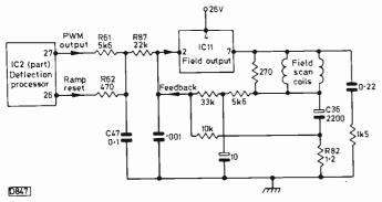
Fig. 6: Field timebase arrangement.
