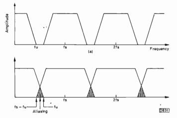
Fig. 2: Frequency spectrum for Nyquist sampling (a); introduction of aliasing (b).
