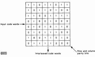
Fig. 6: Interleaved code words.
