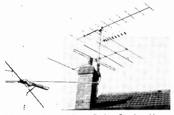
Mark Baldwin's aerials at Rugby. On the chimney, wideband arrays for Bands I/III and u.h.f. In the foreground, the classic Band I omnidirectional X array.
