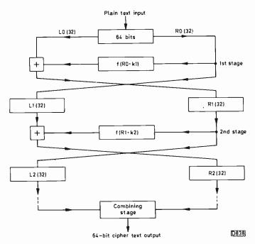
Fig. 9: DES encryption algorithm.
