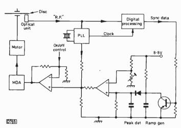
Fig. 6: Simplified diagram showing the arrangement used for motor control in compact disc players.
