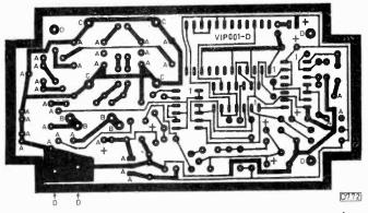
Fig. 3: PCB drilling details. All holes 0.8mm except A = 1.2mm (32), B = 1.5mm (4), C = 1.8mm (4), D = 3mm (5).
