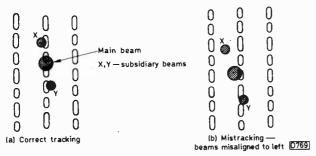
Fig. 10: The main scanning beam is accompanied by two tracking beams: (a) shows correct tracking, (b) mistracking.
