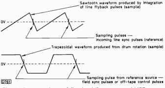
Fig. 2: A comparison of flywheel line sync and VCR servo waveforms.
