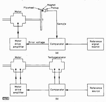
Fig. 1: Basic servo arrangements, (a) with sample signal taken from a flywheel and (b) with the sample signal provided by a tacho-generator.
