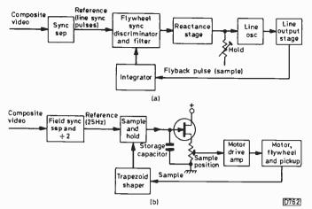
Fig. 3: Block diagrams of basic TV flywheel line sync and VCR servo arrangements.
