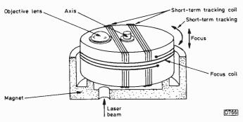
Fig. 7: Two-axis device used to provide optical unit tracking and focusing with laser-scanned disc players.
