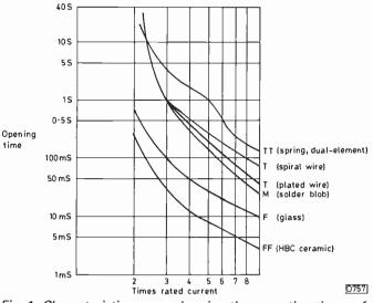
Fig. 1: Characteristic curves showing the operating times of different types of fuses. Note that there's a considerable tolerance in fuse performance.
