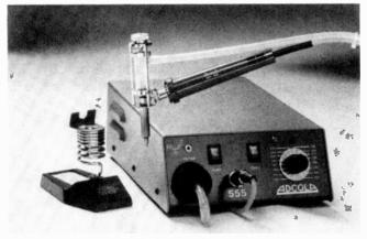
The Adcola 555 desoldering station.
