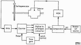
Fig. 5: Block diagram of a simple digital servo system used to provide motor speed control.
