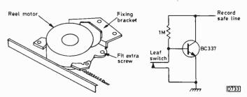
Fig. 1 (left): Modification suggested by Toshiba for Models V71 and V73.
