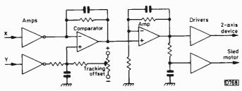
Fig. 9: CD player tracking servo system.
