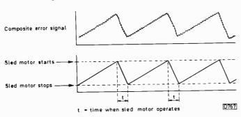
Fig. 8: Disc tracking.
