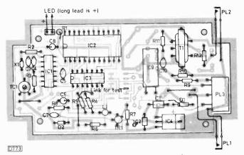
Fig. 4: Component layout. Fit R3 to clear TC1.
