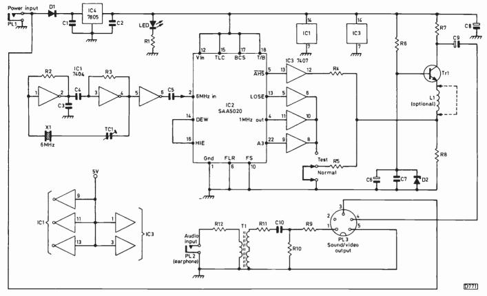
Fig. 1: Circuit diagram of the VCR sound interface unit.
