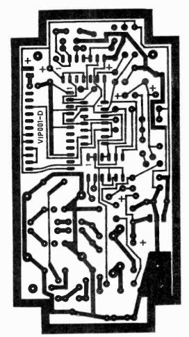
Fig. 2: PCB print layout. Standard, single-sided 1/16in. fibreglass is suitable. To complete, cut along inside the black border line.
