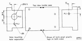
Fig. 5: Case drilling details (not to scale). All dimensions in mm. The lid requires a 3·1mm diameter hole for the LED.
