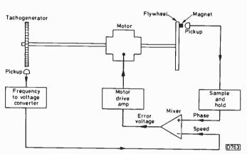
Fig. 4: Block diagram of a twin-loop servo for speed and phase control of a motor.
