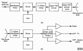
Fig. 1: Block diagram of the transmitter section of an MMD system (a) and the receiver section (b).
