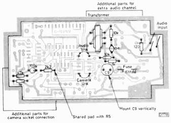
Fig. 9: Component layout details for the extra options.
