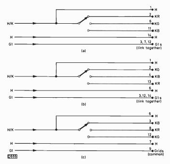
Fig. 4: Common c.r.t. base connections. (a) Delta-gun tube. (b) 20AX tube. (c) PIL tube.
