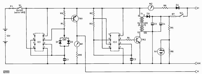
Fig. 1: Circuit diagram of the tube tester-booster.
