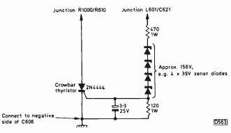
Fig. 9: Suggested crowbar over-voltage protection circuit.
