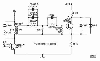
Fig. 5: Line output transistor drive circuit for the Sony KV1810UB. Leave L508 in circuit in the Mk. I version.
