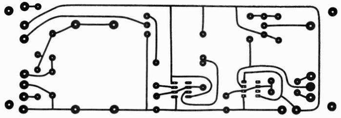
Fig. 3: PCB track pattern used in the prototype.
