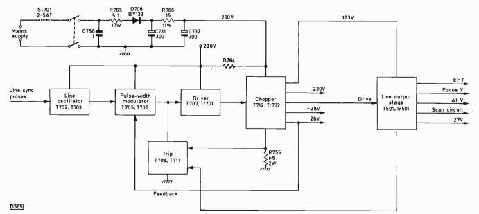
Fig. 1: Block diagram showing the power supply arrangements used in the ITT Model FT110. R764 (3·3k $\Omega$ , 4W) provides a start-up feed.
