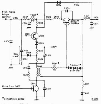
Fig. 2: Modified chopper circuit.
