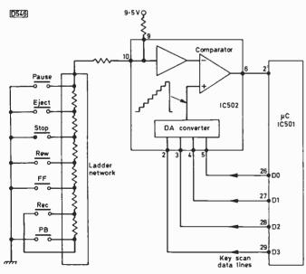
Fig. 1: Block diagram of the electronic function control system used in the Fisher FVH615. The arrangement is widely used in "electronic" VCRs.
