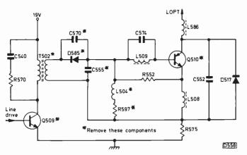
Fig. 3: Line output GCS drive circuit used in the Mk. I version of the Sony KV1810UB.
