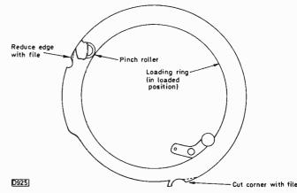
Fig. 1: Loading ring modification for the VTC5300/5400.
