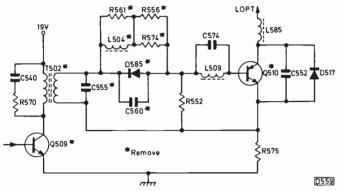
Fig. 4: Line output GCS drive circuit used in the Mk. II version of the Sony KV1810UB.
