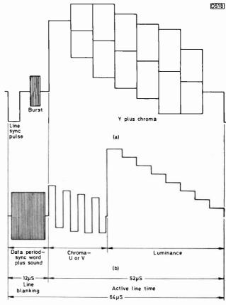
Fig. 2: (a) A single line of PAL carrying a colour-bar signal. (b) A single line of MAC, again with a colour-bar signal. The seven-bit sync word plus digital sound and data occupy the line blanking period.
