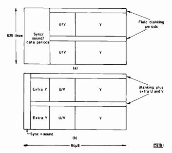
Fig. 3: (a) Layout of one field of MAC. (b) Layout of one field of Extended-MAC.
