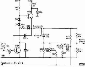
Fig. 4: The field output stage circuit.
