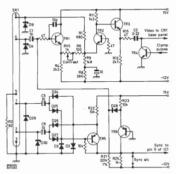
Fig. 2: The video and sync processing circuitry.
