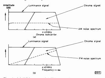
Fig. 1: (a) With terrestrial TV transmissions the "white" noise affects the luminance and chroma signals equally. (b) With an f.m. transmission the "pink" noise increases with frequency, discriminating against the colour signal.
