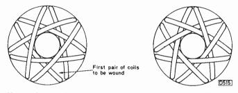
Fig. 5: Comparison between direct and former windings.
