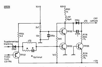
Fig. 3: The video amplifier and beam limiter circuits.
