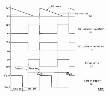
Fig. 5: Spectrum analyser waveforms. Note that as the direction of the line scan has been reversed screen display (e) is the mirror image of the drive (d).
