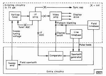
Fig 2: Block diagram of the spectrum analyser.
