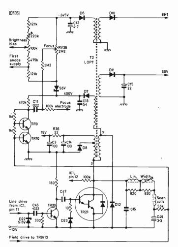
Fig. 5: The line driver, line output and dynamic focusing drive circuits.
