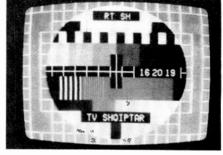
Left: Tropospheric reception of NRK (Norway) ch. E29 in Holland. Centre: The FUBK test pattern in use by NOS (Holland). Right: Albanian PM5534 test pattern received in Holland on ch. IC via SpE. Photographs courtesy Ryn Muntjewerff.
