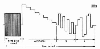
Fig. 4: S-MAC, a variation favoured in the USA for studio work. Having the entire signal on one line makes for simpler mixing and trick work.
