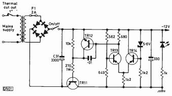
Fig. 1: The regulated power supply circuit.
