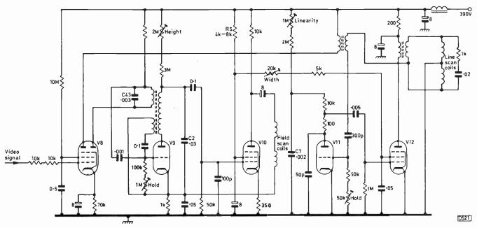
Fig. 1: The timebase circuitry used in the Cossor Model 1210.
