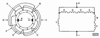
Fig. 3: Wave winding.
