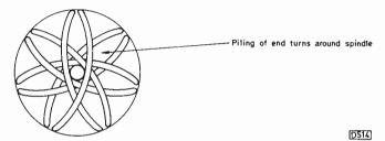
Fig. 4: A winding span of more than 180°.
