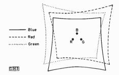
Fig. 3: The inherent raster geometry errors with a delta-gun tube.
