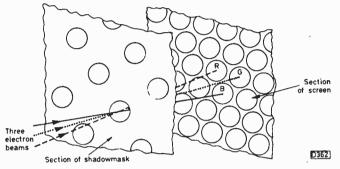
Fig. 2: Trajectories of the beams in a delta-gun tube. In practice each beam is larger than one shadowmask hole.
