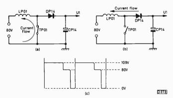
Fig. 1: Principle of the step-up power supply. (a) Chopper transistor on. (b) Chopper transistor off. (c) Waveform at the collector of TP01.
