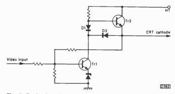
Fig. 6: Basic class AB video output circuit.
