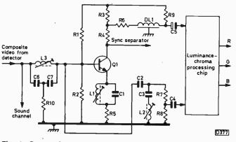
Fig. 1: Separating the outputs from the vision detector.
