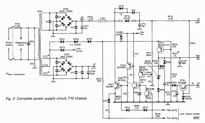
input. The line flyback pulses thus switch TP04 on sooner or later as the mains input is varied over the range 150-260V.
