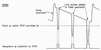
Fig. 4: Showing the way in which adding line pulses (three only shown) to a field sawtooth waveform gives pulse width modulation at the collector of TF07 so that DF08 is switched on progressively earlier as the field scan progresses.
