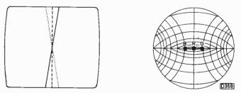
Fig. 10 (left): Errors arising from vertical deflection of in-line beams by a homogeneous magnetic field.
