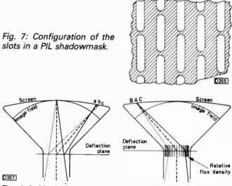
Fig. 8 (left): An in-line gun array projecting three beams through a homogeneous deflection field.
