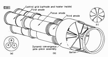
Fig. 1: The thick-neck, delta-gun arrangement. (a) Positions of the three guns in the tube neck. (b) Configuration of the gun electrodes and convergence pole-pieces. (c) Axial view of the pole-pieces mounted at the end of the guns: the polepieces guide the magnetic fields from the adjacent radial convergence coils.
