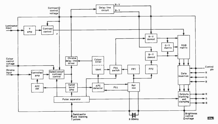
Fig. 2: Block diagram of the TDA3560 luminance and chroma signal processing chip.
