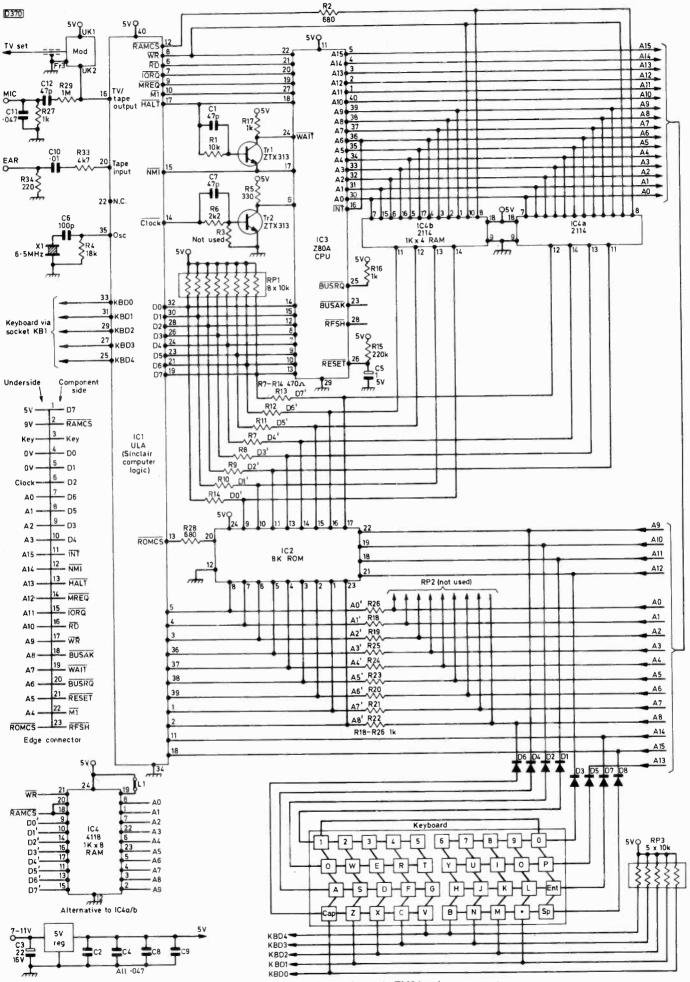
Fig. 1: Basic circuit diagram for the Sinclair ZX81 microcomputer.
