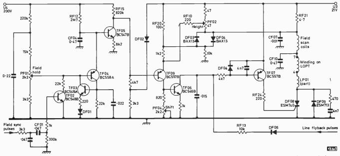
Fig. 3: Complete field timebase circuit, F10 chassis. RF12 is 3-3Ω in the F11 chassis – there are other minor variations.
