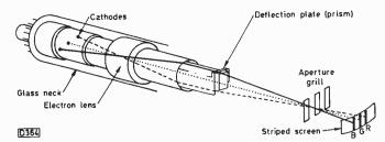
Fig. 4: Principle of the Trinitron tube.
