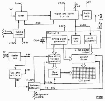
Fig. 1: Block diagram of Citizen's LCD TV receiver.
