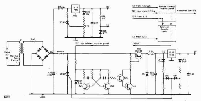
Fig. 1: The teletext decoder/remote control power supply arrangement used in early teletext versions of the Philips G11 chassis. The circuit is shown in basic outline only.
