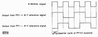
Fig. 3: Obtaining quadrature reference signals to drive the R – Y and B – Y demodulators by using two flipflops to divide by two the output from an 8-86MHz oscillator. FF2 is positive-going edge triggered to produce an in-phase 4-43MHz signal; FF1 is negative-edge triggered to produce a signal with a 90° phase difference.
