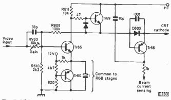
Fig. 7: Video output circuit used in the Thorn TX100 chassis.
