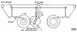
Fig. 6: Ribbon reversing mechanism.
