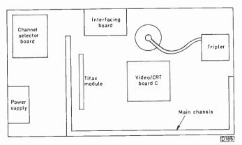
Fig. 10: Positions of the extra panels and the Tifax module in the Sony Model KV1820UB.
