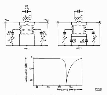
Fig. 1 (top left): Czech notch filter. Fig. 2 (top right): Version for use with a d.c. feed.
