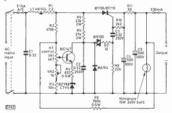
Fig. 1: Circuit of the variable stabilised h.t. supply.
