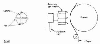
Fig. 5: Printer/plotter system.
