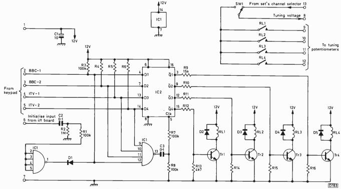
Fig. 5: Remote channel selector circuit.
