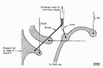
Fig. 4: Method of tapping the video from board A in the Sony Model KV1820UB.
