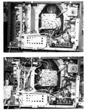
The Sony KV1820UB before (top) and after (bottom) adding teletext and remote channel selection/sound muting.
