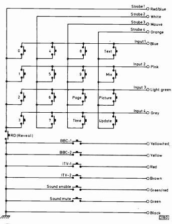
Fig. 2: Circuit of the keypad.
