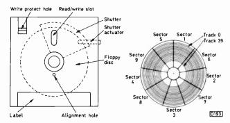
Fig. 1 (left): Three inch floppy disc. Fig. 2 (right): Arrangement of tracks and sectors.
