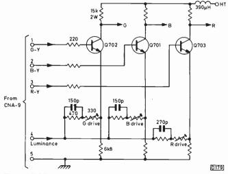
Fig. 1: RGB output stage circuits, Sony Model KV1820UB.
