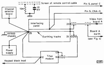
Fig. 7: Recommended earthing arrangements.
