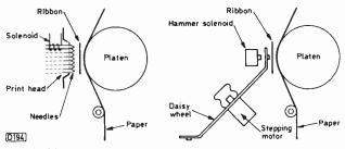
Fig. 3 (left): Matrix printer operation. Fig. 4 (right): Daisy wheel printer operation.
