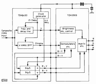
Fig. 2: Decoding with solid-state filters and delay lines.
