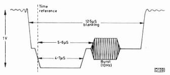
Fig. 1: Standard PAL line blanking period waveform.
