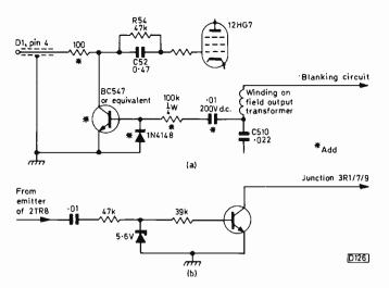
Fig. 3: Modifications for Beovision hybrid colour sets. (a) for 90° models, (b) for 110° models.
