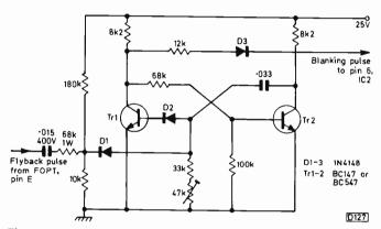
Fig. 4: Monostable multivibrator pulse-stretcher circuit for use with the Decca 30 series chassis. Adjust the preset just to clip the top of the picture.
