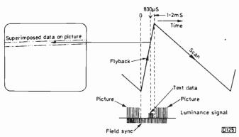
Fig. 2: The effects of slow flyback and inadequate blanking. Text pulses will be displayed on the screen if the beam is not fully extinguished during the flyback.
