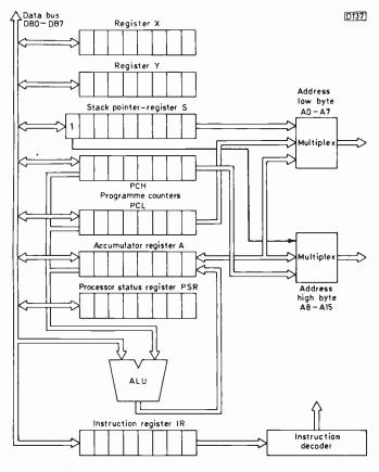
Fig. 1: Microprocessor architecture – the internal arrangements used in the 6502.
