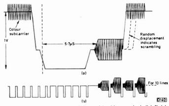
Fig. 2: SECAM waveform: (a) line blanking period, (b) field blanking period (part).
