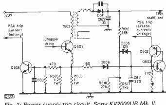
Fig. 1: Power supply trip circuit, Sony KV2000UB Mk. II.
