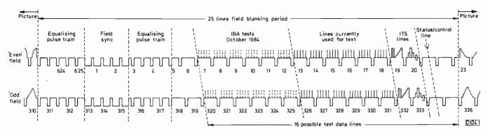
Fig. 1: The field blanking interval in the 625-line system, showing the sync pulses, text, control and ITS lines.
