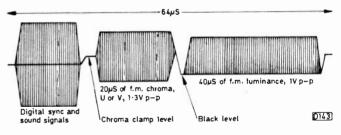
Fig. 5: MAC waveform for a complete line.
