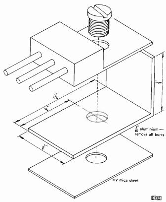
Fig. 1: Suggested heatsink arrangement for use with a BU426A transistor used as a chopper in the Sony Model KV1810UB. Use bush from the original GCS.
