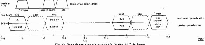
Fig. 6: Broadcast signals available in the 11GHz band.
