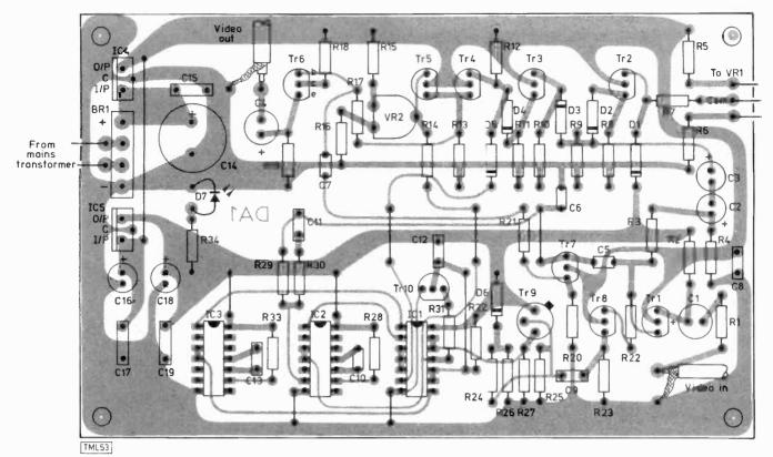
Fig. 2: Component layout on the PCB.
