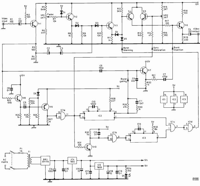
Fig. 1: Circuit diagram of the fader unit.
