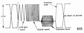
Fig. 4: Oak Orion encrypted signal waveform.
