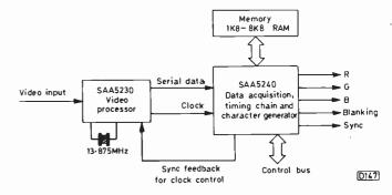
Fig. 3: Two-chip (plus memory) teletext decoder.
