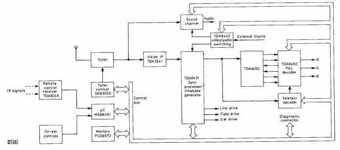
Fig. 4: Computer-controlled TV via a two-wire bidirectional bus.
