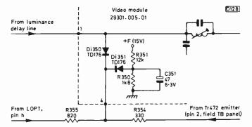
Fig. 5: Luminance blanking circuit used in Grundig sets with colour-difference tube drive. Di350, Di351, C351, R350, R351, R354 and R355 were not present in early production sets.
