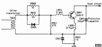
Fig. 1: Original circuit used in the Sony KV1820.
