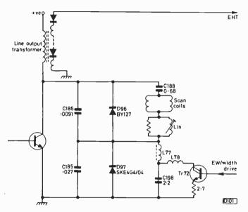
Fig. 5: Line output stage circuit used in the Thorn TX9 chassis – simplified to show basic operation.
