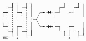
Fig. 2: Use of detectors to recover the two sides of the signal envelope.
