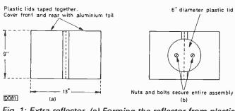
Fig. 1: Extra reflector. (a) Forming the reflector from plastic lids and aluminium foil. (b) Mounting arrangement.
