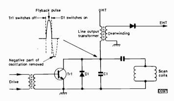
Fig. 1: Basic transistor line output stage.
