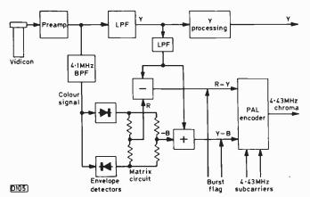
Fig. 3: Block diagram showing signal processing with the step energy recovery colour-separation system.
