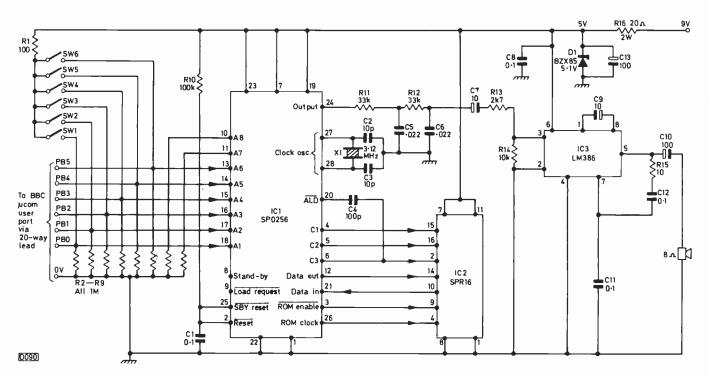
Fig. 2: The simplest way of using the SP0256/SPR16 combination to provide electronic speech.
