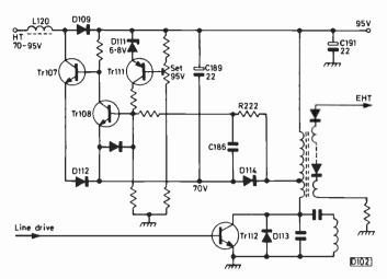
Fig. 6: Line output stage circuit – again simplified – used in the Thorn TX90 chassis, with chopper-controlled boost supply.
