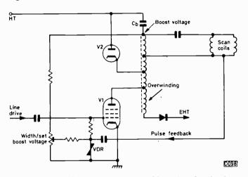
Fig. 2: Valve line output stage with pulse feedback to stabilise the operating conditions. The VDR acts as a pulse rectifier, producing a negative bias voltage proportional to pulse amplitude.
