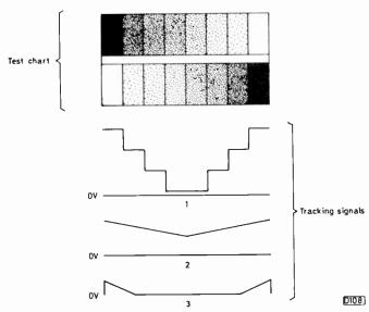
*Fig. 6: Double grey-scale wedge and tracking signals.* TELEVISION MARCH 1985
