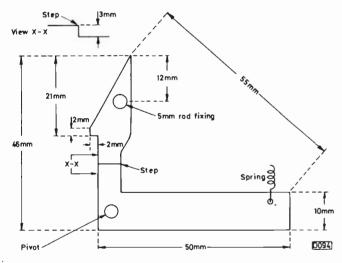
Fig. 2: L-shaped crank for holding the drum in the laced position. It may be necessary to adjust on assembly – what has to be done should be clear when the actual machine is on the bench.
