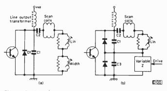
Fig. 4: Basic transistor line output stage with inductor to provide width control (a). Modified arrangement with highlevel EW diode modulator circuit (b).
