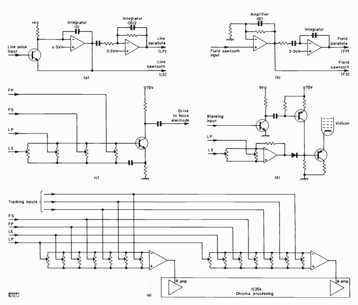
Fig. 5: Generating and using field and line frequency correction waveforms: (d) Shows dark current shading correction, (e) chroma shading correction.
