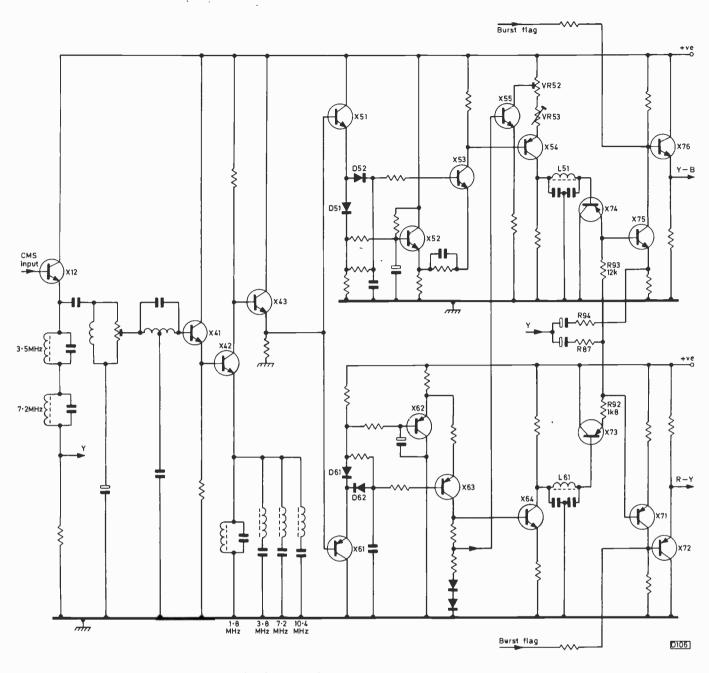
Fig. 4: Colour circuitry used in the Ferguson 3V06 camera – simplified.
