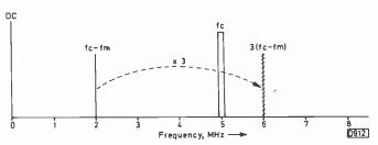
Fig. 6: Harmonic distortion of a modulated carrier: the third harmonic of the first lower sideband here gives rise to an interfering signal at 6MHz (fc 5MHz, fm 3MHz).
