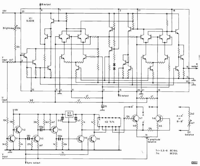
Fig. 1: Spectrum-monitor interface circuit for RGB drive.
