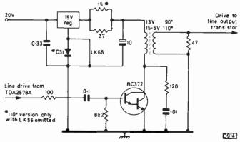
Fig. 2: The low-voltage line driver stage.
