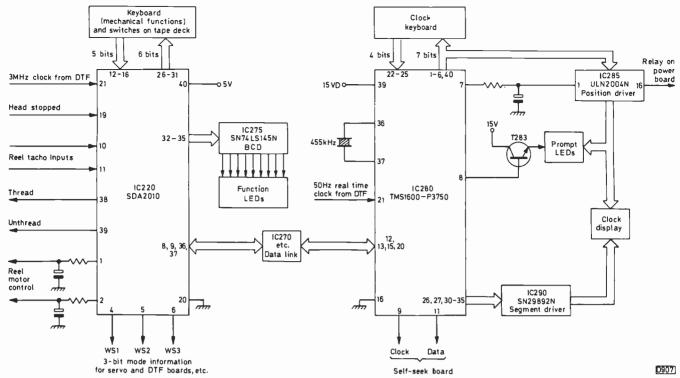
Fig. 2: The keyboard module - simplified block diagram.
