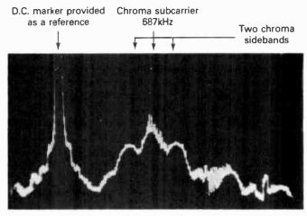
Fig. 7: Spectrum of a colour-under signal. This spectrum goes up to about 1.7MHz and shows the chroma subcarrier and its sidebands neatly contained within a total bandwidth of about 1MHz. Photo courtesy Sony (UK) Ltd.
