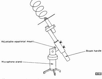
Fig. 4: The helical aerial mounted on its stand.
