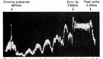
Fig. 4: Luminance and chroma signals and sidebands for colour bars on playback. This is for the Betamax system but others are similar. The modulator's deviation range can be clearly seen, along with the lower sideband energy distribution. The highly saturated colour bars give rise to considerable energy around the 687kHz down-converted colour subcarrier. Photo courtesy Sony (UK) Ltd.
