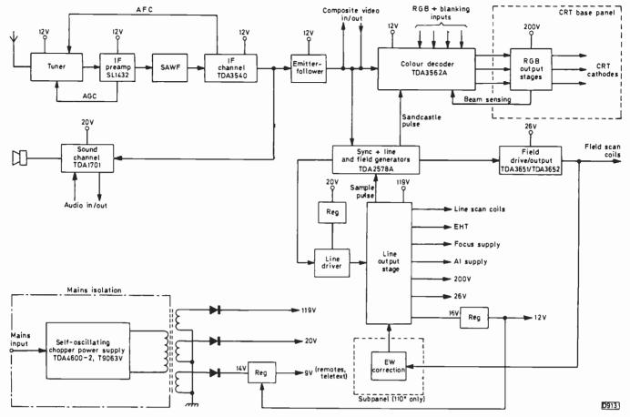
Fig. 1: Block diagram of the Ferguson TX100 chassis. A relay in the 119V line gives remote standby.
