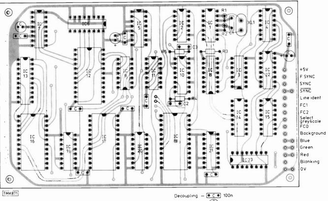
Fig. 9: Logic board component layout.
