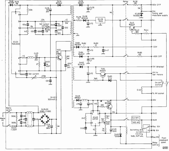
Fig. 1: The power supply - simplified circuit.
