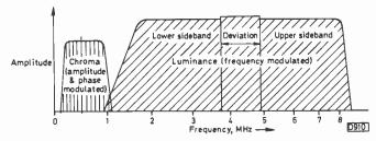
Fig. 3: Typical colour-under VCR recording frequency distribution.
