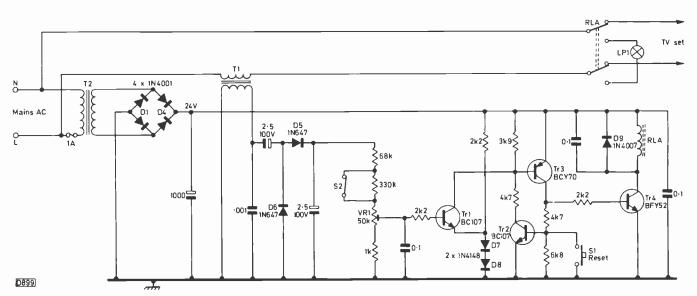
Fig. 1: Circuit diagram of the circuit breaker. Mains transformer T2 has an 18V 1A secondary winding.
