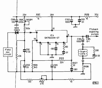
Fig. 3: Field amplifier/output circuit used in early sets.
