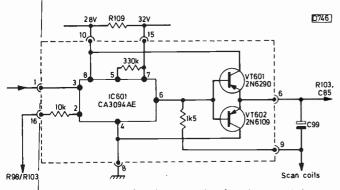
Fig. 5: Final field amplifier/output circuit using module.
