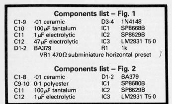
required division by 1,000 is obtained, with a capability well in excess of 1.5GHz. Pin diodes D1-2 (input protection) are optional.
