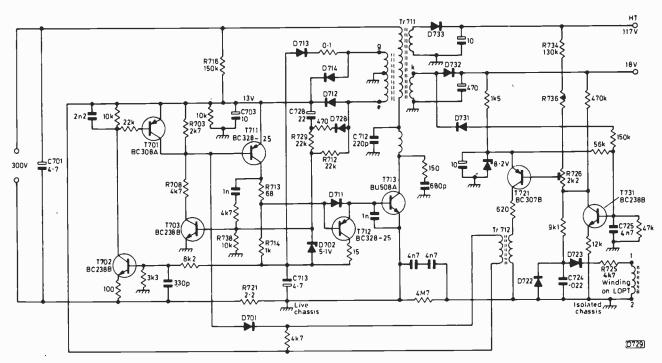
Fig. 1: Simplified circuit of the switch-mode power supply used in the ITT CVC1200 series chassis. The h.t. is 117V in the 90°, 20in. version, 145V in the 110°22/26in. version, the l.t. rails being 18V and 24V respectively. The values of the flyback tuning capacitor C712 and the resistors (R734/R736) feeding the set h.t. control R726 differ in the two versions of the chassis: the values shown above apply to the 90° version.
