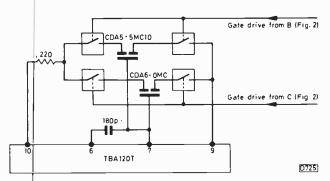
Fig. 3: Use of a second 4066 when ceramic filters are used in the detector circuit.
