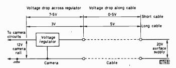
Fig. 1: Constant-voltage supply arrangement.
