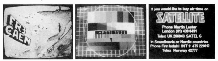
Left: Caen FR3, ch. E28, received by John Tellick during the August enhanced tropospheric conditions. Centre: FuBK test pattern in use by TSI, Switzerland. Courtesy Alexander Wiese. Right: UK Satellite TV caption received on cable in Helsinki via the OTS-2 satellite. Courtesy Petri Pöppönen.
