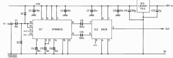
Fig. 2: Circuit diagram, prescaler 3.
