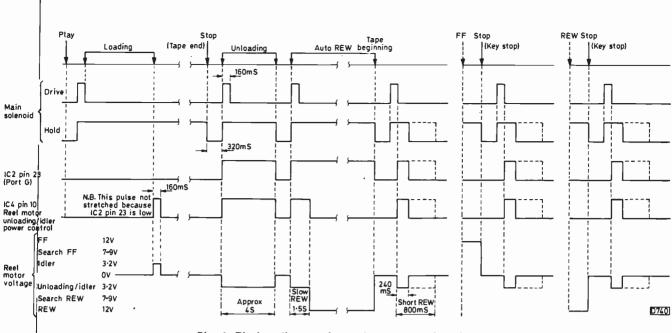
Fig. 4: Timing diagram for various control functions.
