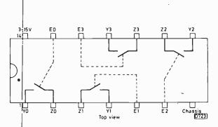
Fig. 1: Pin connections for the 4066 switch i.c. Pins E0-E3 are the control terminals for the four switches.
