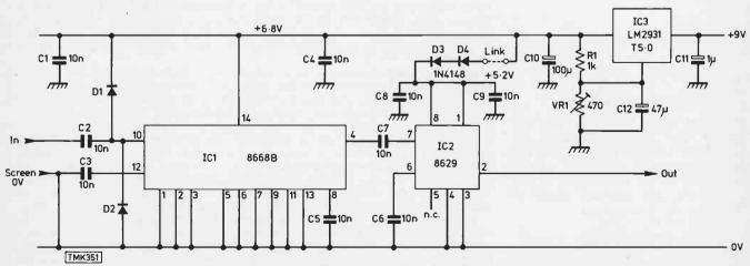
Fig. 1: Circuit diagram, prescaler 2.
