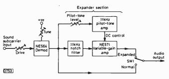
Fig. 7: Block diagram of the sound board.
