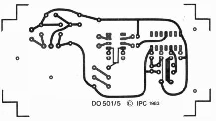
Fig. 3 (above): Prescaler 2 board track pattern (scale 1:1). Fig. 4 (right): Prescaler 2 board pattern, component side.
