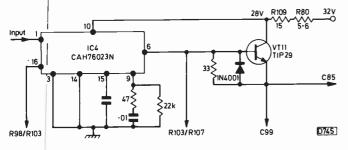
Fig. 4: Modified field output circuit with VT11 added.
