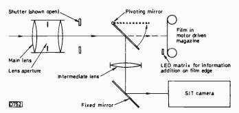
Fig. 5: Simplified diagram of a combined stills and TV camera.
