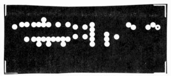
Fig. 6: Prescaler 3 board pattern, component side.
