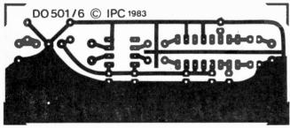
Fig. 5: Prescaler 3 board track pattern (scale 1:1).
