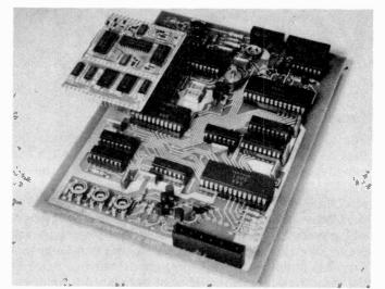
Comparison between a teletext decoder using conventional through-panel component mounting and the equivalent using surface mounting technology.
