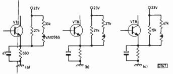
Fig. 6: Field oscillator bias circuit modifications. (a) Early. (b) With circuit shown in Fig. 4. (c) With Fig. 5.
