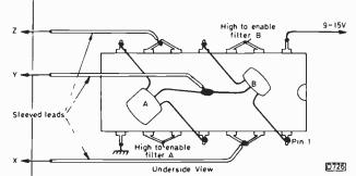
Fig. 4: Solder the filters directly to the pins of the 4066, on its underside. Wires X, Y and Z can then be inserted in the holes used by the original filter – their stiffness will support the assembly above the board. Keep the connecting wires as short as possible.
