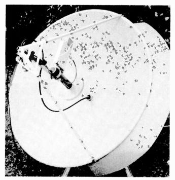
Nick Harold's head unit, with low-noise amplifier, used in conjunction with a 4ft ex-radar dish.
