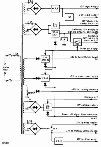
Fig. 67: The 3V23's power supply arrangements.
