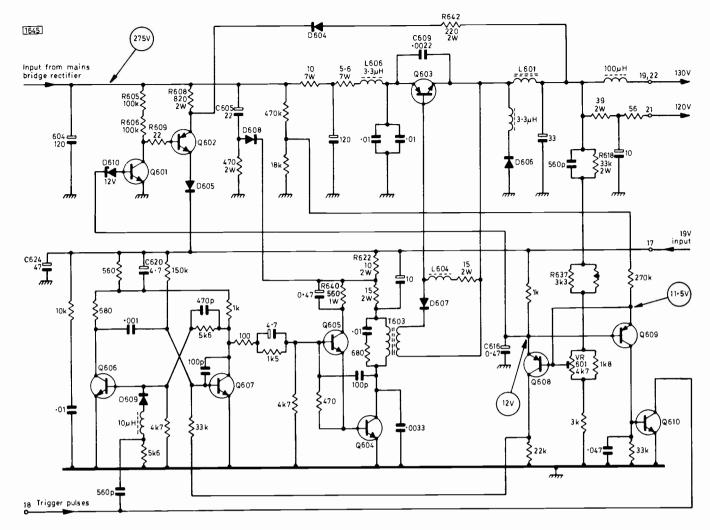
Fig. 2: The chopper circuit used in the Sony Model KV1810UB.
