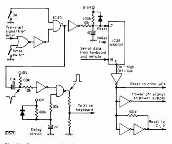
Fig. 72: Power-on switching system.
