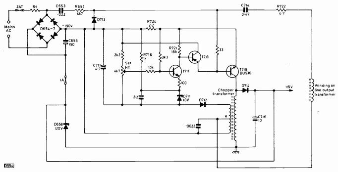
Fig. 4: Chopper power supply circuit (simplified) used in the CVC1100 chassis.
