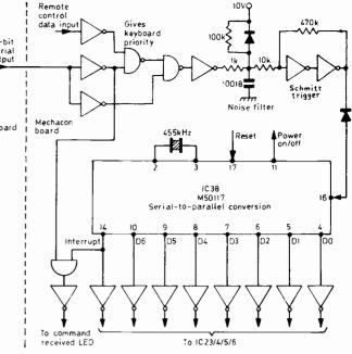
until about five seconds after switch on - it's then necessary to switch "off" then "on" at the front panel. The machine can be switched on and off by remote control provided the front panel switch is at "on", i.e. pin 17 of IC38 is high.
