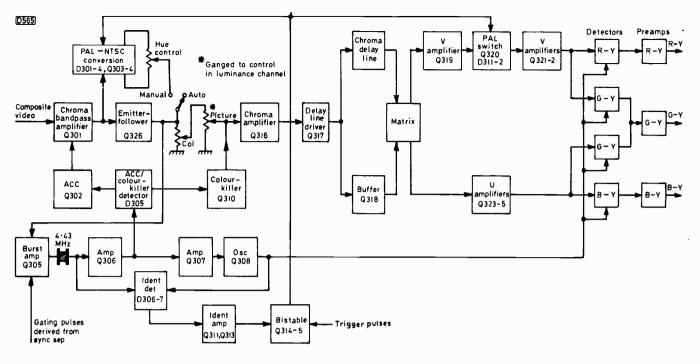
Fig. 4: Block diagram of the KV1810UB's decoder.
