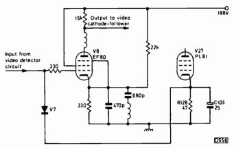
Fig. 3: Video overload diode.
