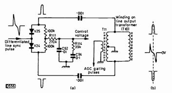
Fig. 1: (a) The flywheel line sync circuit used in the Pye Model V4. (b) Waveforms showing the circuit action.
