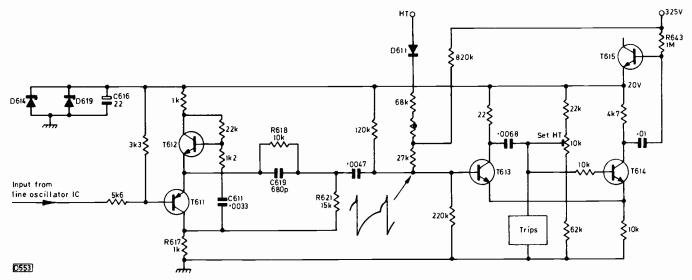
Fig. 3: Chopper control circuitry used in the ITT80 chassis.
