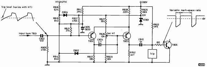
Fig. 2: The pulse-width modulator circuit used in the CVC40/CVC45 series chassis.
