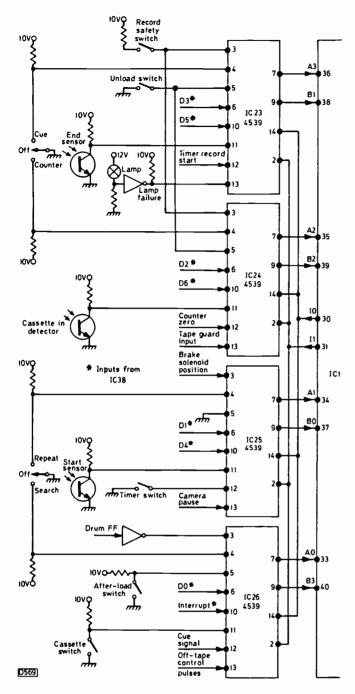
Fig. 70: Data selection arrangement.
