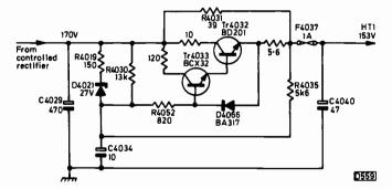
Fig. 1: The h.t. smoothing circuit used in the Philips G11 chassis. C4029 is the h.t. reservoir capacitor. The following circuit consists of an active filter: the potential divider R4030/R4035 with C4034 provide a smoothed bias for the base of Tr4033 which drives the emitter-follower Tr4032.
