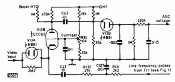
Fig. 2: The vision a.g.c. circuit used in the Pye V4.
