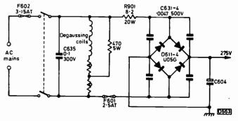
Fig. 1: The mains input circuit.
