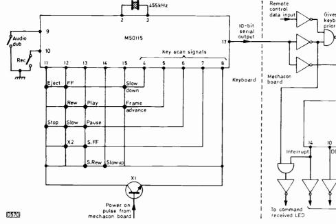
Fig. 71: The user command arrangement.
