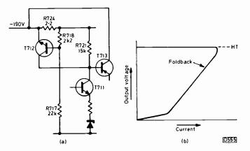
Fig. 5: (a) Excess-current circuit used in the CVC1100 chassis. (b) Foldback voltage characteristic.
