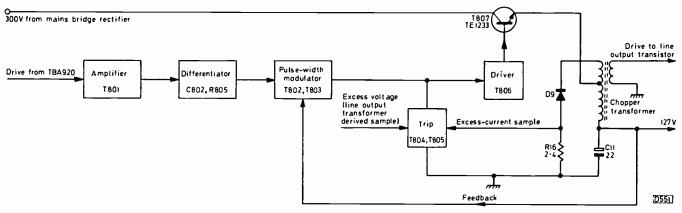
Fig. 1: Block diagram of the chopper power supply used in the CVC40/CVC45 series shassis.
