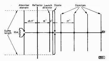
Fig. 1: John Beech's modified Yagi system. The dimensions shown apply to the 144MHz amateur band.
