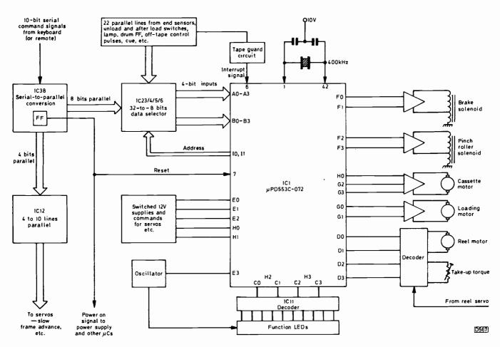
Fig. 68: The microcomputer control system.
