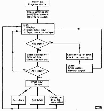
Fig. 4: Flow chart of the TMS1070 microcomputer's programme. The microcomputer starts at the top, then carries out each operation in turn. The whole cycle takes less than  $1 \times 10^{-3}$  seconds.
