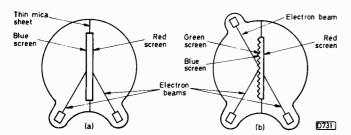
Fig. 2: The basic principles of Baird's Telechrome colour display tube, which he patented in 1940 and demonstrated to the press in 1941. (a) Arrangement of the phosphor coatings for a two-colour version. (b) Use of a riged back to the screen to provide two surfaces for a three-colour system.
