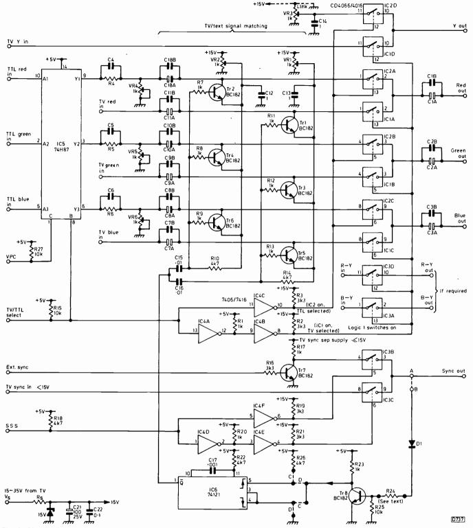
Fig. 1: Circuit diagram of the TV-VDU interface unit. The value of Rs in ohms is given by  $(Vs - 15V)/(20 \times 10^{-3})$ . SSS is the sync source select line and VPC the video polarity control line. Input to the monostable IC6: link C with negative-going pulses, link D with positive-going pulses. Link A-B if the set's sync pulses are less than 15V: if the sync pulses are greater than 15V, insert the sync feed at B. Reverse the polarity of D1 for negative-going input pulses.
