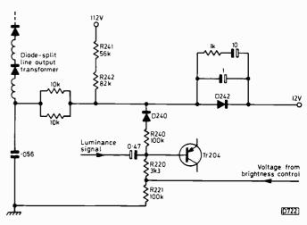
Fig. 5: Circuit used in the Rank-Toshiba T24E chassis.
