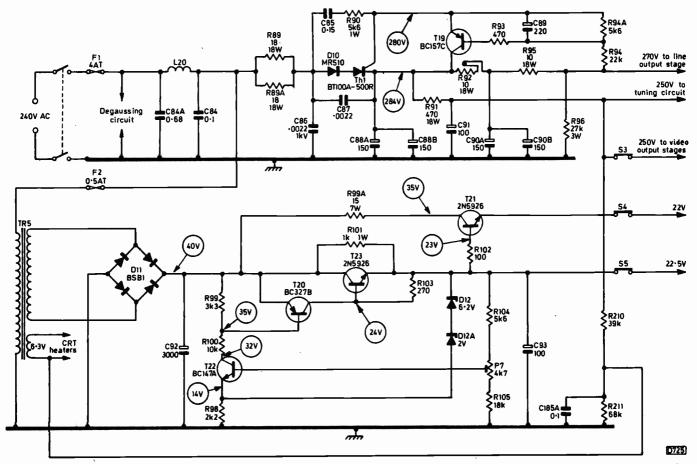
Fig. 5: The power supply circuitry used in the Zanussi Model BR1026. 270V and 250V h.t. supplies are derived from the mains by half-wave rectification, thyristor Th1 acting as an over-current trip. The 270V line supplies the line timebase, the 250V line supplying the luminance output transistor (T16, BF338) and the three colour-difference output transistors (T35/6/7, type SE7056). Series regulators stabilise the 22V and 22·5V l.t. supplies.
