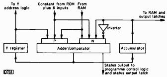
Fig. 5: The arithmetic logic unit's inputs and outputs.
