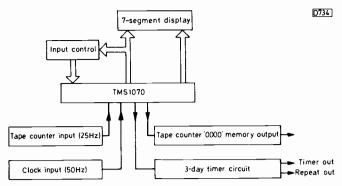
Fig. 6: Use of the TMS1070 in the Sanyo VTC9300P VCR.
