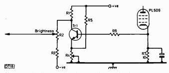
Fig. 1: Typical hybrid chassis beam limiter circuit.
