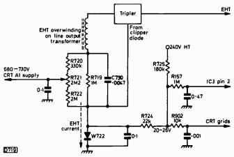
Fig. 2: Beam limiting in the Thorn 9000 chassis.
