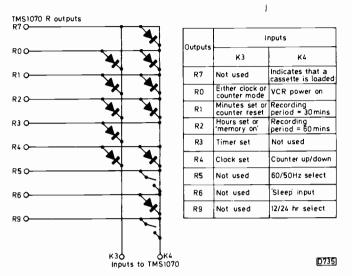
Fig. 7: Arrangement of the input control system.
