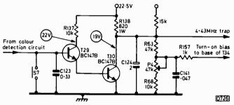
Fig. 2: The two-stage switch which provides the colour-killer action. In the absence of a colour signal, the two transistors are biased into conduction, the voltage at the junction of R138/R63 thus being reduced. To override the colour-killer, add link S 7 to remove the bias from the base of T29. With a colour signal present and the reference oscillator locked to the burst, the synchronous colour-killer detector D16/17 provides a negative-going output to switch T29/30 off.
