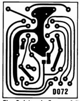
Fig. 3 (above): Copper foil diagram of DO72. Fig. 4 (right): shows the component locations.
