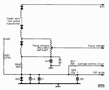
Fig. 3: System used in the Beovision 3502 chassis.
