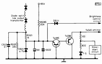
Fig. 7: The circuit used in the Pye/Philips G11 chassis has two modes of operation (see text).
