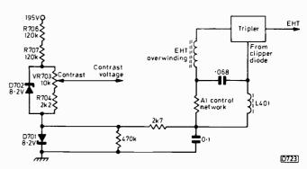
Fig. 6: Use of a zener diode for beam sensing in the Decca 70 series chassis.
