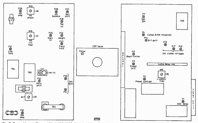
Fig. 3: Control layout, Zanussi Model BR1026. Boards viewed from the front (component side).
