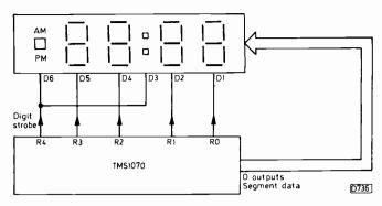
Fig. 8: Driving the fluorescent display.
