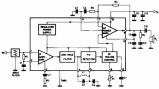
Fig. 1: Functional block diagram of the TDA1190Z with peripheral components.
