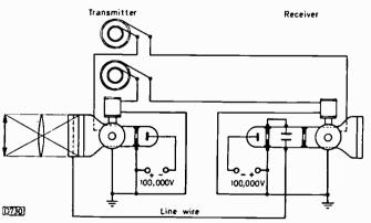
Fig. 1: A. A. Campbell Swinton's 1912 scheme for an electronic TV system. The main problem was that a camera "plate" to convert the picture into an electronic signal was not at the time available – the development of an effective camera tube was in fact the key to modern television.
