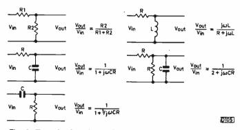
Fig. 9: Transfer functions of common circuits.
