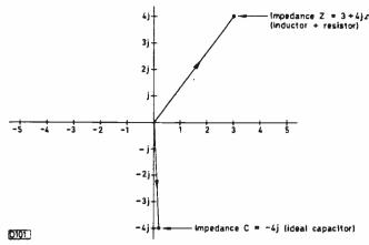
Fig. 5: Impedance diagram for a real inductor and an ideal capacitor.
