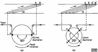
Fig. 3: VHS and VHS-C compared, (a) VHS with 62mm drum, (b) VHS-C with 41mm drum.
