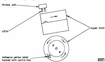
Fig. 3: Method of using the video head position checker. Use with low background light.
