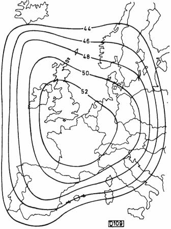
Fig. 1: Approximate service area of Astra's channels 4, 8, 12 and 16, which have been allocated to Eurosport, Sky Channel, Sky News and Sky Movies respectively. Polarisation is nominally vertical. Figures represent e.i.r.p. in dBW. Centre frequencies are as follows: channel 4 11·2585GHz, channel 8 11·3175GHz, channel 12 11·3765GHz and channel 16 11·4355GHz. The f.m. video deviation is 16MHz/V.
