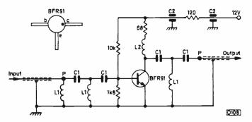
Fig. 2: Circuit of the u.h.f. amplifier to boost the output from the HS D100 converter.  $C1 = 5.6 \mathrm{pF}$  sub-miniature ceramic;  $C2 = 1 \mathrm{kpF}$  feedthrough;  $P = \mathrm{stand}$ -off insulator, RS type 433-876; resistors should be low-noise types, 0.25 or 0.2W;  $L1 = 2 \mathrm{V4}$  turns,  $\mathrm{Vein}$ . diameter close-spaced; L2 = 2 turns  $\mathrm{Vein}$ . diameter wound on from the leadout wire of the series  $68\Omega$  resistor.
