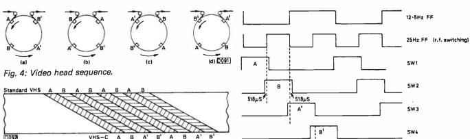
Fig. 5: How the tape is scanned in the VHS and VHS-C systems, showing how compatibility is achieved. Tape viewed from the head side.
