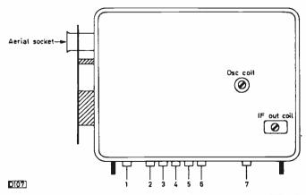
Fig. 1: Physical appearance of the NSF type 240-039-ET001 tuner. Pin connections are as follows: 1 Band I 12V; 2 tuning 0-28V; 3 u.h.f. 12V; 4 12V supply; 5 0-8V a.g.c.; 6 Band III; 7 i.f. output. Details from Bill Cotterill.
