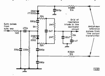
Fig. 3: Flywheel line sync circuit used in the ITT CVC5 and related chassis.
