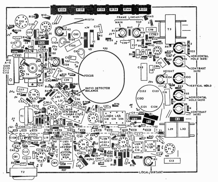
Fig. 2: Main chassis component layout.
