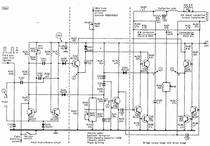
Fig. 1: Complete field timebase circuit. Following the sawtooth waveform charging circuit, the phase-splitter transistor T454 provides antiphase outputs to the driver transistors T456 and T457 which in turn drive, in push-pull, the bridge output transistors T458/T459/T461/T462. To assist with the flyback, a pulse obtained from the collector of T452 is applied via D456 to the impulse adder emitter-follower transistor T453 and is fed via C457 to the output stage.
