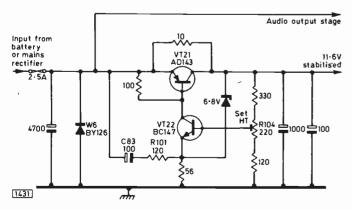
Fig. 2: L.T. stabiliser circuit used in the Thorn 1590, 1591 and 1593 chassis. W6 provides protection against reverse battery connection. C83/R101 provide hum cancellation.
