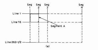
Fig. 2: (a) The Sampledot pseudo-random sampling matrix. (b) An expanded view of segment A, showing a typical pseudorandom sampling code sequence.
