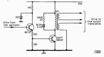
Fig. 5: Typical transistor line driver stage – as used in the Rank A823 chassis.
