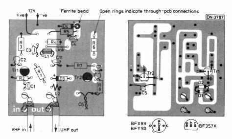
Fig. 3. Component location diagram. Note that some components are mounted on the reverse side of the board. Although other transistors may be used, the preferred type is BF357K.
