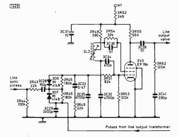
Fig. 2: Line oscillator circuit used in the A774 chassis.
