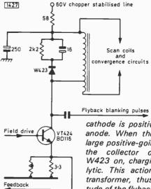
Fig. 1: Field output stage circuit used in the Thorn 3000 and 3500 chassis. W423 and its associated RC network provide flvback pulse limiting to protect the output transistor. During the forward scan W423 nonis conducting since its
