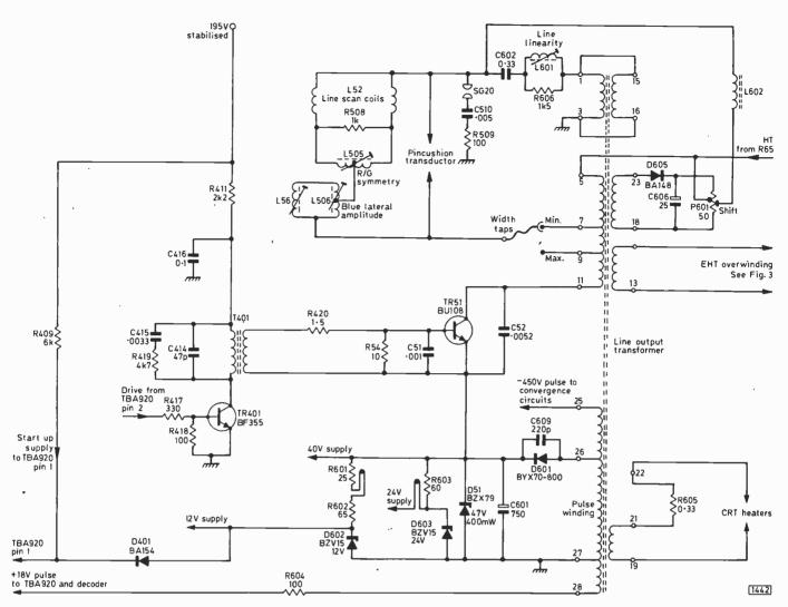
Fig. 2: Circuit of the line output stage. The 47V zener diode D51, a 400mW type, provides circuit protection. Should the 40V line, which is obtained by scan rectification (D601), rise above 47V the zener will go short-circuit, thus removing the l.t. supplies and shutting down the line output stage since there is no line drive.
