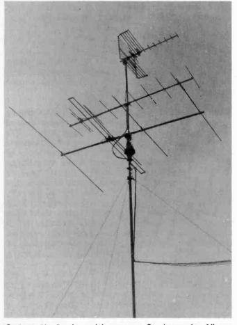
Graham Harrison's aerial mast at St. Leonards. All are wideband arrays: backfire for u.h.f., 10-element for Band III (Telerection), 4-element home constructed unit for Band I.
