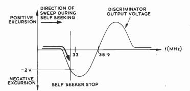
Fig. 2: Response curve of the a.f.c. circuit in the self-seeking tuning system devised by Grundig. The self-seeking action stops as soon as the discriminator voltage sinks to -2V.
