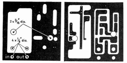
Fig. 2. Printed circuit board details. It is imperative to follow the artwork given very closely, as this will determine the characteristics of the tuning line. For those wishing to buy a ready made board, these are available from Clearline (Bampton), Brook Street, Bampton, Devon, at £1.30 including VAT and postage and packing.
