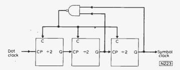
Fig. 45(a): Divide by six counter for symbol clock divider.
