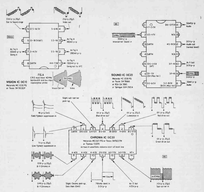
Fig. 9: Voltages and waveforms associated with the three i.c.s. Courtesy Thorn Consumer Electronics.
