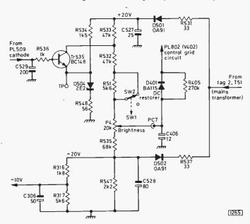
Fig. 2: The brightness control, luminance d.c. restorer, and beam limiter circuitry. Diode D501 was shown the wrong way round in the September issue.
