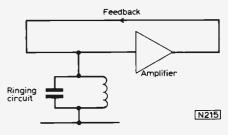
Fig. 7: General circuit of an oscillator as a ringing circuit plus an amplifier with positive feedback. The ringing element can be a series LC circuit, a quartz crystal or an RC circuit.
