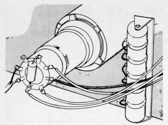
Fig. 2: Tube base leads caught around the mains dropper: make sure that all wiring is routed clear of power resistors and sources of high pulse voltages.
