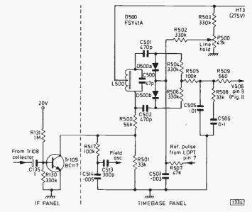
Fig. 3: The sync separator and flywheel line sync circuitry.
