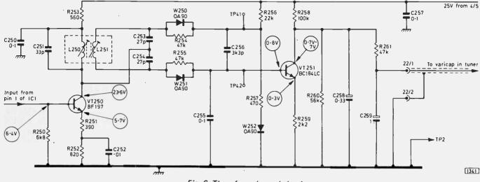
Fig. 6: The a.f.c. subpanel circuit.
