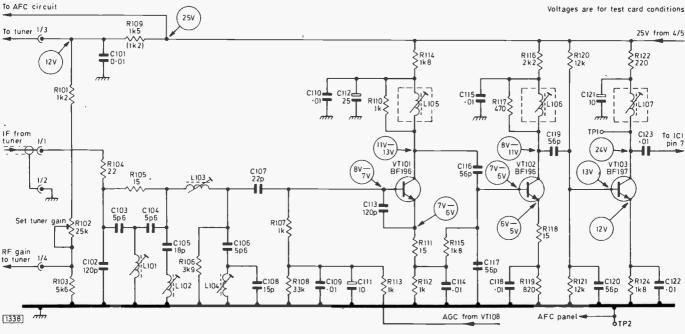
Fig. 2: Circuit of the i.f. amplifier.
