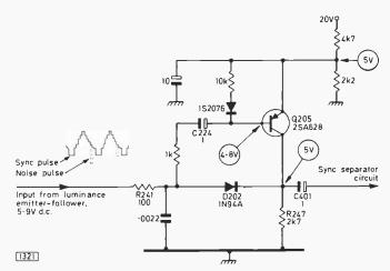
Fig. 2: Simple amplitude-discriminating circuit used in the Mitsubishi Model CP140B. Q205 conducts in the presence of noise, reverse biasing D202.
