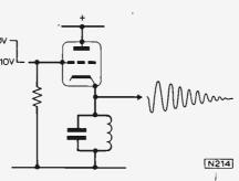
Fig. 6: A simple ringing circuit. Note how the amplitude of the oscillations decreases.
