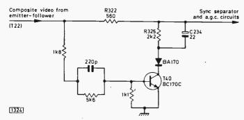
Fig. 5: This circuit was used in early versions of the ITT CVC5 chassis to remove noise from the feeds to both the sync separator and the a.g.c. circuits.
