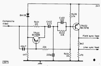
Fig. 8: Noise-cancelling circuit used in the Indesit Model T24EGB. TR401 acts as a clamp when driven into conduction by noise pulses.
