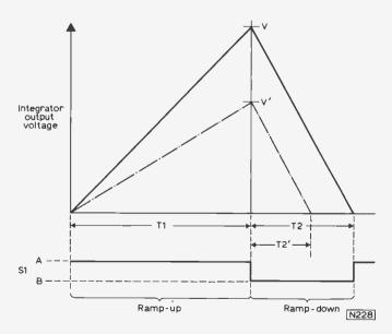
Fig. 2: The dual-ramp integrator cycle. Capacitor C charges to V volts from the input voltage during T1, and is discharged at a constant rate during T2. T2 is thus proportional to V. The broken line represents integrator output with a lower voltage input V'. Note that the angle of the ramp-down slope is constant.
