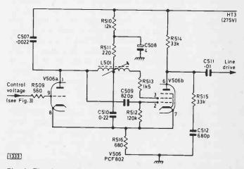
Fig. 1: The line oscillator circuit. The line output stage circuit was shown in Fig. 2, page 518 of the September issue.
