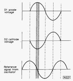
Fig. 13: Waveforms of the circuit of Fig. 12. The reference oscillator runs 90° out of phase with the incoming bursts.
