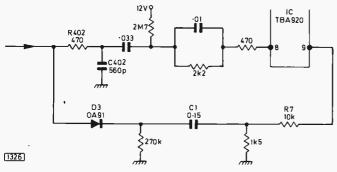
Fig. 7: In the Grundig 5010/6010 series the noise gate in the TBA920 is used to remove the effect of noise on the sync separator.
