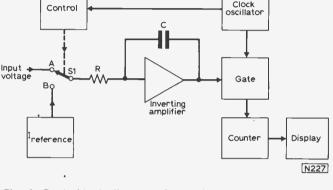
Fig. 1: Basic block diagram of a dual-ramp d.v.m. The clock oscillator is an accurate source of timing pulses, and S1 is an electronic switch, i.e. a transistor junction. The I reference is derived from a stable zener diode.
