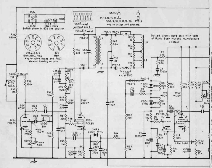
Fig. 1: Circuit of the power supplies and timebases, Bush TV161 series. Voltages marked with an asterisk apply to 625-line of
