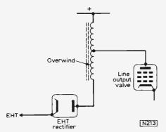
Fig. 5: Basic principle of e.h.t. generation by the line output stage.
