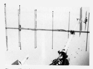
The modified wideband Telerection Band III array.
