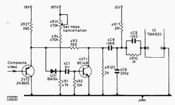
Fig. 6: Noise-cancelling circuit used in conjunction with a TBA920 sync separator/line oscillator i.c. in the Rank Z179 110° colour chassis.
