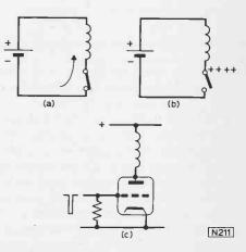
Fig. 3: When an inductive circuit is broken, a high voltage is induced in the inductor.
