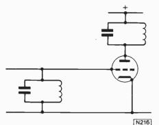
Fig. 8: How can this circuit oscillate?
