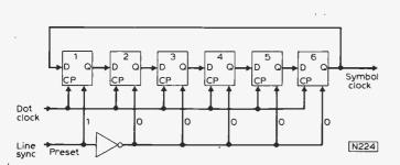
Fig. 45(b): A symbol clock divider using a shift register.
