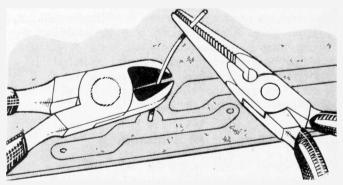
Fig. 1: When cropping excess wire from a joint on a printed panel, hold the free end to prevent it falling down into the chassis where it may cause a short-circuit.
