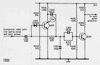
Fig. 3: Circuit used in the Toshiba Model C81B. Q307 conducts in the presence of noise, producing a negative output pulse to cancel the noise pulse in the feed to Q301.
