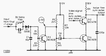
Fig. 1: This circuit, used in 90° B and O colour sets, distinguishes noise by its wider bandwidth. In the presence of noise, D1 and Tr3 conduct, ensuring that Tr2 and Tr4 remain cut off.
