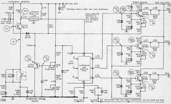
Fig. 4: The luminance, RGB output and brightness circuits.
