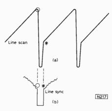
Fig. 9: Relative timing of line scan and line synchronising pulses.
