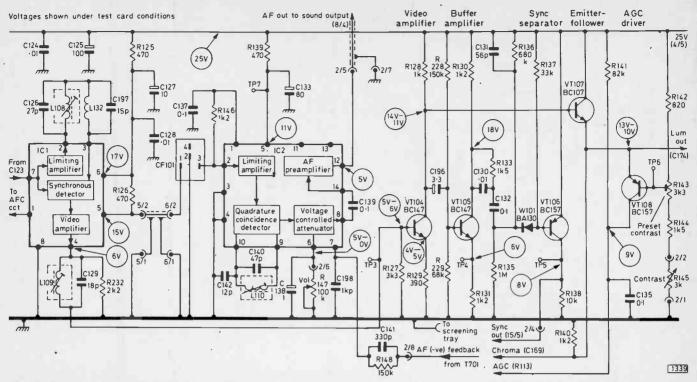
Fig. 3: The video detector (IC1), intercarrier sound (IC2), sync separator and a.g.c. circuits. Negative feedback from the secondary of the sound output transformer T701 is fed to pin 7 of IC2 via R148/C141: the tap on T701 was omitted in Fig. 3 last month.
