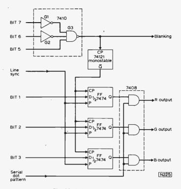
Fig. 46: Colour decoding logic.
