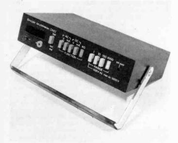
This is one of the least expensive DVMs on the market, yet it has most of the facilities and specifications of its more pricey counterparts. Function and range selection are by push-buttons. The case is extremely rugged, being made of cast aluminium. The power source is an internal PP9.
