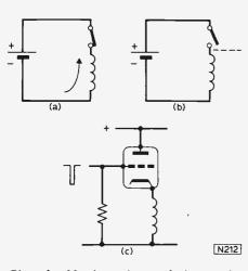
Fig. 4: Moving the switch to the opposite end of the inductor does not alter the circuit action, only the polarity of the induced voltage. This will always be opposite to the voltage that was applied.
