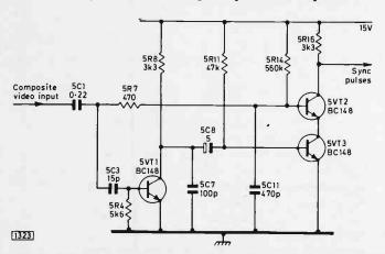
Fig. 4: This circuit, used in the Rank Z504 scan drive panel, discriminates between noise and the sync pulses by the higher amplitude and greater bandwidth of the former, 5C3 and 5R4 forming a high-pass filter.
