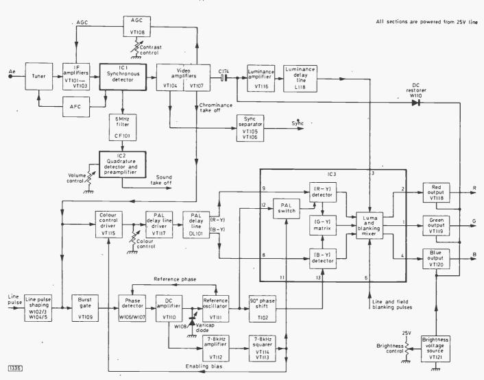
Fig. 1: Block diagram of the i.f./decoder/RGB output panel.
