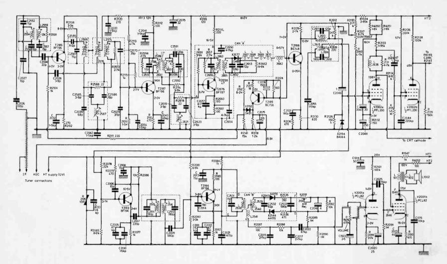
Fig. 3: Circuit of the i.t. strip, sound and video output stages and sync separator, Philips 300 chassis.
