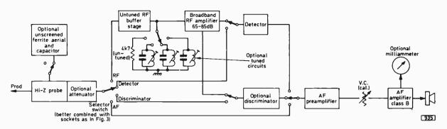
Fig. 1: Signal tracer block diagram, showing optional features that can be incorporated to increase the instrument's usefulness. The untuned r.f. buffer stage would be needed only to isolate the optional tuned circuits from the optional attenuator.
