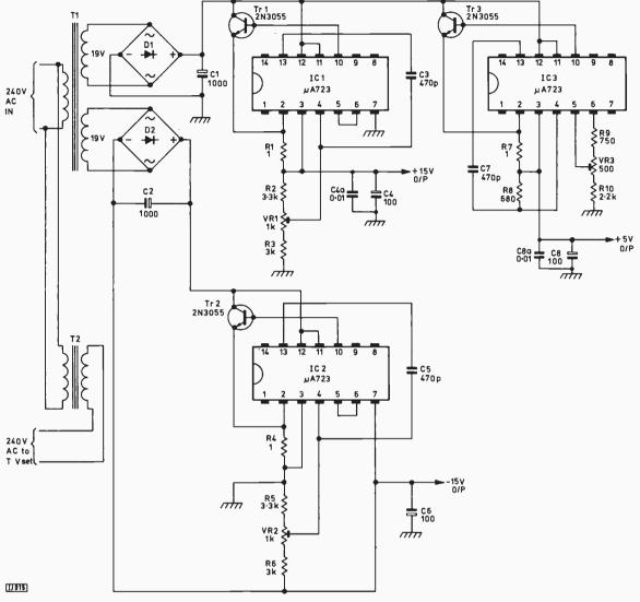
Fig. 2: Circuit of the power supply unit.
