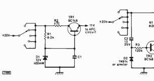
*Fig. 1: Basic slow run-up regulator circuit adopted to provide electronic a.f.c. muting.*
