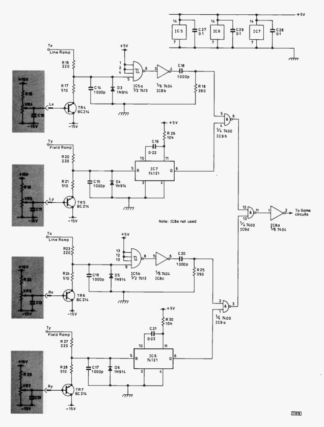
Fig. 5: Circuit of the left and right man control systems. The shaded circuitry is contained in the joy-stick controls to be described in Part 2.
