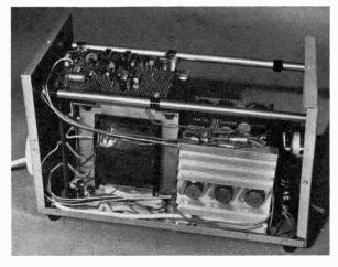
Fig. 3(a): This view of the prototype control unit during construction shows on the left the isolation transformer with the ramp generator board (to be described in Part 2) above it and on the right the power supply regulator board with its associated series stabiliser transistors. The mains transformer is beneath the regulator board.
