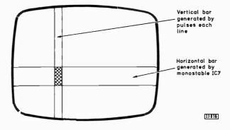
Fig. 6: How a man is produced on the TV screen.
