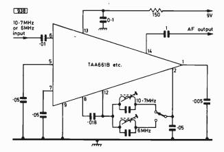
Fig. 4: Use of a coincidence (quadrature) f.m. discriminator integrated circuit.
