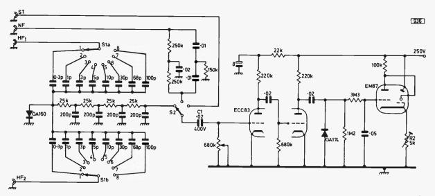
Fig. 2: Circuit (slightly modified) of the Telefunken design for a signal tracer and frequency comparator. Note that networks of capacitors like those at SIa and SIb could also be used at the ST and NF inputs—without the OA160 and  $25k \Omega/200pF$  filter.
