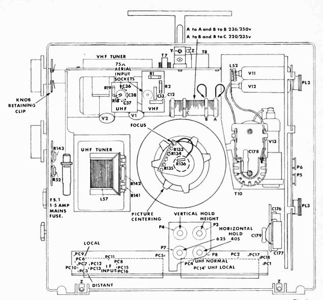
Fig. 4: Rear view of the receiver with the cabinet back removed. Screw Y and distance piece secure the handle. The three screws Z secure the chassis to the cabinet.
