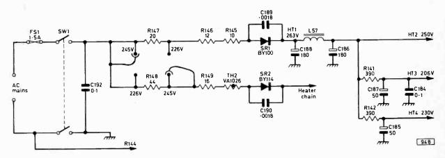
Fig. 5: Power supply circuit. H.T. voltages apply on 625 lines—they are slightly higher on 405 lines.
