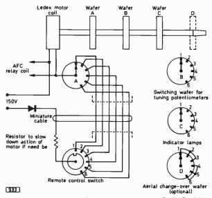
Fig. 1: Remote control system suggested by B. D. Dodd.
