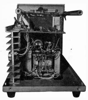
Fig. 3(b): View of the prototype control unit with the front panel removed to show the mains transformer, rectifiers and reservoir capacitors mounted under the regulator circuit board.
