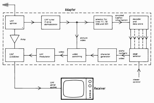
Fig. 1: Block diagram of a Ceefax adapter unit, courtesy BBC.
