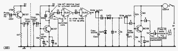
Fig. 3: A.M. signal tracer, All sections of the circuit except the class B audio module and the loudspeaker should be screened. The SL612 requires 6V at pin 2: pins 4 and 8 should be earthed and there is no connection to pin 1.
