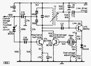
Fig. 4: Line generator circuit used in earlier versions of the RBM 90' single-standard colour chassis. The capacitance of varicap diode D4 is varied by the output from the flywheel sync discriminator circuit. Since D4 is connected in the capacitive feedback loop between the collector and base circuits of VT4 this adjusts the degree of reactive feedback. In effect VT4 acts as a reactance multiplier,
