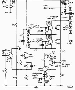
Fig. 3: Line output circuit used in later versions of the Philips G8 chassis, with two-transistor beam limiter circuit. (BY14 scan unit.)
