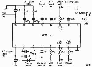
Fig. 5: Use of a phase-lock-loop discriminator/detector i.c. The signal inputs must be via capacitors. The f.m. input pins 12 and 13 feed a balanced circuit: if an unbalanced input is used earth one pin via the capacitor.
