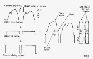
Fig. 1: Showing the make up of two successive lines of the composite camera output waveform (not to scale).
