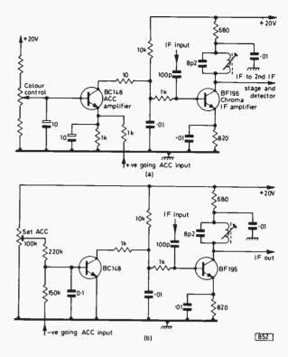
Fig. 4: (a) The original a.c.c. circuit on the RBM i.f. board. (b) Modified a.c.c. circuit to suit the input from the Mullard type decoder.
