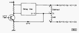
Fig. 4: Typical practical chroma delay line circuit.
