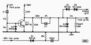
Fig. 12: Blanking and beam limiting circuits.
