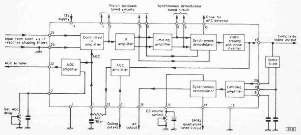
Fig. 1: Block diagram of the SL437F i.c., which provides a complete TV i.f. system.
