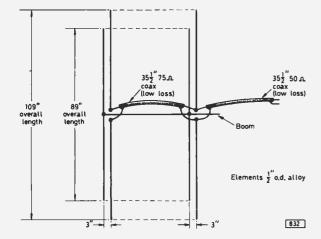
Fig. 1: Exploded view of the improved Band I omnidirectional array. The dipole assemblies are mounted at right angles to each other—see accompanying photograph.
