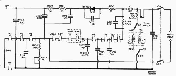
Fig. 2: Power supply circuit with capacitive (C121) heater dropper (early 960 chassis).
