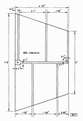
Fig. 3: The printed circuit board pattern. Two boards are required, mounted as shown in Fig. 1. Dimensions given are for a group CD aerial: for group B multiply all dimensions by 1.2 and for group A by 1.5. The width of the conducting strips is 0.1 in. Shown half scale.
