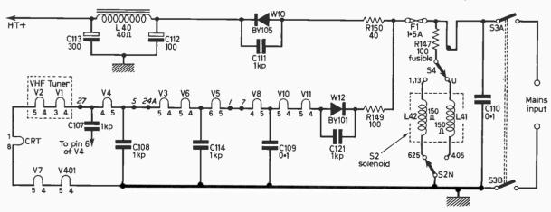
Fig. 3: Power supply circuit used in later versions of the 960 chassis.
