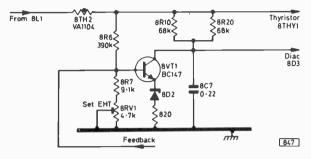
Fig. 2: Modifications introduced in the stabilised power supply circuit used in later versions of the RBM 90° single-standard chassis.
