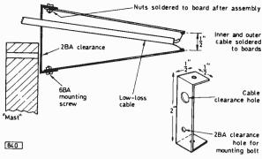
Fig. 1: Cross-section of the assembled aerial, showing the taper. The separation between the insides of the two printed boards at the front is ½in.
