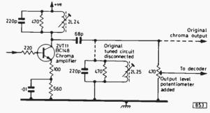
Fig. 5: Modification to the chroma amplifier on the RBM board to make it suitable for feeding the Mullard type decoder circuit.
