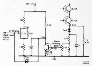
Fig. 1: The beam limiter circuit used in the Philips G8 colour chassis.
