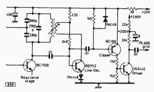
Fig. 11: Modification to the RBM line drive circuit to enable it to drive a valve line output stage.
