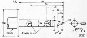
Fig. 3: The jointed test finger-courtesy of the British Standards Institution. Dimensions in mm.
