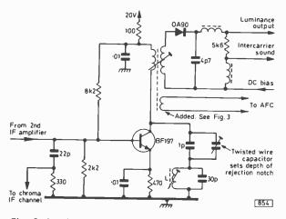
Fig. 6: Luminance i.f. output stage. The rejector L was redeployed as a chroma rejector to delete sound-chroma beat patterning.
