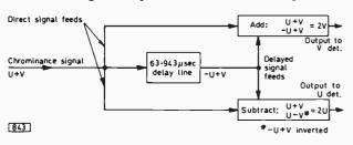
Fig. 2: How the chrominance delay line and its associated add and subtract networks in a PAL decoder separate the two transmitted colour-difference signals prior to demodulation.
