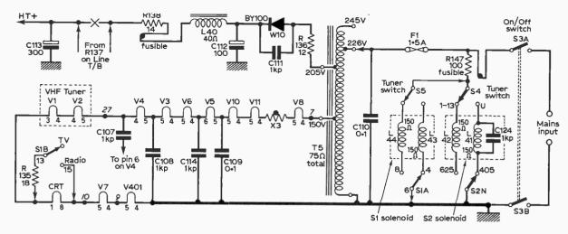
Fig. 1: The power supply circuit used in the basic 950 chassis.
