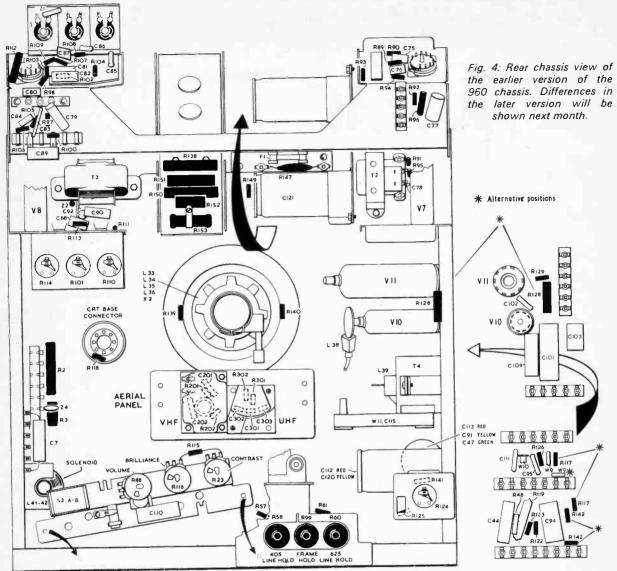
thermistor. Note that whereas the output from h.t. rectifier W10 is positive that from the heater rectifier W12 is negative. The surge limiting resistors for the two rectifiers, R149 and R150, are wound on a substantial ceramic former mounted at the top centre of the chassis along with the fusible resistor R147.
