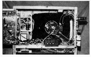
Rear view of B. C. James's version of the "Television" Colour Receiver. The decoder and timebase panels are mounted on hinges at the left- and right-hand sides respectively. The i.f. strip is mounted on the left-hand side panel. The mains transformer is on the left, with the power circuit board above. The RGB drive controls are beneath the c.r.t. base panel, with the RGB board behind.
