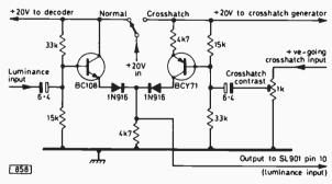
Fig. 10: Crosshatch input and switching circuit.
