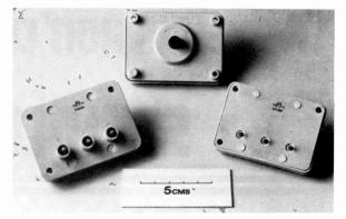
Fig. 2: High-voltage thick-film focus modules for use in colour TV sets. The circuit provides automatics focus voltage correction for wide variations in mains voltage. Courtesy Welwyn Electric Ltd.
