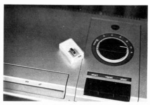
This exclusive "Television" photograph shows a close-up view of the TED player with the pick-up cartridge in its box on top.
