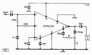
Fig. 4: Typical peripheral circuitry for the Texas SN76013N audio output i.c.
