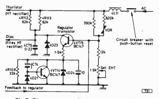
Fig. 2: Slow-start system in the power supply circuit.
