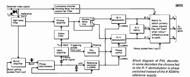
(a). It establishes the correct operating phase for the PAL bistable. This is a multivibrator which is clocked (reversed) by line pulses to run at half line frequency and operates a phase reversing switch in the reference oscillation supply to the R-Y demodulator. This arrangement is necessary because the R-Y phase is reversed at the transmitter on successive lines; without 'ident' the PAL bistable cannot 'know' in which of its two phases to start.
