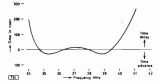
Fig. 5: A group delay curve for a complete i.f. strip.
