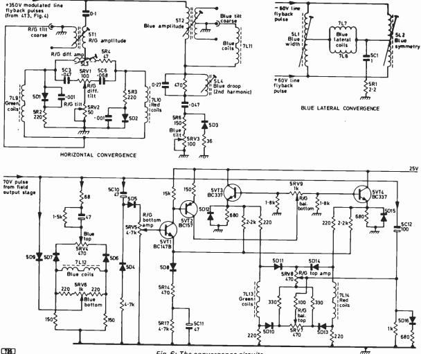
Fig. 6: The convergence circuits.
