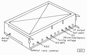
Fig. 1: ELC1043 u.h.f. tuner pin connections.
