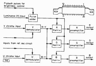
Fig. 1: Block diagram of the SL901 chrominance demodulator and matrixing i.c. used in Bush/Murphy models.
