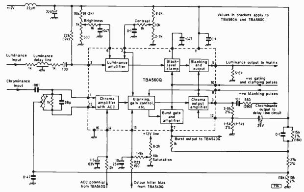
Fig. 3: Block diagram together with peripheral circuitry for the TBA560 series of chrominance i.c.s.
