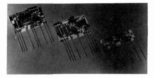
Fig. 1: Thick-film hybrid circuits for use in colour TV receivers. Courtesy Erie Electronics Ltd.
