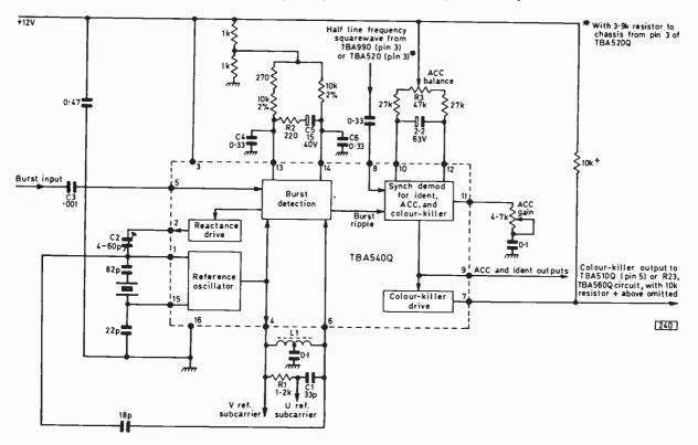
Fig. 2: Block diagram together with peripheral circuitry for the TBA540 decoder reference oscillator i.c.
