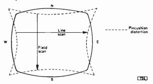
Fig. 5: Illustrating the pincushion distortion correction required.
