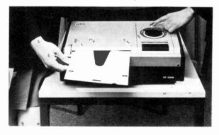
The Telefunken TP1005 "TED" videodisc player. The 21cm. disc in its sleeve is inserted in the slot at the front of the player. The only controls required for operation are the start, stop and repeat buttons.
