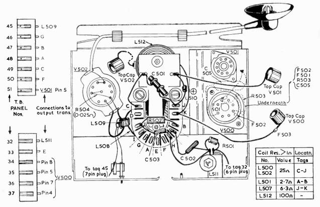
Fig. 3: Physical layout of the line output stage. When replacing the line output transformer clear the tags then unsolder the heater wires from V502 holder, accessible after prising out the top moulding. Coil d.c. resistances given where greater than  $1\Omega$ .
