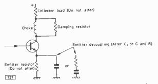
Fig. 8: The response of a video output stage can be modified by altering the damping of the peaking coil or the emitter decoupling.
