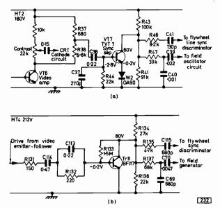
Fig. 4: Representative sync separator circuits used by UK setmakers, both with a single npn transistor. (a) From the BRC 1580 chassis. (b) From the ITT-KB VC200 chassis. The network C113, R132 in (b) is included to provide noise suppression so that the sync separator transistor is triggered on by a clean sync pulse.
