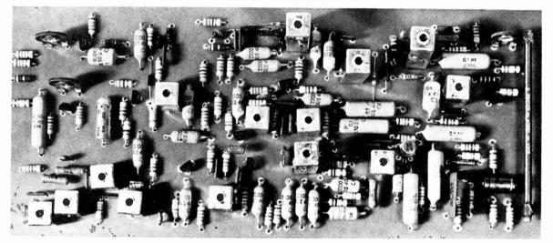
THE i.f. module in our colour receiver contains not only the i.f. amplifier and its associated chroma/ sound and luminance detectors but also the sound intercarrier amplifier and f.m. detector, the a.f.c. detector, the a.g.c. circuits for i.f. amplifier and tuner gain control, the controlled chroma amplifier stage, and the luminance delay line circuit and output phase splitter.
