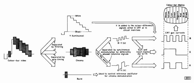
Fig. 2: Simplified representation of the processes in which the composite video signal is decoded to give a colour display. Factors glossed over here include the use of a delay line for initial U and V signal separation and the coefficients in the basic colour equations.
