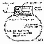
set's own demagnetising coil to cope. A small area can sometimes be cleared of magnetism by holding an "instant heat" mains solder gun close as these produce a strong a.c. field. It is however so simple to make up a demagnetising coil that there is no excuse for doing without one. Incidentally it is often called a "degaussing" coil which is rather a misleading name.
