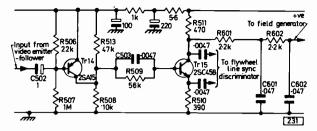
Fig. 3: The two-stage pnp-npn transistor sync separator circuit used in Hitachi mains/battery portables.
