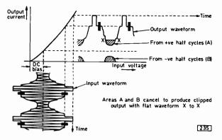
Fig. 3: This shows why applying d.c. bias to a common luminance/chrominance detector diode will not give a linear detection characteristic.
