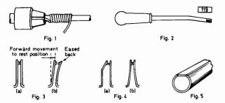
Fig. 1: Using a wheelbrace to wind a spring. The end is anchored securely in the chuck and the wire kept taught and pulled backwards to ensure close turns.
