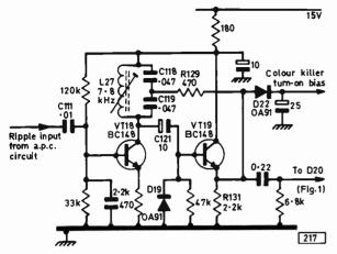
Fig. 2: The V switching must be synchronised and for this purpose the ident circuit shown here (Pye 691 chassis) generates a 7-8kHz sinewave from the phase swings of the transmitted burst signal.
