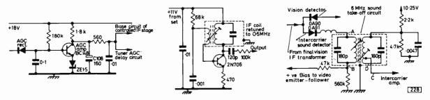
Fig. 1 (left): The a.g.c. circuit used in the GEC-Sobell 2048-1048 series. Fig. 2 (centre): The 0.5MHz oscillator circuit suggested by Ronald Exeter for the reception of CCIR sound signals. Fig. 3 (right): Philips T-Vette sound take-off circuitry to which the 0.5MHz signals were applied.
