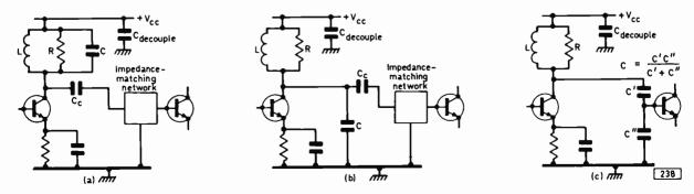
Fig. 6: Impedance matching by using tapped tuned circuit capacitance (d.c. biasing arrangements not shown).
