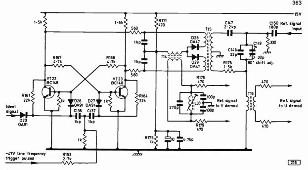
Fig. 1: Typical PAL V switch circuit (T15 with D28 and D29) and its controlling bistable circuit (VT22 and VT23) which provides antiphase squarewave outputs to switch the diodes D28 and D29 alternately on and off. In this circuit (Pye 691 chassis) it is the reference signal to the V demodulator that is switched line by line.
