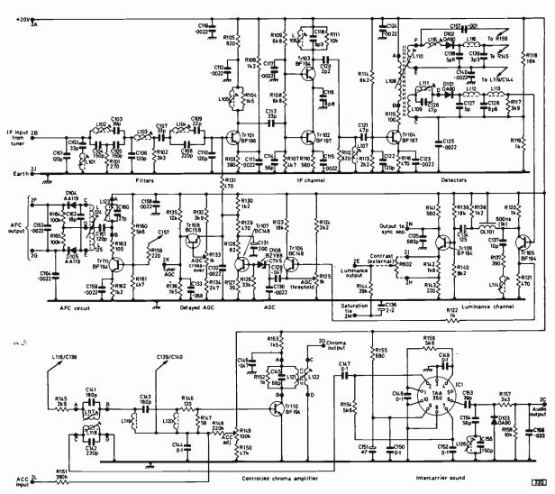
Fig. 7: Complete circuit diagram of the i.f. strip for the Television colour receiver. The strip incorporates the luminance channel, the a.g.c. circuits, the a.f.c. circuit, the intercarrier sound channel and the first chrominance amplifier. C138 may be 5pF.
