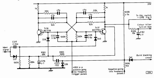
Fig. 4: The bistable circuit used in the ITT-KB chassis also provides the colour killer turn-on bias to bring the chrominance channel into conduction on a colour signal.
