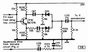
Fig. 3: The PAL V switch used in the ITT-KB CVC5 chassis uses a pair of switching diodes (D25 and D26) in conjunction with a transistor phase splitter (Tr30). In this chassis it is the signal feed to the V demodulator that is inverted on alternate lines.
