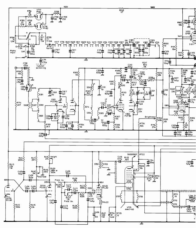
Fig. 3: Circuit diagram, Philips Model 19TG108U. Voltages shown measured using a 20,000  $\Omega$ /V meter.
