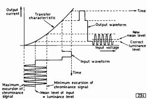
Fig. 2: With a common luminance and chrominance signal detector the non-linear transfer characteristic of the diode produces the form of distortion shown here.
