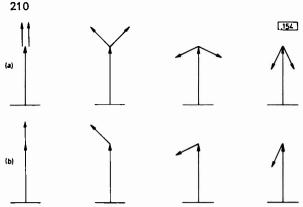
Fig. 6: A double-sideband signal (a) and a single-sideband signal (b) with the lower sideband removed.
