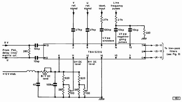
Fig. 5: External connections to the TBA520Q i.c. as used in the Philips G8 chassis.
