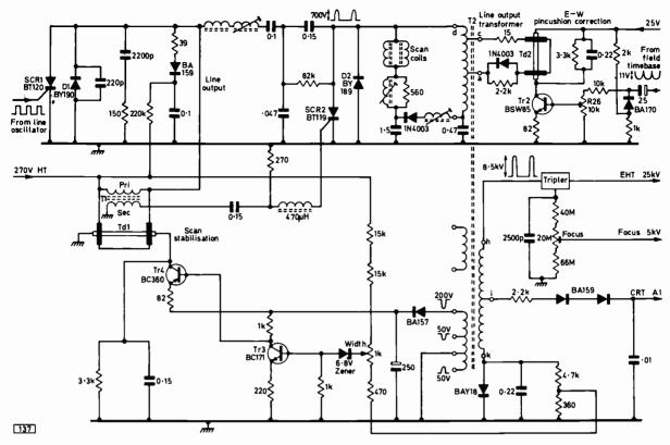
Fig. 3: Complete ITT 110° thyristor line output stage for colour receivers.
