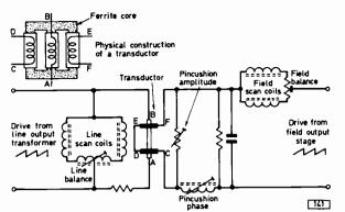
Fig. 6: Simplified 90° pincushion correction circuit.
