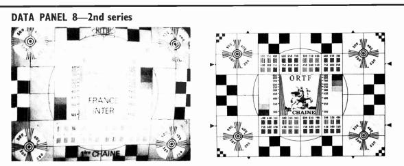
**France:** The test card for both chains is similar, with an identification below the circle to indicate the chain. At present the test card above left is used by both chains though at times the alternative version with the horse may be used. The second chain colour card is shown below.
