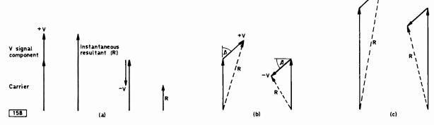
Fig. 10: Imperfect demodulators are not immune to quadrature crosstalk or phase errors in the subcarrier. (a) Correct signal phase. (b) With phase error β the resultant is changed as shown here. (c) Using a larger amplitude reference carrier the effect of the errors shown at (b) is reduced.
