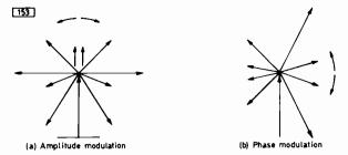
Fig. 5: In practice there are innumerable sideband components for even the simplest signal. A few arbitrarily selected ones are shown here.
