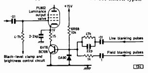
Fig. 1: Flyback blanking in the cathode circuit of the luminance output pentode.
