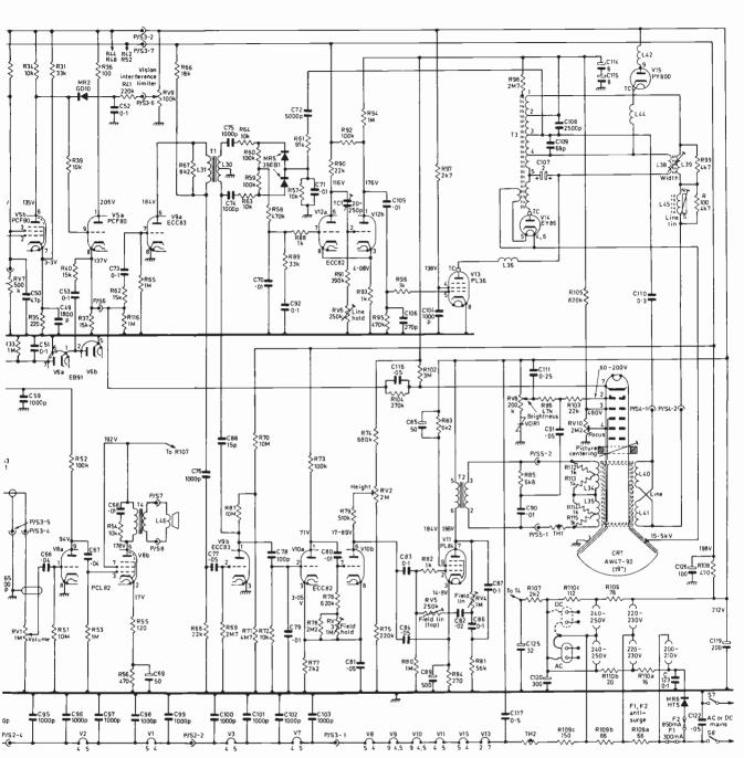
Fig. 3: Circuit diagram, Bush Models TV103, TV105, TV108, T105c and T108c. Model TV109 (21in.) is similar.
