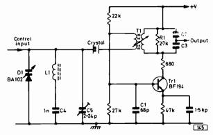
Fig. 4: The reference oscillator circuit used in the Philips G8 single-standard chassis. The crystal is in the feedback circuit.
