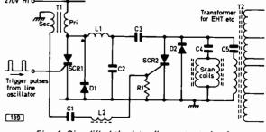
Fig. 4: Simplified thyristor line output circuit.
