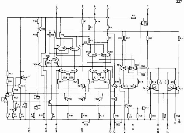
Fig. 4: Internal circuit of the TBA520Q chrominance demodulator, G-Y matrix and V switch i.c.
