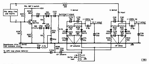
Fig. 2: The chrominance synchronous demodulator and PAL V switch circuits.
