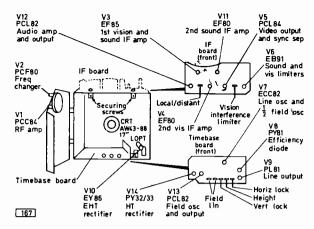
Fig. 5: Chassis layout, 506T series.
