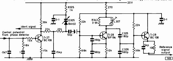
Fig. 5: D.C. amplifier, reference oscillator and buffer amplifier circuits used in GEC dual-standard models.
