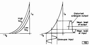
Fig. 2: (a) Beam current/grid voltage curves for a typical c.r.t. (b) The curved la/Vg characteristic of a c.r.t. causes an increased d.c. component of beam current output due to subcarrier rectification.
