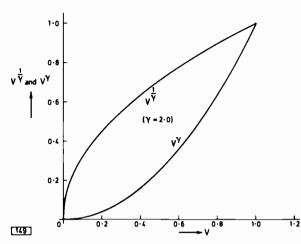
Fig. 1: How the gamma correction applied at the transmitter (top curve) compensates for the characteristics of the c.r.t. (lower curve). For simplicity it has been assumed that gamma is 2: in practice it is normally in the range  $2\cdot7-3$ .
