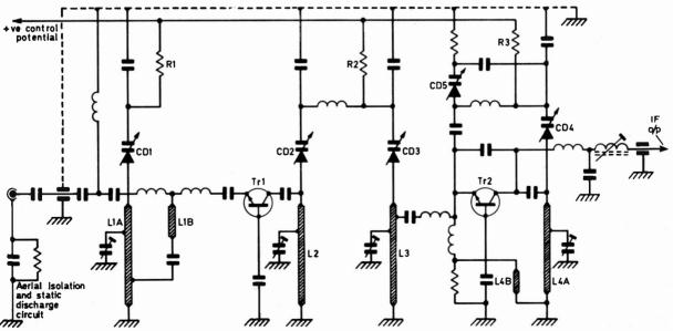
Fig. 3: Skeleton circuit of the Philips capacitance-diode tuner unit.
