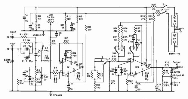
Fig. 1: Circuit diagram of the integrated circuit oscilloscope preamplifier.
