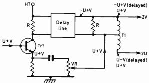
Fig. 2: Commonly used PAL delay line circuit.
