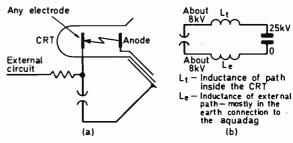
Fig. 7: (a) The basic protection circuit. (b) The equivalent circuit of the flashover path of (a). The e.h.t. voltage is divided between the two inductances.
