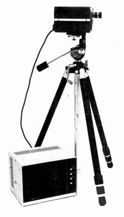
One of Teleton's new inexpensive CCTV systems, comprising a 920 camera, standard lens, 9 in. monitor, tripod and cable.
