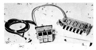
Fig. 2: The capacitance-diode tuner unit used in the Philips G8 single-standard colour chassis.
