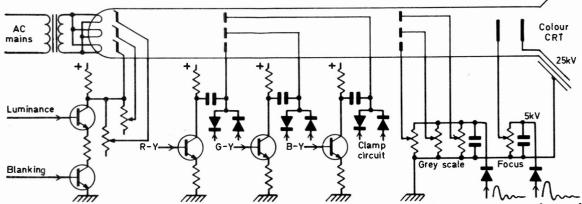
Fig. 3: How much damage would be caused by a flashover to each electrode in turn? Answer, one transformer, four high-voltage power transistors, one low-level transistor, eight diodes (one a 6kV type), six potentiometers and several miscellaneous components!
