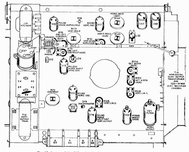
Fig. 10: Layout of the 368 main chassis, shown in the lowered position.
