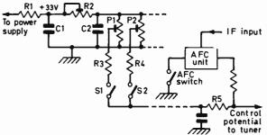
Fig. 4: Basic control arrangement used with the Philips capacitance-diode tuner.
