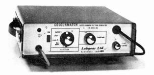
The Labgear CM6010/RG colour pattern generator.
