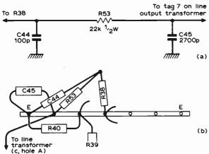
Fig. 1: (a) Line timebase modification. C44 and C45 are 500V ceramic capacitors. (b) Modified tagstrip layout to incorporate the extra components.
