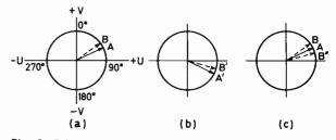
Fig. 3: Principle of phase-error cancellation in the PAL system.
