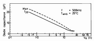
Fig. 1: The capacitance/reverse bias characteristic of a Mullard variable-capacitance diode.
