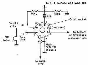
Fig. 1: Socket connections for initial testing.
