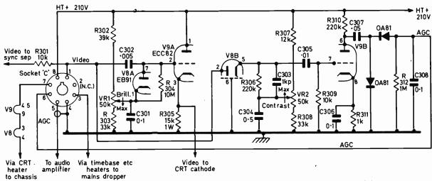
Fig. 3: Circuit of the add-on unit which forms a link between the Murphy unit and the rest of the set.
