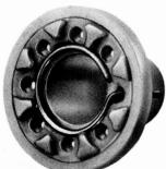
Left: Ringtrap type tube base to provide flashover protection for a monochrome tube. The wire ring forms a sparkgap to each tube pin. (Photograph courtesy of Mullard Ltd.) Unfortunately this technique is not very appropriate for use in colour receivers because the focus electrode needs a larger sparkgap. A further snag is that there are no unused pins, so it is difficult to bring out a connection from the ring for earthing purposes.
