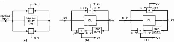
Fig. 1: Principle of operation of the chroma delay-line circuit in a PAL-D receiver,
