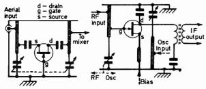
Fig. 5 (left): Basic f.e.t. u.h.f. amplifier circuit Fig. 6 (right): Basic f.e.t. u.h.f. mixer circuit.
