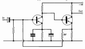
Fig. 11: Feedback pair: the feedback resistor RF determines the gain of the pair and also stabilises the d.c. working bias.
