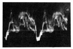
Fig. 3: Two vision signal lines at the detector load.
