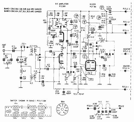
Fig. 3: V.H.F. tuner circuit and interconnections.
