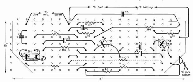
Fig. 4: Veroboard layout. Note that f.e.t.s. are very sensitive to static discharged through the device via the gate electrode and to avoid the possibility of damage to the gate oxide layer due to this cause the leads of the TAA320 are shorted by a clip when supplied. The clip is arranged so that it need not be removed until the i.c. has been mounted on the Veroboard. R7, R10 and C6 are on the conductor side of the board.
