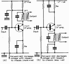
Fig. 3: Application of forward a.g.c. to transistor i.f. amplifier stages.
