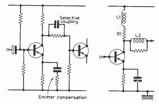
Fig. 9 (left): Use of selective coupling and decoupling. Fig. 10 (right): Use of peaking coils. The inductance of the coils is given by the formulae
