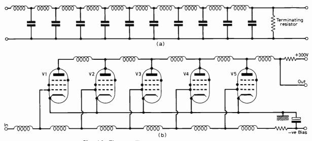
Fig. 14: The travelling-wave or distributed amplifier.
