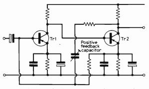
Fig. 13: The use of selective positive feedback with a pair of transistors to boost h.f. gain.
