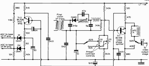
Fig. 4: Transistor a.g.c. system used in many Pye/Ekco models.
