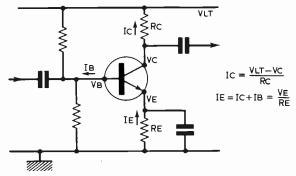
Fig. 29: A simple npn transistor amplifier stage, illustrating the d.c. operating conditions.
