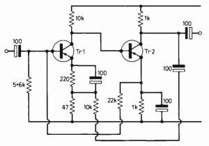
Fig. 12: Video amplifier (30dB gain up to 10MHz) using negative feedback. The 22 k $\Omega$  resistor between Tr2 emitter and Tr1 base is for d.c. stabilisation only. Tr1 and Tr2 can be any r.f. transistor (OC171, AF119 etc.) and the line voltage should be close to the maximum permissible. Bypass each of the 100  $\mu$ F electrolytics with a 1,000 pF mica capacitor.
