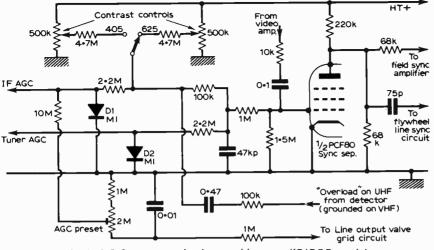
Fig. 1: A.G.C.-contrast circuitry used in many KB/RGD models.
