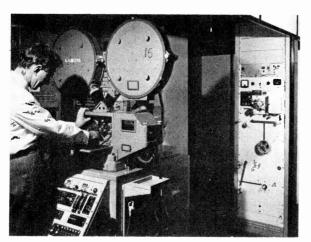
Interior film recording camera with control panel below and two 35mm, magnetic recording machines.
