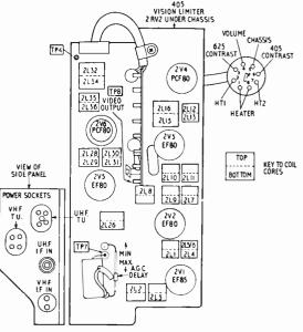
Fig. 4: Above chassis view of the receiver unit.
