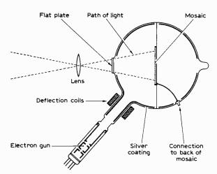
Fig. 3: Construction of the Emitron tube.
