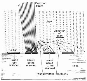
Fig. 5: The action of the Emitron target.
