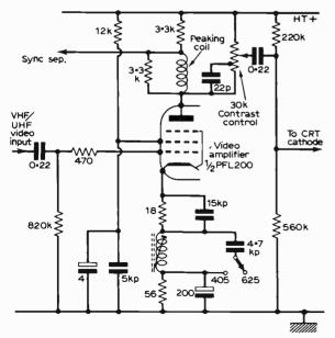
Fig. 2: High-level contrast control system as used in many valve-only and hybrid Pye/Ekco models.
