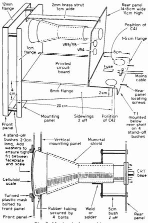
Fig. 6: Mechanical assembly.
