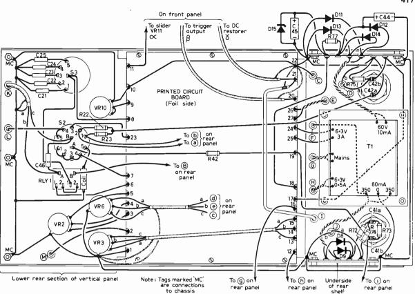
Fig. 5: Underside wiring diagram.
