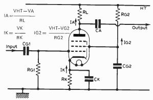
Fig. 27: A simple pentode valve amplifier stage, illustrating d.c. operating conditions.
