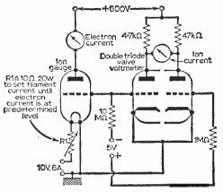
Fig. 2; Method of setting up ion gauge.
