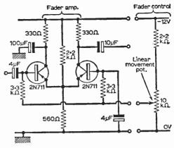
Fig. 53: Circuit of the fader amplifier.
