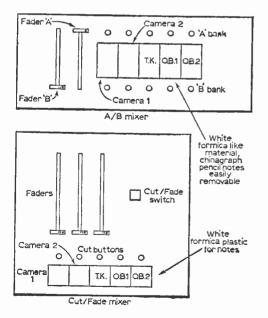
Fig. 58: Layout of mixer control panels.
