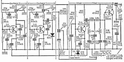
Fig. 2: Complete circuit diagram of the wide range wobbulator.
