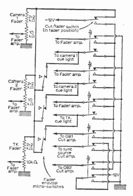
Fig. 57: D.C. control of cut/fade vision mixer
