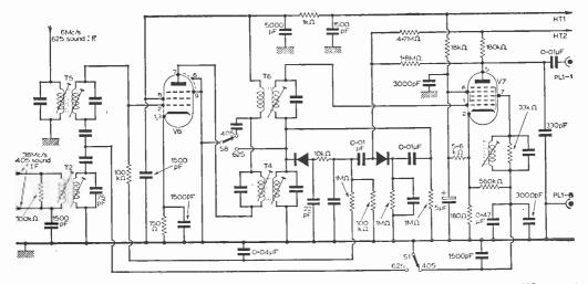
Fig. 2: Typical EH90 dual-standard sound system. On 625 it functions as a 'locked oscillator'' f.m. detector and on 405 as an a.f. amplifier. (G.E.C./Sobell/McMichael series).
