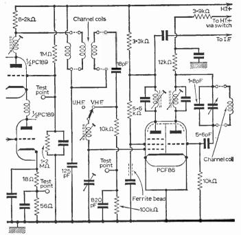
Fig. 46: Simplified circuit of the Philips tuner used in the Cossor CT1964A.
