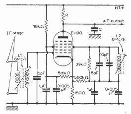
Fig. 1: Basic EH90 'Locked Oscillator' f.m. discriminator. Space charge coupling between G1 and G3 induces a replica of the nput frequency on the latter but lagging by 90°. F.M. variations of the input signal then produce slight variations of this phase disparity to produce an a.f. signal across the anode load resistor.
