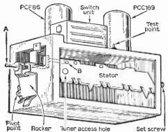
Fig. 47: Philips tuner, the circuit shown in Fig. 46 (above).
