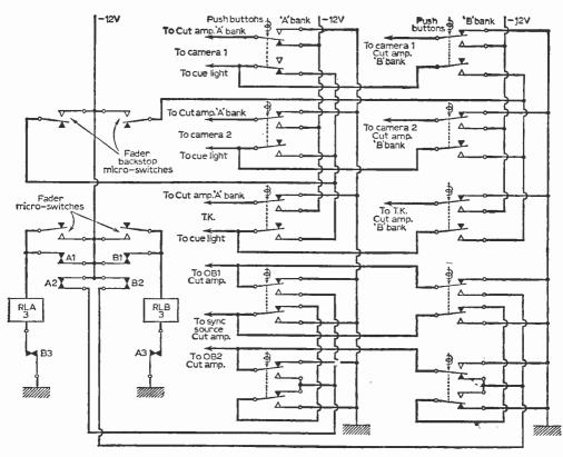
Fig. 55: A/B mixer d.c. switching.
