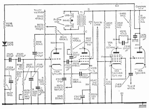
Fig. 6 (above): Field timebase circuitry.
