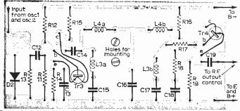
Fig. 3: Etched circuit board for the filter unit. Note: Layout of this unit is fairly critical, the filter operating at new Television frequencies
