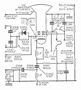
Fig. 4: Cathode-ray tube circuitry.
