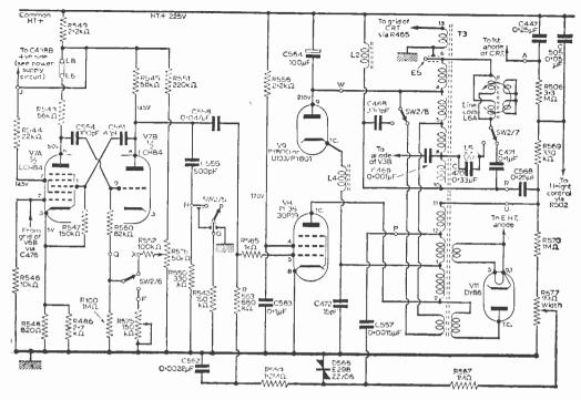
Fig. 5: Circuit of the line timebase
