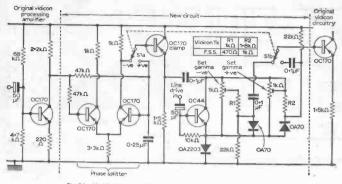
Fig. 34-Modifications to vidicon processing amplifier for use with TK screens.
