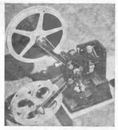
The Specto without covers showing lamp and drive mechanisms.
