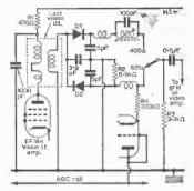
Fig. 2—Dual-standard vision detector employing 2 diodes. (Alba) DI and D2 (DA795) are the 405 and 625 detectors respectively, with R4 3:3 k(1) resistor as common detector load but vitually shunded on 525 by R2 to increase bandwidth to accommodate 6Md5; inter-carrier sound. Diode connected PCL84 triode functions as overload diade on 525. A.C. coupling to video amplifer valve eliminatos need for bias change on system. change-over.
