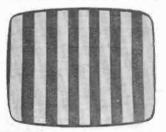
Fig. 7—Vertical bar generator running at an exact multiple of the line frequency. (Useful for checking fine linearity.)
