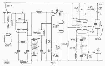
Fig. 21—An example of modern cethode follower video amplifier and output stages is given by the Decce circuit. This has many common features, but also one or two quite individual tricks of design and is worth studying.
