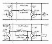
Fig. 33-Modifications to sean chassis to move shift control.
