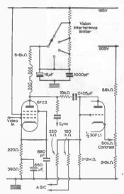
back at middle and low frequencies, while the 1.000pF across the upper leg of the bias network removes the negative feedback at the upper end. This gives a form of "top lift" as negative feedback is progressively applied as the frequency falls.
