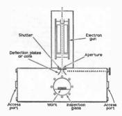
All this can also be done by the laser, but the electron beam has one great advantage over the laser; it can be deflected with great accuracy, and the deflection can be electronically controlled, and, if necessary, programmed by a computer.
