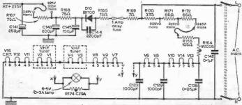
Fig. 6-Power supplies including the heater chain.
