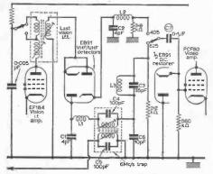
Fig. 3—Dush-standard vision detector circuit (Deces), L12/3 are Li, Hiller chokes with RI and R2 respectively being 405 and 625 detector diode loads. A.C. grid coupling V1a, C7 to video amplifier grid has d.c. restoration by EBSI diode. Unusually, the 6Mc/s Inter-carrier sound i.l. is taken from the detector instead of from the video amplifier video.
