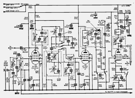
Fig. 3-Circuit of the i.f. unit.
