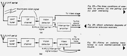
effectively carries the sound modulation at f.m. The vision modulation fails to influence the f.m. detector and, in any case, the a.m. is suppressed by amplitude limiting in the intercarrier channel.
