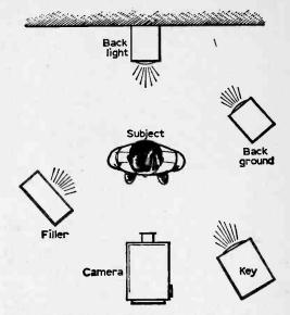
Fig. 29—Layout of studio lamps and cameras.
