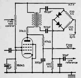
Fig. 17—Sync separator stage of Ekco T344F, using a 6F23 pentode.
