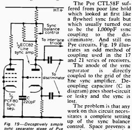
Fig. 19-Deceptively simple sync separator stage of Pye 17 and 21 groups of receivers with direct coupling from sync separator anode to line sync amplifier grid.
