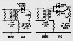
Fig. 2-Switchable diode detector (diodes).
