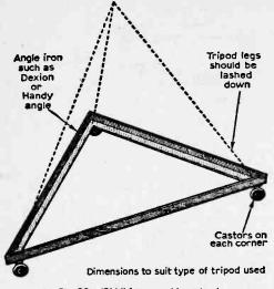
Fig. 28-Skid' for use with a tripod.
