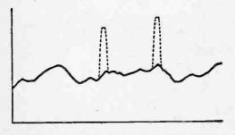
Fig. 3—Typical a.f. waveform with two random noise pulses superimposed.
