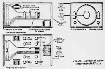
mask in the areas not scanned by the raster. The perspex is edged with plastic trim (obtainable from hardware stores), as used on kitchen tables and similar furniture. Any rough edges of the camera and viewfinder could be trimmed with this provided that it does not restrict access.
