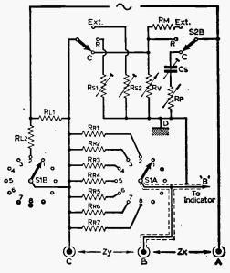
Fig. 3-Circuit of the bridge
