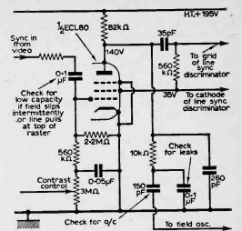
Fig. 18—Unusual regulation method for G2 voltage employed by Decca in the DM35 range.
