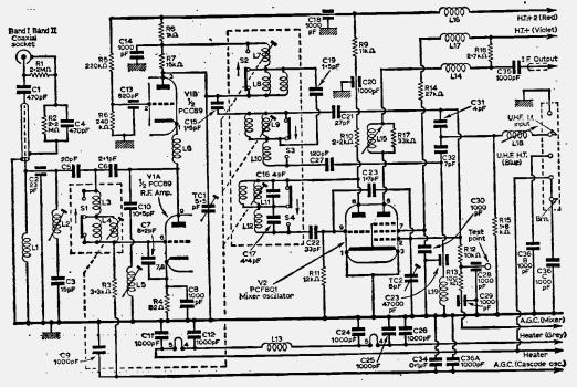
Fig. 1-The dual-standard tuner unit.
