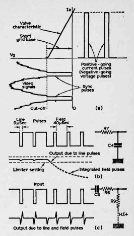
Fig. 14—What happens to the waveforms. (a) the composite signal is applied to a short grid base stage so that sync pulses cause conduction while video information cuts the valve off (positive-going sync negative-going video). (b) longer field pulses are integrated to form one larger pulse and limiter setting renders smaller line pulses ineffective. (c) passing the total sync signal through a differentiating circuit produces short steep pulses at leading and trailing edges.
