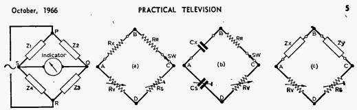
Fig. 1—Basic a.c. bridge circuit.
