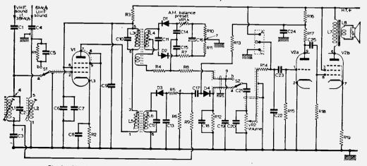
Fig. 1—Circuit diagram of the 405/625 sound system used in the STC VC2 range of receivers.
