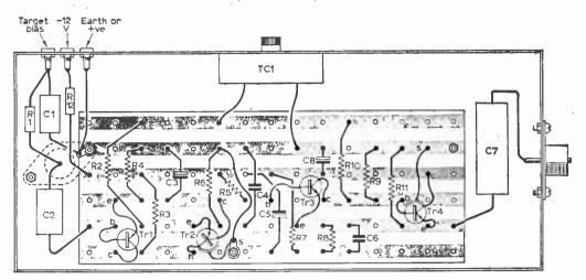
Fig. 17-Veroboard layout of the head amplifier.
