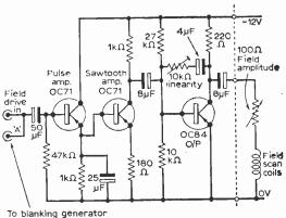
Fig. 15-The field scan circuit.
