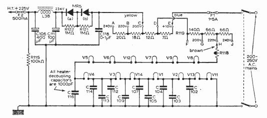
Fig. 2—The power supply and heater chain.
