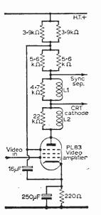
and a node voltage variations which reduce the anode voltage and signal thus the overall amplification. Again bv choosing a decoupling capacitor to offer high reactance to very low frequencies but negligible reactance to other frequencies, the response curve can be straightened.
