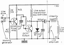
Fig. 14-The line scan circuit.
