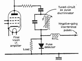
Fig. 26—Showing how the triggering interference pulses for the heptode circuit in Fig. 25 may be obtained from a tuned circuit discriminator and pulse detector, fed from the final vision i.f. amplifier anode circuit.
