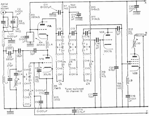
Fig. I—Circuit of the r.f. tuner unit.
