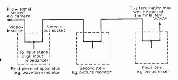
Fig. 10—Showing method of "linking" the coaxial cable between units. Note that cable terminated at one end only.
