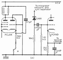
Fig. 4a (above)—Conversion of vision interference limiter triode to diode for frame sync caupling, as in (b), below.
