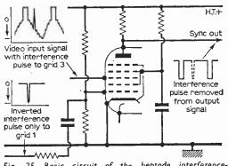
Fig. 25—Basic circuit of the heptode interferencecancelling sync separator.
