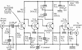
Fig. 16-The head amplifier circuit.
