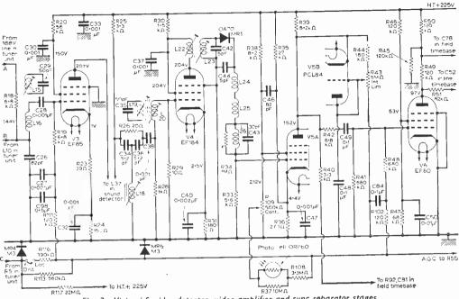
Fig. 3-Vision i.f. video detector, video amplifier and sync separator stages.
