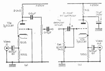
Fig. 9(a) Earthed grid amplifier and 9(b) Cathode follower.
