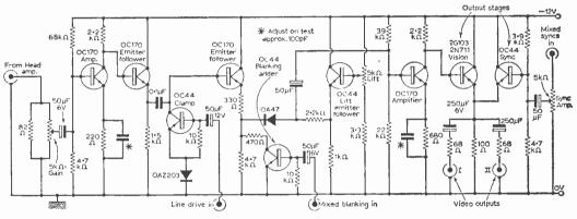
Fig. 18—Circuit of the processing amplifier.
