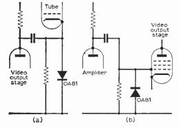
Fig. 11(a)—D.C. restoration at the c.r.t. cathode and 11(b) grid of the video detector.
