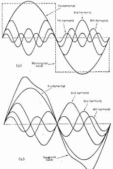
Fig. 21—Showing at (a) how a rectangular wave is produced by the addition of odd harmonics and (b) the formation of a triangular or sawtooth wave by the addition of both odd and even harmonics.
