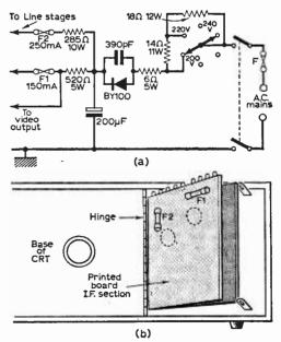
Fig. 5--Separation of h.t. lines can produce confusing symptoms. H.T. supply circuit used in many Philips models is shown (a), with physical position of fuses (b).
