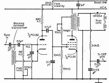
Fig. 6----Typical Pye circuit, as used in Invicta 538. Note anode feed to oscillator triode, use of variable pentode screen voltage to control height, and varistor in scan coil circuit.
