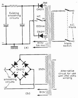
Fig. 12(a)—Power supply for parallel heater and 12(b) alternative cct.
