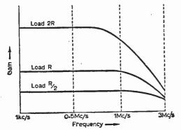
Fig. 1—This graph shows how the overall response of a video stage can be changed by varying the value of the resistive loads.
