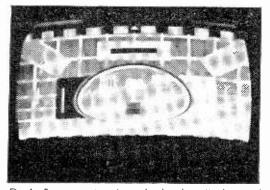
Fig. 4—Bottom compression and reduced amplitude caused by an open-circuit electrolytic capacitor on the cathode of the field output valve.
