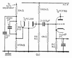
modification. A PCL84 is used as video output and part interference limiter. By disconnecting the limiting feed component and using the triode section as a diode the interlace trouble was immediately overcome. Another shot fired in the valve v semiconductor battle! This change is incorporated in later chassis.
