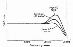
Fig. 2—Additional inductance tuned to resonate with the stray circuit capacitance can be used to peak the h.f. end of the band.
