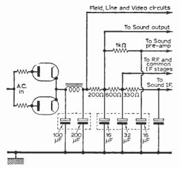
Fig. 7—Another example of division of h.t. supply lines (Decca DM35), which can be complicated by the use of common multiple electrolytic capacitors. Poor earth returns or development of leaks causes circuit interaction.
