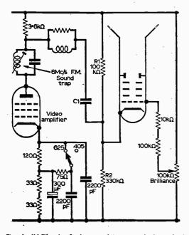
Fig. 4—"AC" tube feed as used in many dual-standard receivers. RI and R2 form a fixed potential divider holding tube cathode at a predetermined voltage thus keeping brilliance level constant despite bias changes on 405/625 changeover.
