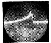
Fig. 11—Damped oscillation on a pulse in the line timebase. This can cause alternate dark and light vertical bars at the left of the bicture.
