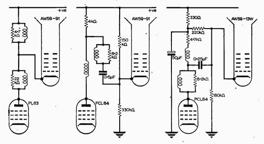
Fig. 6-Typical examples of the three types of resistive/inductive video loads. Left, parallel (Philips 23TG-122A) centre, series (Ferguson 850) right, combined series/parallel (Regentone VCI series).
