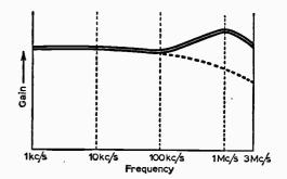
Fig. 5—Typical response curve of video amplifier with series or parallel-connected resistive/inductive load. Dotted trace shows effect of open circuit in, coil if paralleled.
