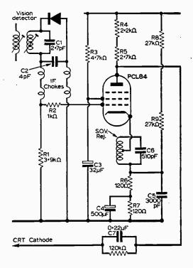
Fig. 3—Video circuit of typical modern 405-line receiver (G.E.C. BT455) embracing details found in practically all other models.
