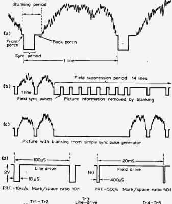
during a black part of the signal. It is sometimes required to stabilise the black level; this is done by a "clamp" which acts during the "back porch" period (Fig. 2a, b).
