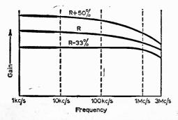
Fig. I—Effect of increased and reduced values of load resistor on typical purely resistive video amplifier.
