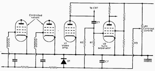
Fig. 1—Typical mean-level auto gain control circuit.
