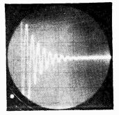
Fig. 10—Damped oscillation suppressed by parallel resistance, as explained in the text.
