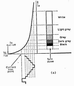
Fig. 2a—Video amplifier waveform operated at the correct biasing point.
