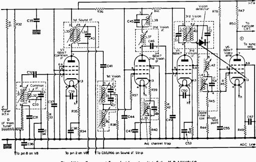
Fig. 1(b)-Common i.f. and video circuits of the K-B NV40/60
