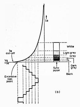
Fig. 2b-Shows effects of excessive biasing (see text).
