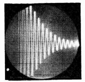
Fig. 9—Oscillogram of unsuppressed damped oscillation.
