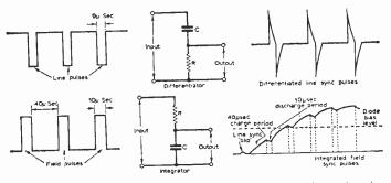
Fig. 5—Line sync pulses after differentiation have a good timebase triggering waveform. Fiela sync pulses after integration (essential for separation) have an inferior slowly rising front produced by the  $40\mu$ Sec charge  $10\mu$ Sec discharge 8 pulse train. The difficulties imposed by this waveform disparity are reflected in the more complex field sync supply systems shown in Fig. 6.
