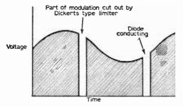
Fig. 2—Showing how part of modulation is cut out when the diode conducts.
