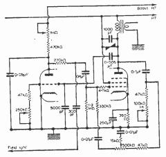
Fig. 1—Typical modern triode-pentode field generator and output circuit (Sobell, McMichael). For rapid fault diagnosis and minimum component checking, identification of the four sub-circuits, sync feed, generator, amplifier and linearity loops is essential.
