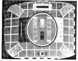
Fig. 11—Compression towards the left-hand edge of a picture can be caused by low mains voltage or by the mains voltage selector being set to a value above that of the mains voltage.
