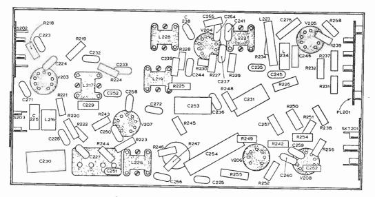
Fig. 6—Underchassis layout of sound receiver.
