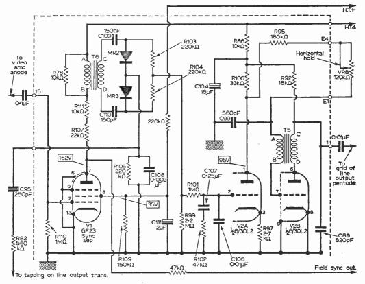
Fig. 4—Complete a.f.c. line oscillator circuit (Ekco-Ferranti) showing sync separator, discriminator, control voltage amplifier (V2A) and blocking oscillator (V2B). Control of V2B frequency is obtained by varying its grid potential by tying it to the anode of V2 instead of the h.t. rail. Sawtooth waveform sample is fed to the junction of the two diodes, with the control voltage taken from the junction of the twin  $220k\Omega$  resistors, a re-arrangement of the system shown in Fig. 1.
