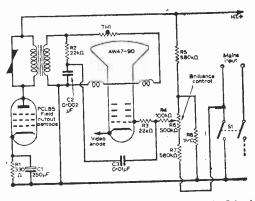
Fig. 4—Typical field flyback suppressor (GEC). On flyback a negative pulse developed across C2 is fed via C3 to the tube grid and blanks out the re-trace. Thermistor THI reduces in value as heat increases the resistance of the scan coil windings thus maintaining height. R7 is returned to the mains side of the mains switch to reduce duration of the "switch-off spot".
