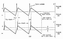
Fig. 2—Discriminator action of Fig. 1. When sync pulses coincide with points of zero voltage on the injected sawtooth waveform as at (a) the net discriminator output is zero, and the line oscillator receives no controlling voltage. If the t.b. alters its frequency so that these points fail to coincide as at (b), a positive or negative controlling voltage is developed to restore the t.b. frequency to its original state.
