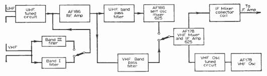
or Band III aerial filter circuit is selected, the output then feeding into the common r.f. amplifier (the presence of the u.h.f. input circuits here has no effect on the v.h.f. performance), then to the v.h.f. bandpass filter (which again is switched for Band I and III) and on to Tr3 which, on v.h.f. acts as a mixer.
