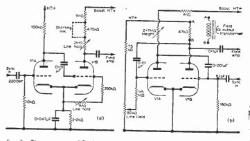
Fig. 2—The two types of field multi-vibrator circuits used in modern receivers, (a) using both capacitive and common cathode resistor coupling. (b) using purely capacitive coupling.
