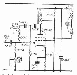
Fig. 3—Unusual field output circuit used in many Decca dual-standard receivers. Scan-coils are directly connected to auto-transformer TI via thermistor, while 40052 decoupling resistor feeds both anode and screen of pentode.
