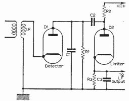
Fig. 4—-Simplified form of Fig. 3, diode valves being shown instead of germanium diodes.
