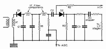
Fig. 3-Circuit containing a series limiter using germanium diodes.
