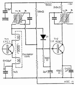
Fig. 3—Overload diode circuit as used in many Alba receivers. Normally TRI collector voltage exceeds TRI collector voltage so that DI fails to conduct. However if a large positive-going a.g.c. voltage reduces Tr2 collector current sufficiently, Tr2 collector voltage will rise above that of Tr1 the diode will conduct and shunt the primary of T1 with its low forward resistance plus that of the 68-52 series resistor. In this way, overloading on very strong signals is prevented.
