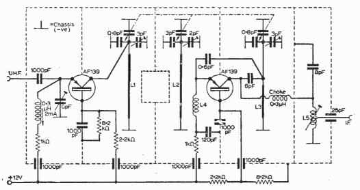
Fig. 2-Circuit diagram of a transistor u.h.f. tuner using quarter-wavelength lecher wires.
