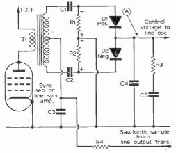
Fig. 1—Basic duo-diode discriminator circuit. TI feeds equal but opposite polarity sync pulses to diodes DI and D2, which develop identical value outputs across RI and R2 but which results in a net zero output at (A).
