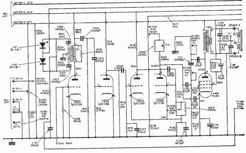
Fig. 5-Sync separator and field timebase circuits.
