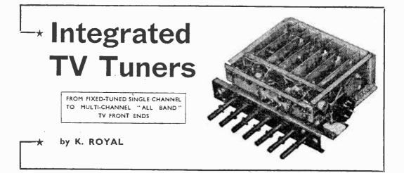
DURING recent times there have been many developments associated with the front ends of television receivers. In very early sets the front end consisted first of an r.f. amplifier and frequency changer built into the main chassis and fixed-tuned to one local Band I channel. Then a modification arose whereby the front end could be pretuned to any one channel in Band I.
