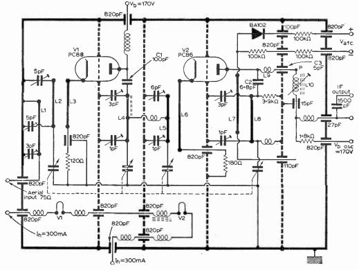
Fig. I—Circuit diagram of Mullard u.h.f. tuner, using valves and half-wavelength lecher wires.
