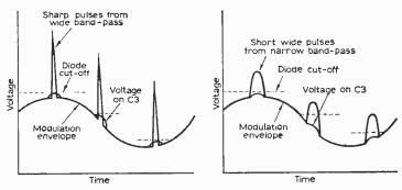
Fig. 1-Effect of wide or narrow bandwidth on interference pulses.
