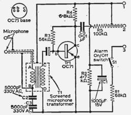
Fig. 2—Circuit of the baby alarm amplifier. The OC71 transistor is powered from the h.t. line of the receiver via potential-divider R1 and R2. Extra smoothing is given by C1. For double safety, two isolating capacitors C2 and C3 are used in the microphone circuit. These must be no larger than 5,000bF and rated at 330V a.c.
