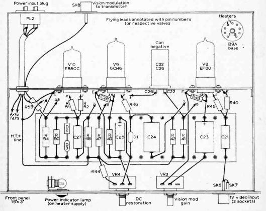
Fig. 10-Component layout diagram of the vision modulator chassis.
