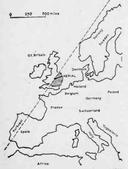
Fig. 1—Showing how a swing through 180° enables the aerial to line up on transmitters all over the continent. transmissions, and this leaves the aerial as perhaps the weakest link in the chain of reception.
