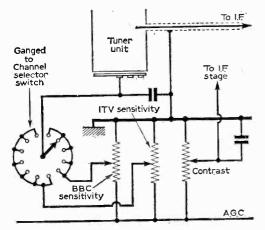
Fig. 4-Contrast and sensitivity arrangement.
