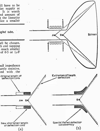
shortened (Fig. 10a) or the deflection coils can be flared to take them further up the neck of the cathode ray tube (Fig. 10b).
