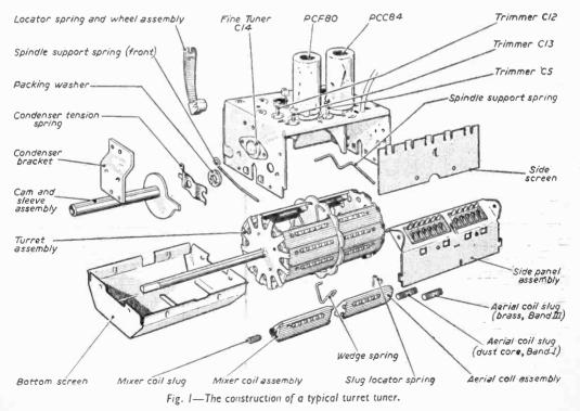
If the springs have been distorted, and can be gently eased back to something near their original shape with a pair of fine pliers, they may be reset by gently pushing inward from the access slots at the outside of the side panel assembly while the turret is switched to a blank position. The turret is then rotated so that the studs "wipe" the springs in a direction from the rivet towards the
