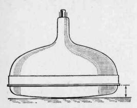
Fig. 2—The arrowed line indicates the critical measurement for tubes held to the cabinet front.
