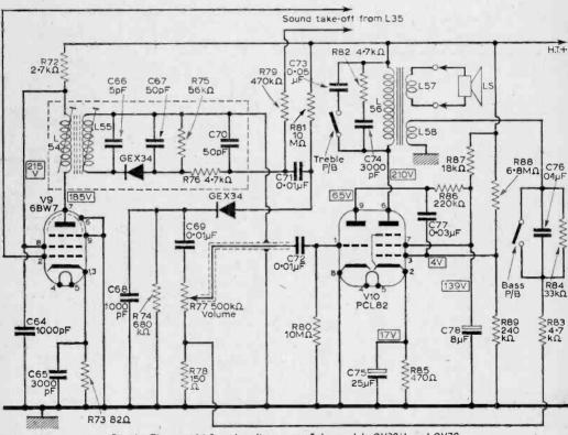
Fig. 4-The sound i.f. and audio stages of the models QV30/1 and QV70.
