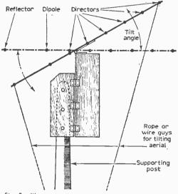
Fig. 2-Illustrating how the aerial tilts up and down on its axis.
