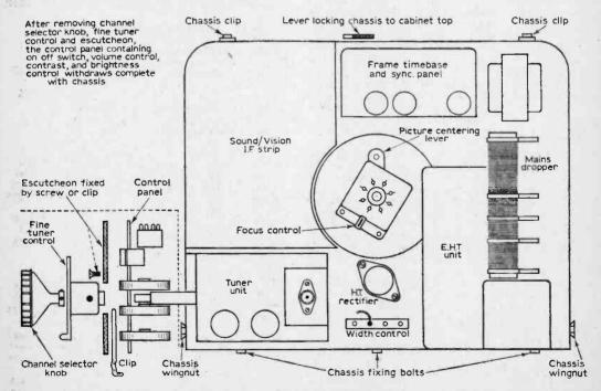
Fig. 1-The basic chassis arrangement of the models covered by this month's article
