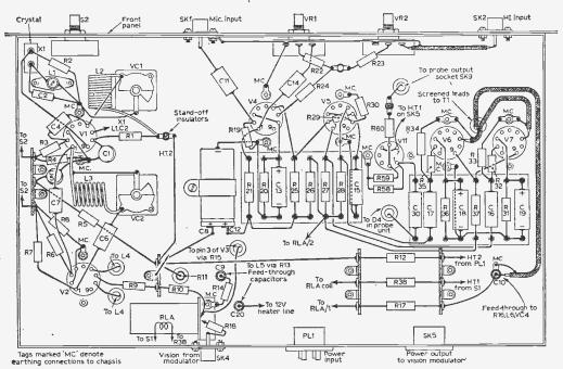
Fig. 9—Underside view of the r.f. and sound modulator unit showing components and major wiring. Note that wiring relating to the following circuits is not shown, or only in part; valve heaters; relay; switches S1 and S2; power supplies; PLI; SK5.
