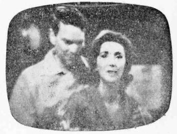
Fig. 5 .- The result of excessive picture "noise."
