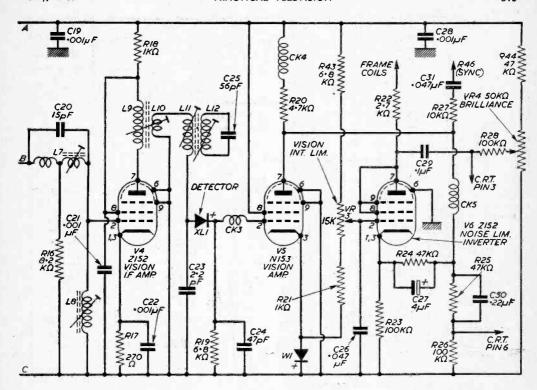
in a lack of voltage at the screen or anode and of course in the case of R13 the sound will also be almost entirely absent. These resistors often burn out as a result of a shorted  $0.001\mu\text{F}$  decoupling capacitor or an internal short in a Z152 valve. Thus when a short is recorded at pin 8, before disconnecting the  $0.001\mu\text{F}$ , always remove the Z152 to see if this is responsible after all.
