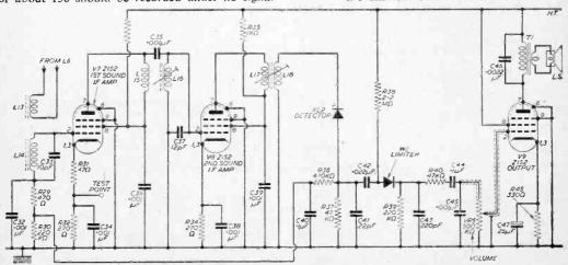
Fig. 6.—Circuit of the sound strip.
