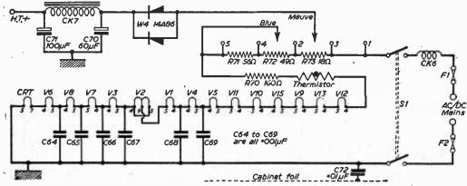
Fig. 8.-Power supply and heater chain.
