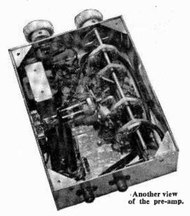
The condenser C2 which is part of the neutralising network for V1 is best set for optimum results on the Band III channel and is simply adjusted until the best picture quality is obtained—for lowest noise. The turns of the inductance L5 may be opened out or closed up when switched to Band III. If it is desired to avoid the losses which may be associated with change of cable at the input socket this socket may be omitted and the aerial downlead wired directly to S1A.
