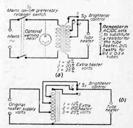
Fig. 1 (a).—A transformer tube booster and (b) an auto-transformer booster. (In A.C./D.C. sets, instead of substituting a resistor for the tube heater, as at (a), the voltage selector may be moved to the next highest position and the tube heater leads shorted together.)
