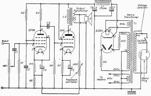
Fig. 1.—Circuit diagram (omitting tone controls).
