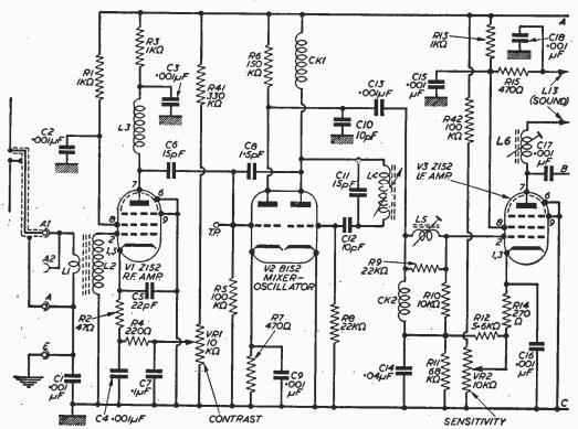
Fig. 7 (a) and, opposite, (b)—Circuit of the vision strip.
