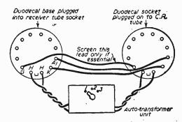
Fig. 3.—Typical arrangement of booster unit.
