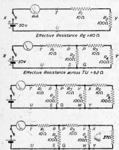
Figs. 3, 4, 5 and 6.—Circuits showing the effect of various resistances, and the voltage and current distribution round the network.
