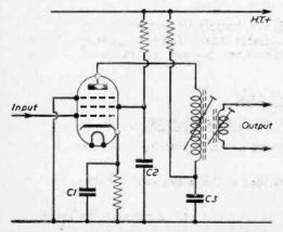
Fig. 3.—Decoupling capacitors, such as C1, C2 and C3, can be checked by shunting each in turn with a similar type of component while observing the instability symptom.
