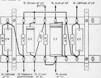
Fig. 3.— Wiring of the group board upon which the smaller parts are mounted.
