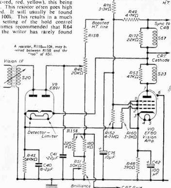
Fig. 3.-Video detector and amplifier stages.
