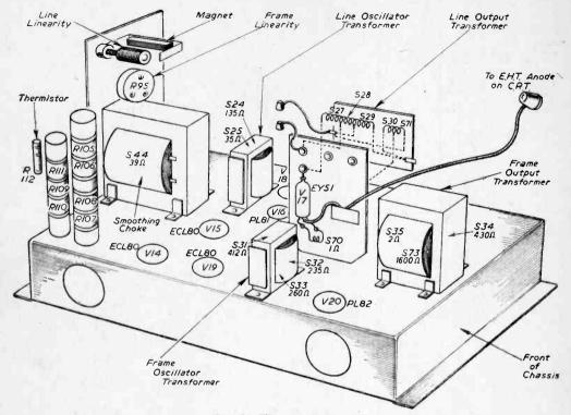
Fig. 6.—The chassis layout.
