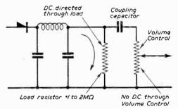
Fig. 3(b).—Fitting an isolating capacitor before the volume control.
