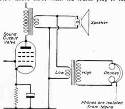
Fig. 2.—Headphones should be wired using an isolating transformer.
