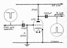
Fig. 2.—A typical line sync inverter circuit using a triode valve.
