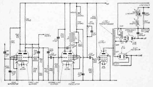
Fig. 1.—Sync separator and line timebase circuits.
