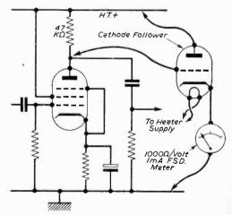
Fig. 2.—Using the cathode follower voltmeter for reading an anode voltage.
