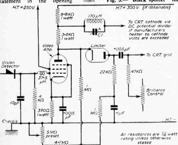
Fig. 6.—Circuit which can be added to any existing receiver.
