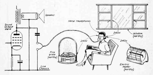
Fig. 1.—The dangers of connecting headphones direct to a live chassis.
