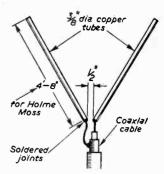
Fig. 1.—The construction.
