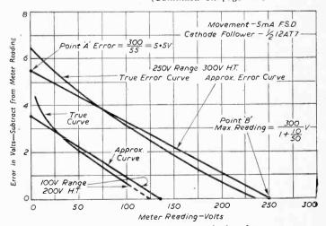
Fig. 5.—Comparison of approximate method and true error.
