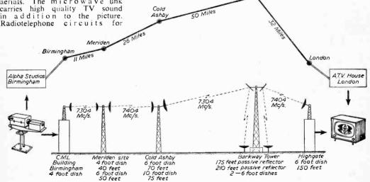
Fig. 1.—A diagram of the route taken by the new TV link.
