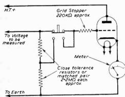
Fig. 4.—A suitable circuit for the cathode follower voltmeter.
