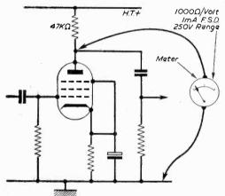
Fig. 1—Using a conventional meter to read an anode voltage; errors may be introduced if the meter takes a large current.
