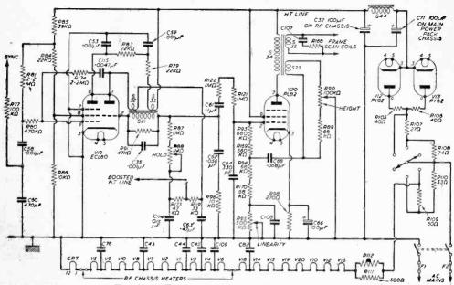
Fig. 2.—H.T. supply and frame timebase circuits.
