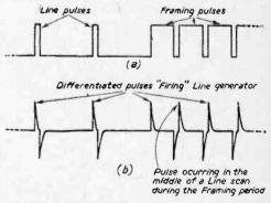
Fig. 4.—The differentiated pulses employed to hold the line generator in synchronisation during the framing period.
