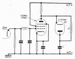
Fig. 1.—Simple automatic type of vision limiter.
