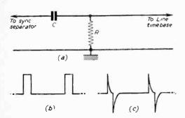
Fig. 1.—A basic differentiator circuit is shown at (a) and line sync pulses af (b), while (c) shows how the pulses are shaped due to the action of (a).
