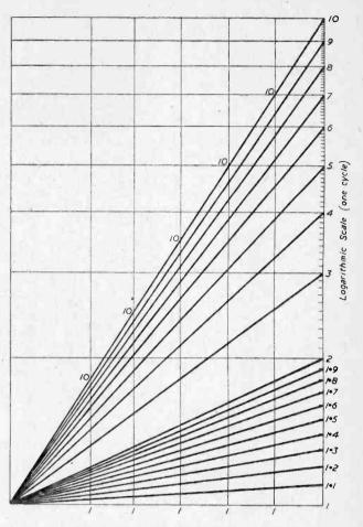
Fig. 1.—Drawing the modulus chart.
