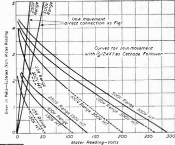
Fig. 3.—Error curves corresponding to the connections in Figs. 1 and 2.
