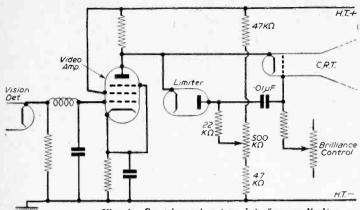
Fig. 4.—Spot inversion type interference limiter.
