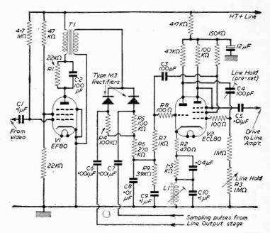
Fig. 5.—The "auto-sync" and associated circuits of a commercial television receiver.
